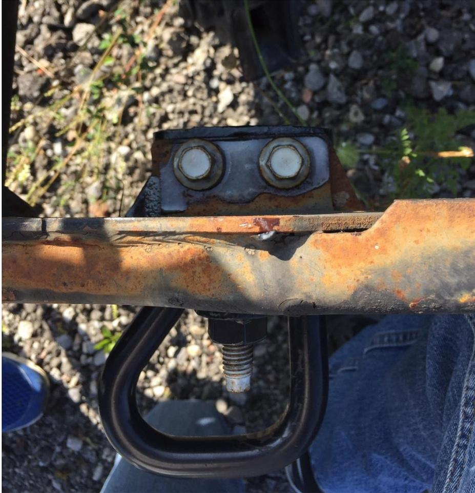
Note how the bolt coming out the front of the cross member bolts in from the engine bay side.
