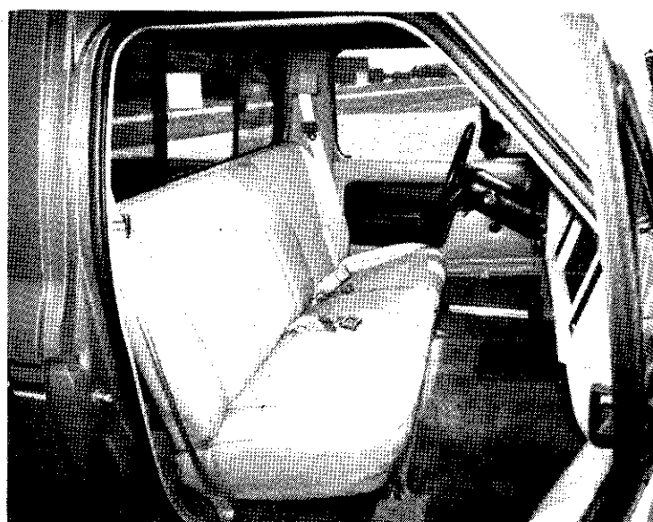
Standard bench seat has 5½-inches of travel and features 4-inch foam on Flex-O-Lator suspension w/helical springs.
