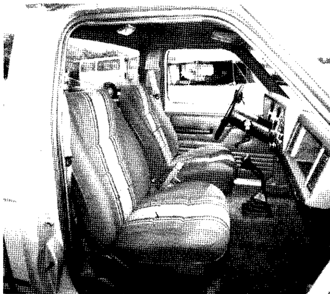
Contoured reclining bucket seats w/lumbar supports in a cloth and vinyl combination have 5½-inches of travel, are optional.
