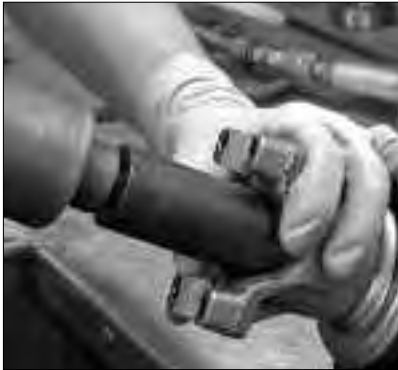
1/2" impact gun on pinion nut
