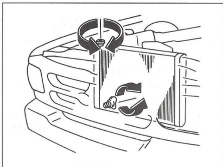
5. Drain the system completely and retighten the plug. Add as much ethylene-glycol-based coolant and water as necessary to provide freezing and corrosion protection.
