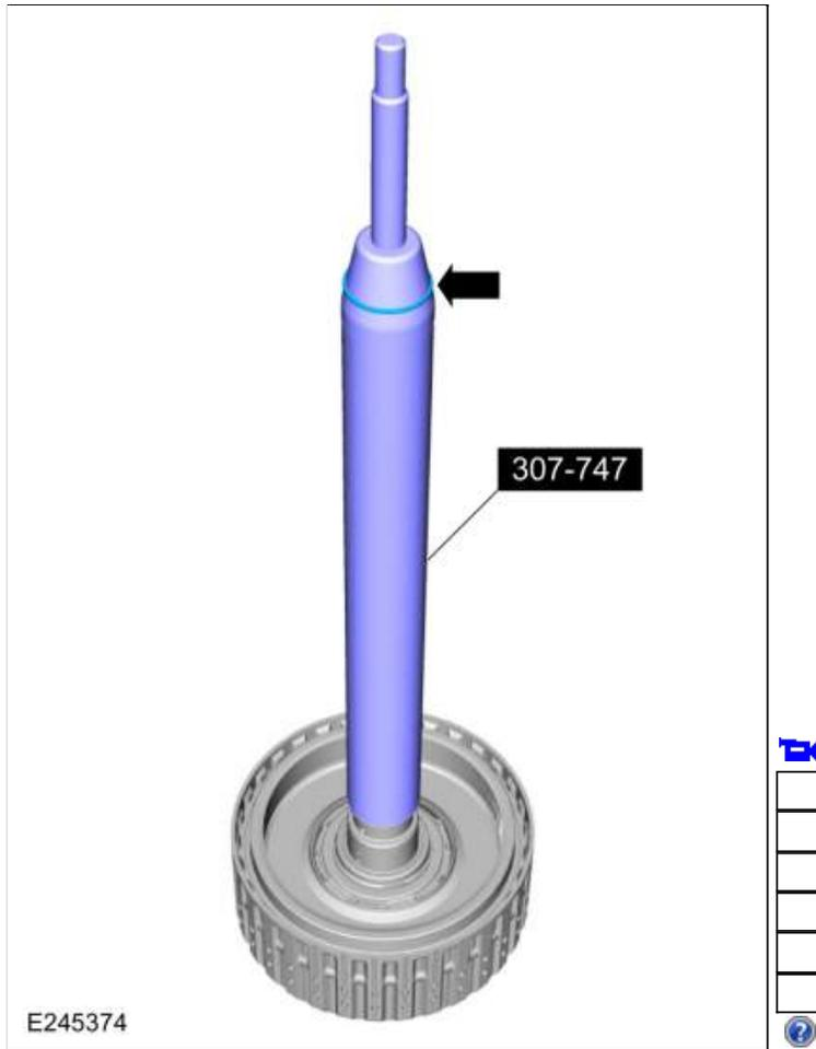
196. Using the top half of the special tool, slide the Teflon® seal into the groove. Remove the special tools and repeat the steps for the other 4 Teflon® seals.
