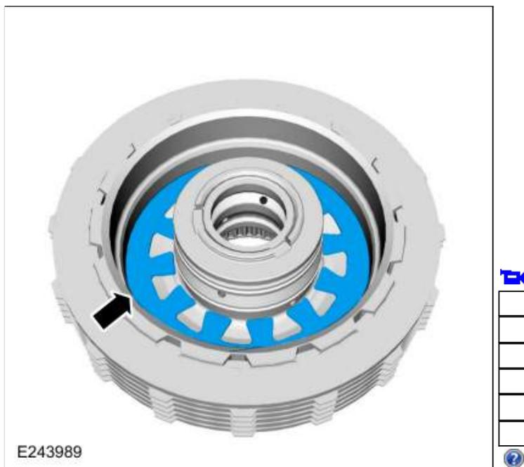
174. Remove the E clutch assembly. Inspect the clutch plates for excessive wear or damage. If the clutch plates are excessively worn or damaged replace as necessary. If the clutch plates are not excessively worn or damaged, they can be reused.
