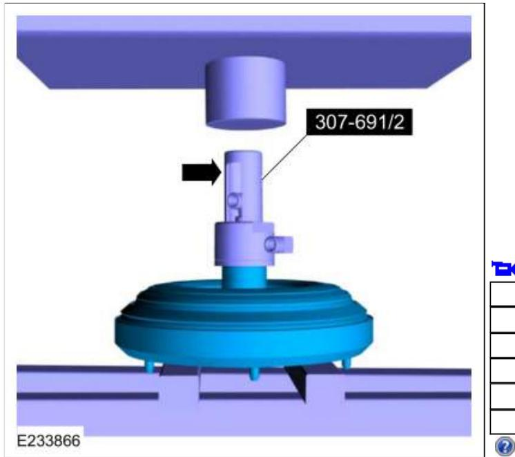
14. Apply enough force from the press to seal the torque converter flush main hub to the torque converter hub.
