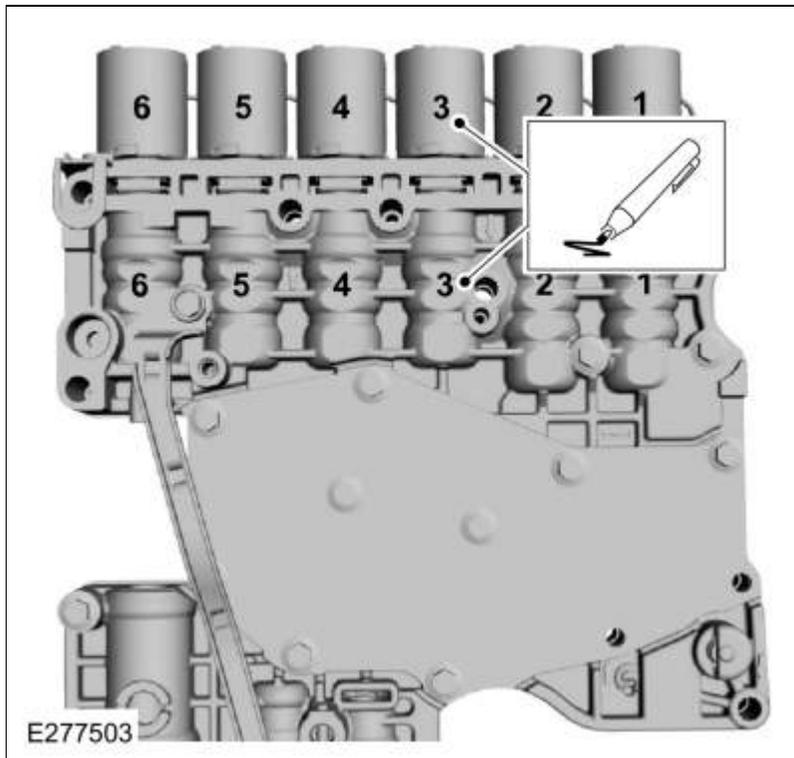
13. Remove the shift solenoid retainer(s).
