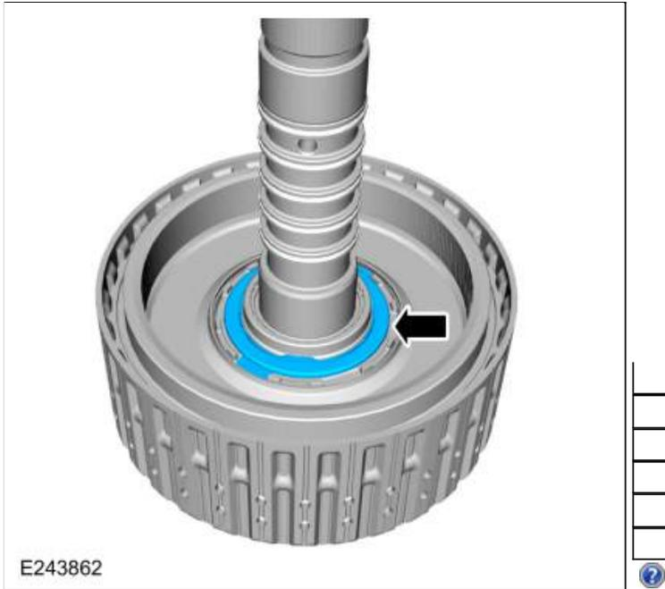
158. Remove the snap ring and the No. 3 ring gear.
