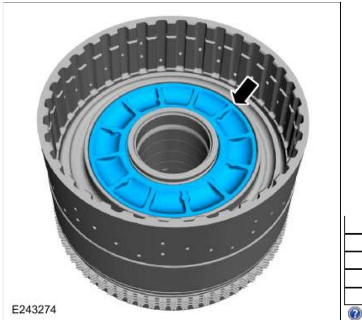
152. Using the special tools and a press, compress the C clutch balance dam and install the retainer.
