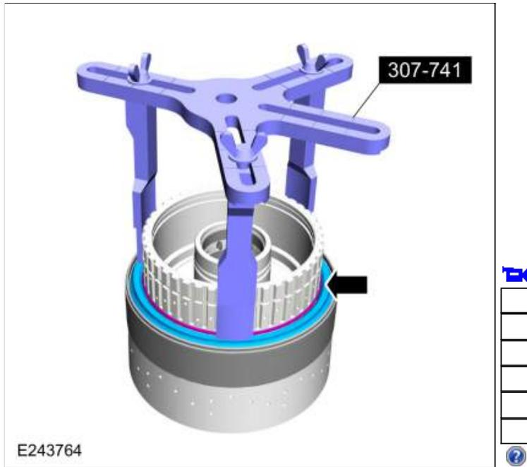
119. Remove and discard the F clutch balance dam outer seal.
