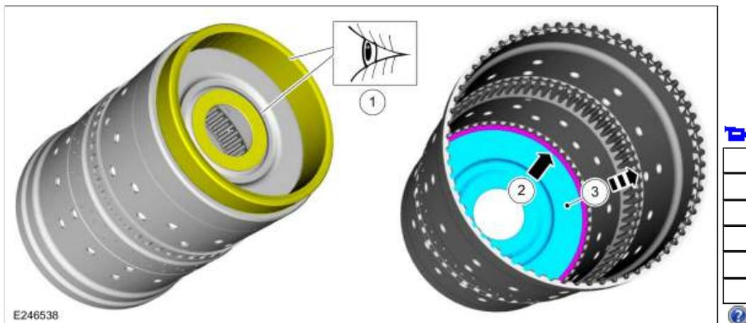
69. Remove the (T8) thrust bearing.
