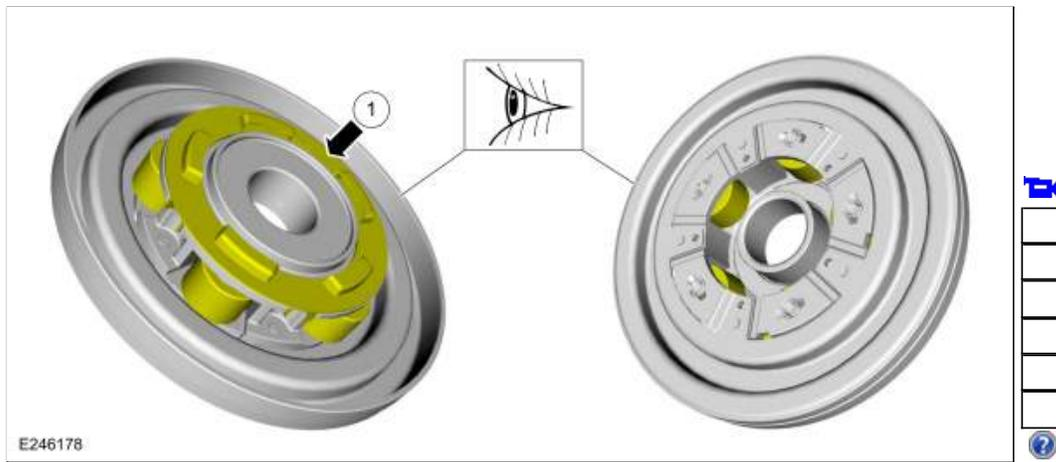
79. If necessary, install the new the fluid collector.
