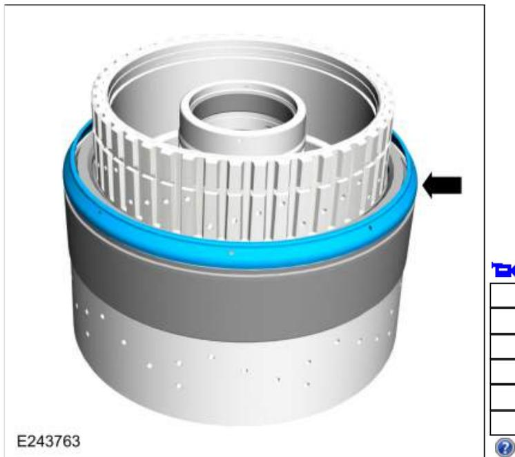
118. Using the special tools and a press, compress the F clutch balance dam and remove the retainer. Remove the F clutch balance dam.
