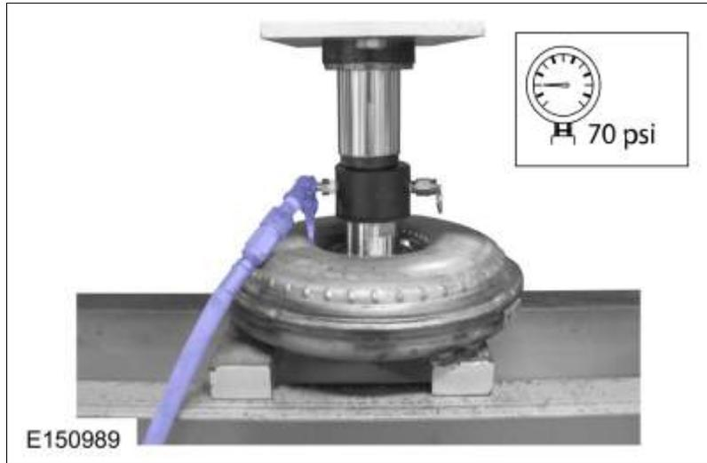
20. Inspect for leaks at the torque converter hub weld and seams with air pressure applied to the valve. A soap bubble solution can be applied around those areas to aid in the diagnosis. If any leaks are present, install a new torque converter.
