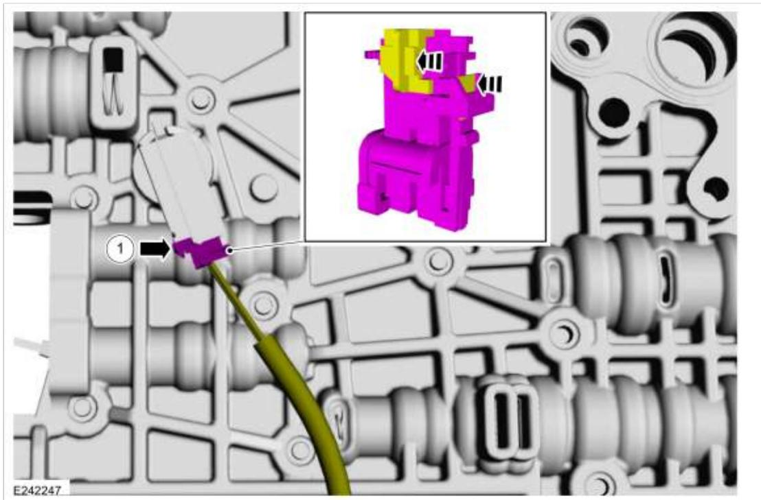
3. Remove the TFT sensor.
