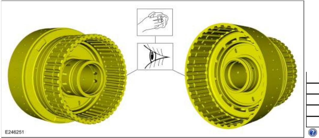
125. Install the new F clutch piston seals. Lubricate the seals with petroleum jelly.
