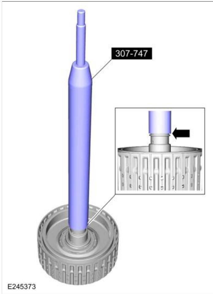
195. Install a new Teflon® seal on the special tool.
