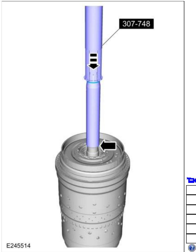
217. Install the special tool to size the 5 Teflon® seals. Allow the special tool to stay on the input shaft for 5 minutes prior to final assembly.
