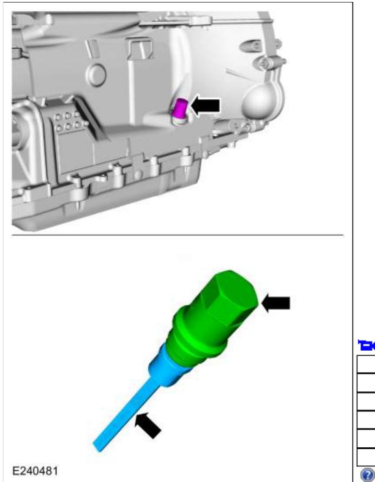
2. **NOTE:** Add 4.8L (5 qt) of transmission fluid to the transmission as an initial fill if:
