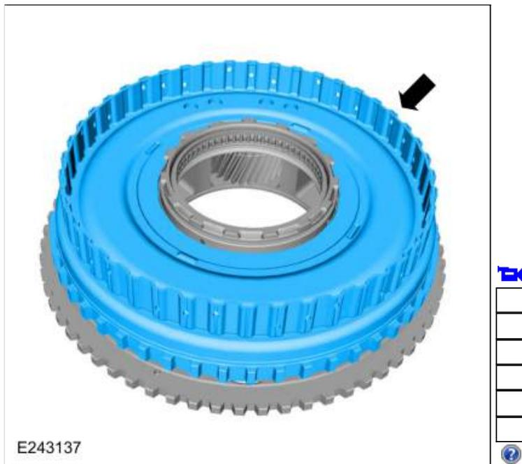
93. Install the No. 1 ring gear bearing.
