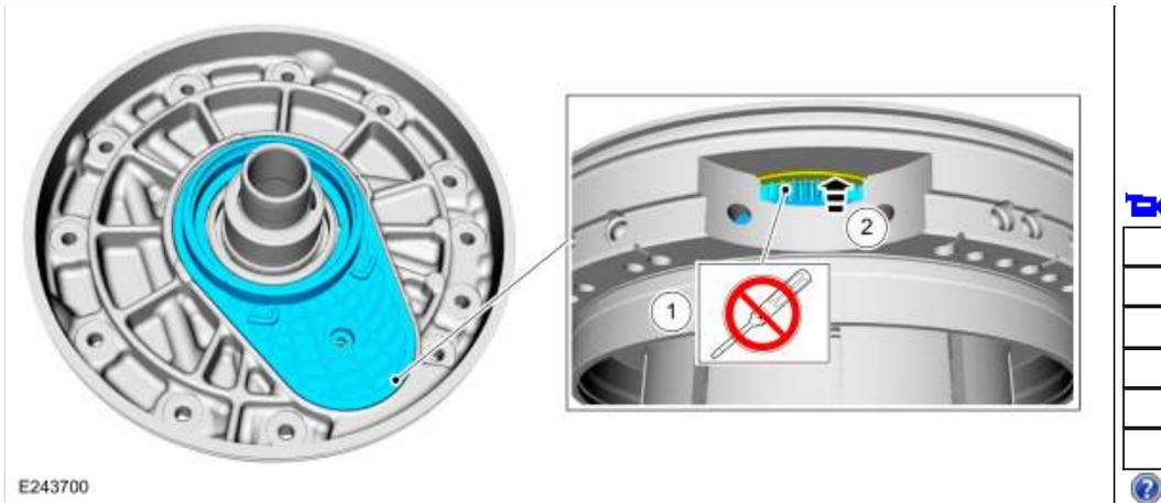
250. Remove the transmission fluid pump drive gear.
