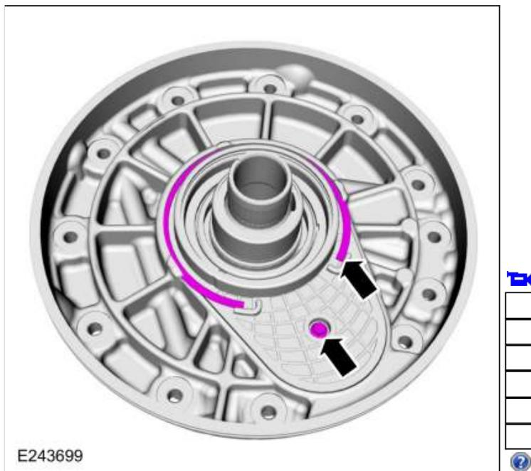
262. Install the new torque converter hub seal on the special tools.
