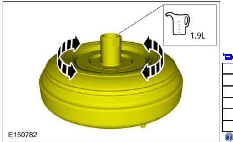
26. Thoroughly drain the transmission fluid.
