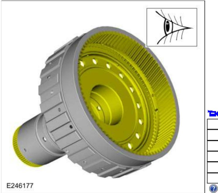
76. Remove the (T5) thrust bearing.
