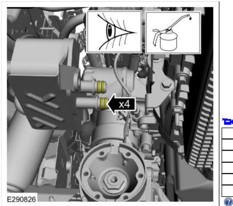
24. Install the transmission fluid cooler and the bolts.
