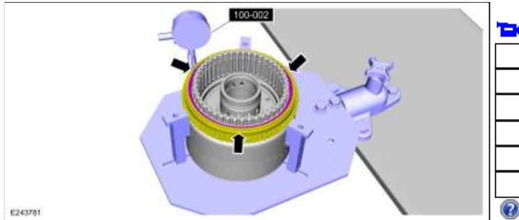
137. Install the new D clutch piston inner and outer seals. Lubricate the seals with petroleum jelly.
