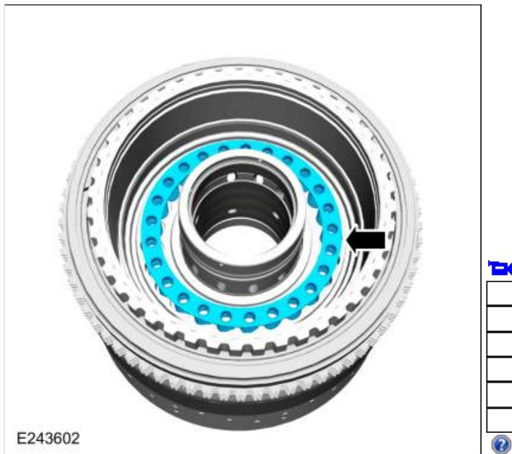
140. Lubricate the new D clutch balance dam seals with petroleum jelly.
