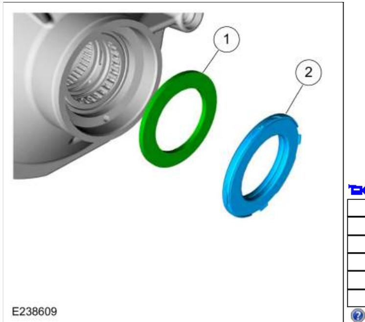
62. Clean and inspect the transmission case and bearings. Check for leaks from plugs and park pawl actuator rod sleeve. Repair or replace as necessary. Refer to: [Transmission Case](#) (307-01 Automatic Transmission - 10-Speed Automatic Transmission - 10R80, Disassembly).
