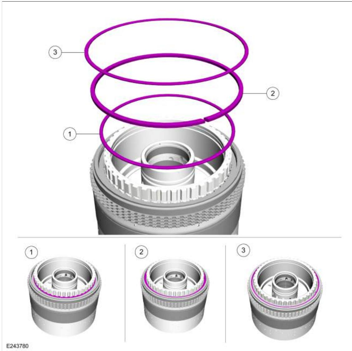
135. Assemble the special tools and position the CDF clutch cylinder with the F clutch facing up.
