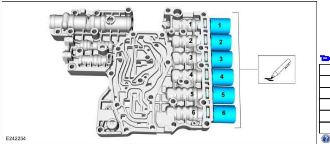
16. **NOTE:** Note the location of the clutch control valves and solenoids for assembly.
