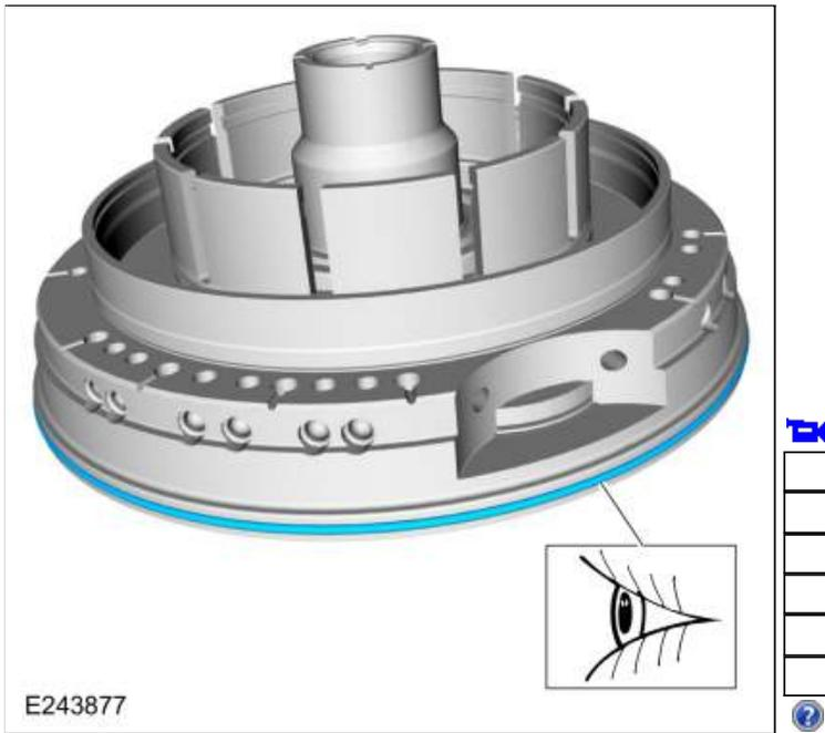
266. Install the new A clutch piston outer seal and the new A clutch piston inner seal. Lubricate the A clutch piston seals with petroleum jelly.
