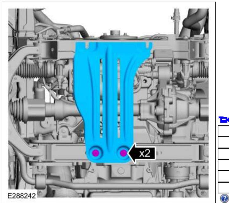
39. Install the skid plate and the bolts.
