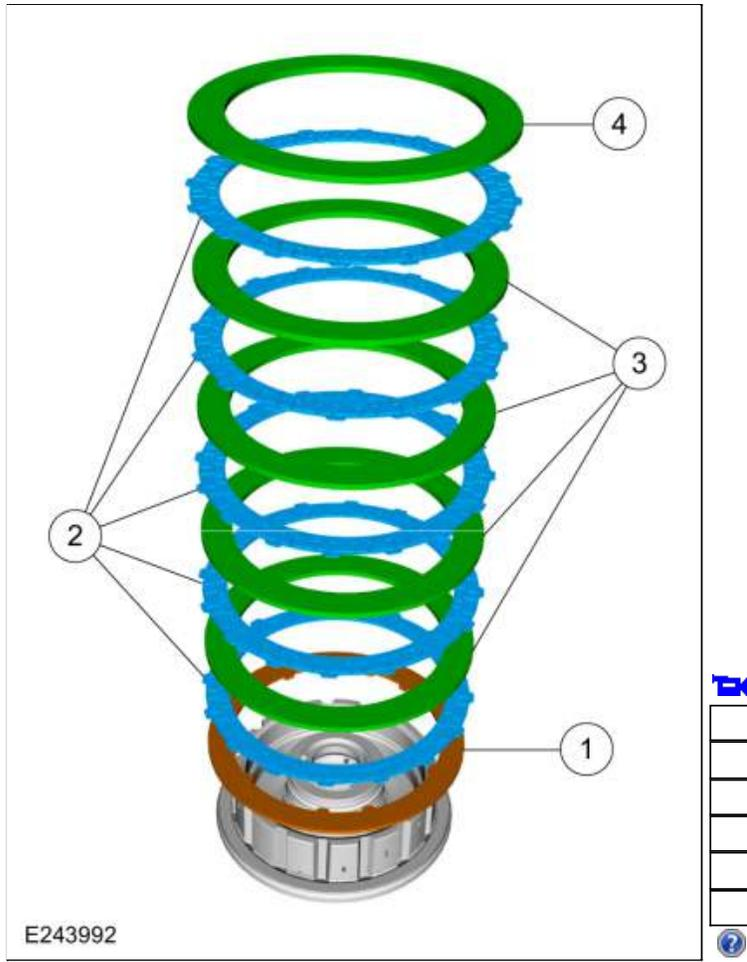
179. Install the E clutch piston return spring.
