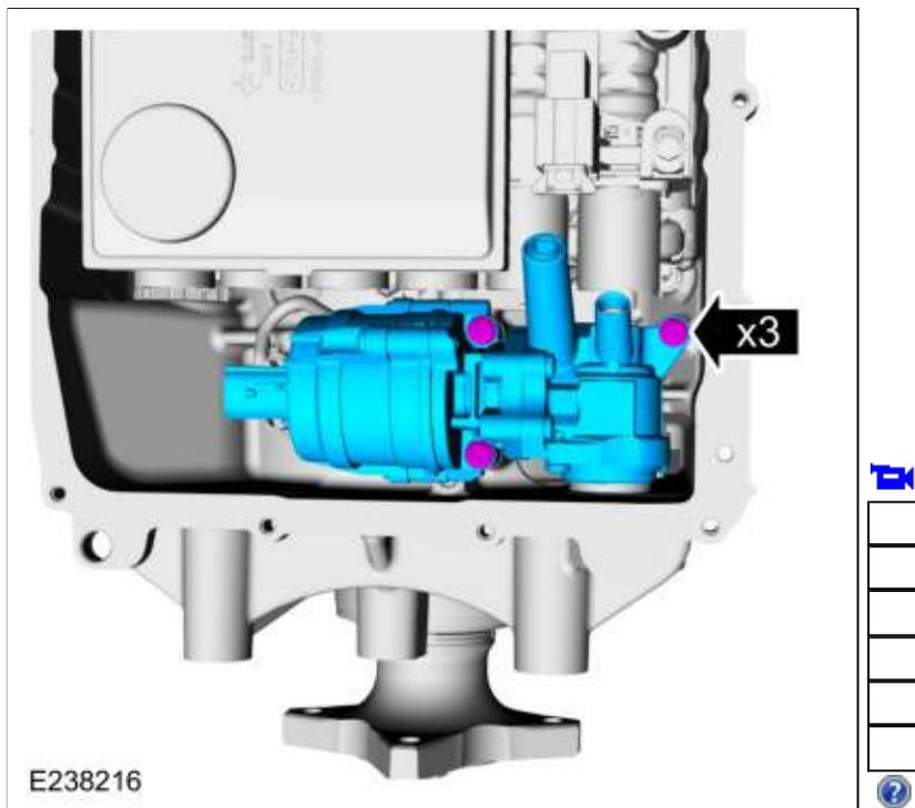
2. Install the transmission fluid auxiliary pump tube seal.
