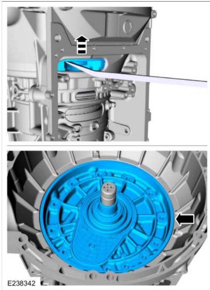
56. Using the special tools and a floor crane, remove the clutch and planetary assembly.
