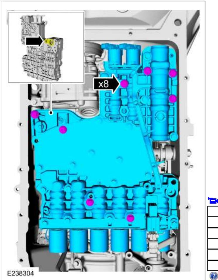
37. Clean and inspect the main control for damage.
