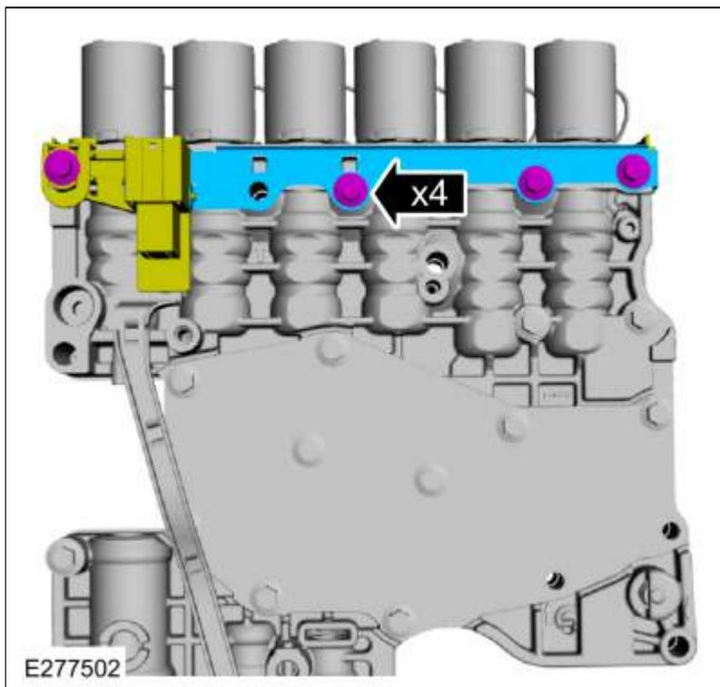
6. Install the main control valve body.
