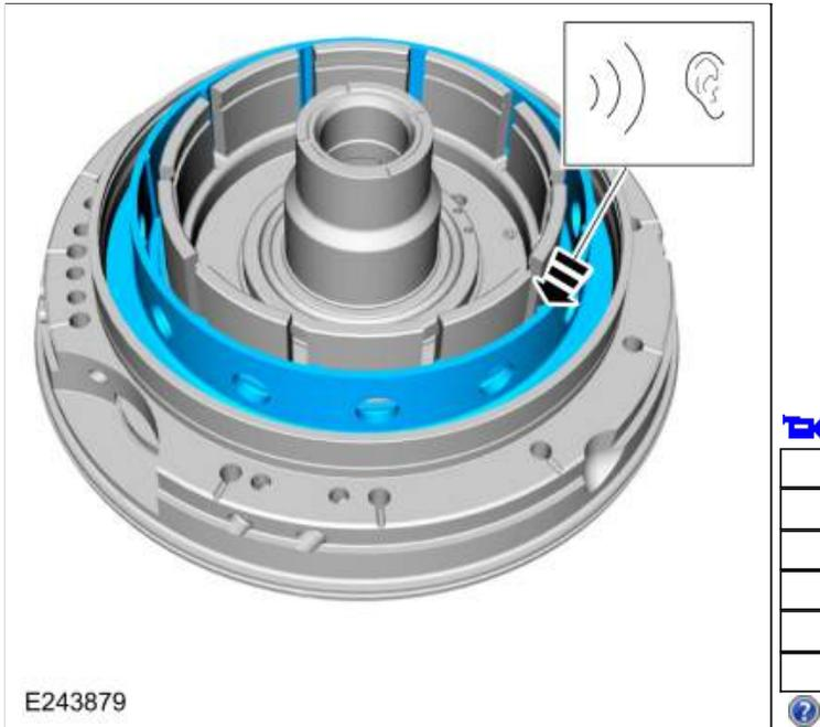
268. Install the A clutch piston return spring with the retaining tabs facing upward.
