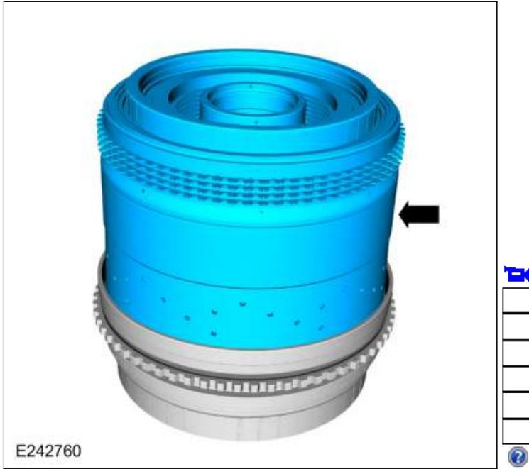
74. Remove the No. 3 sun gear shaft and No. 2 ring gear assembly.
