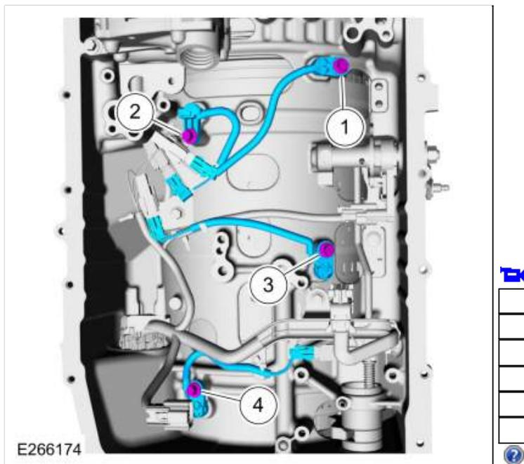
305. Connect and lock the speed sensors.
