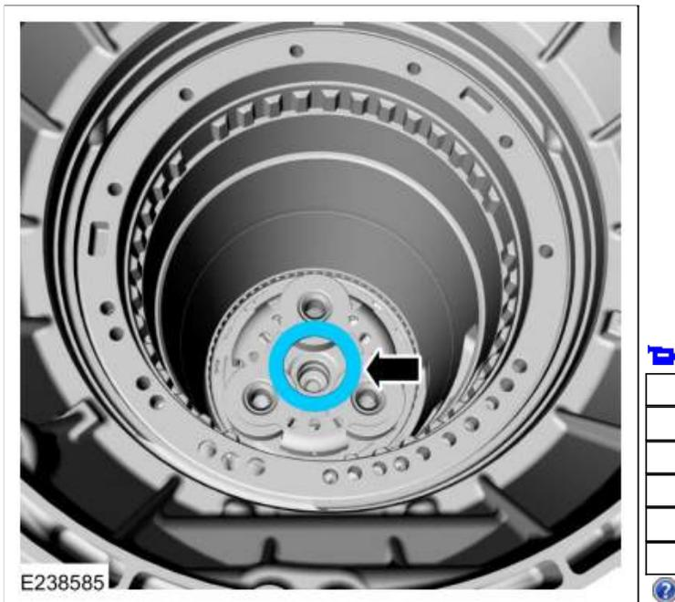
233. Lubricate the output shaft bushing with petroleum jelly.
