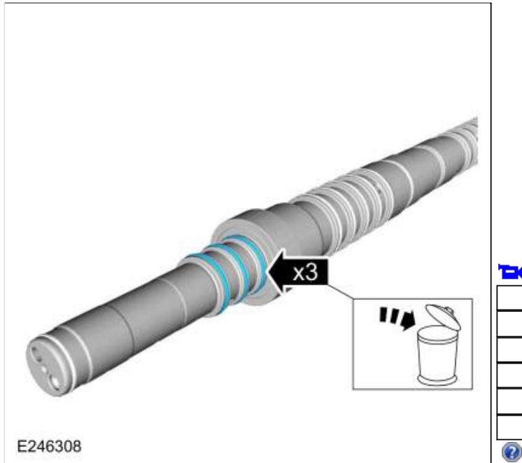
167. Remove and discard the input shaft Teflon® seal.
