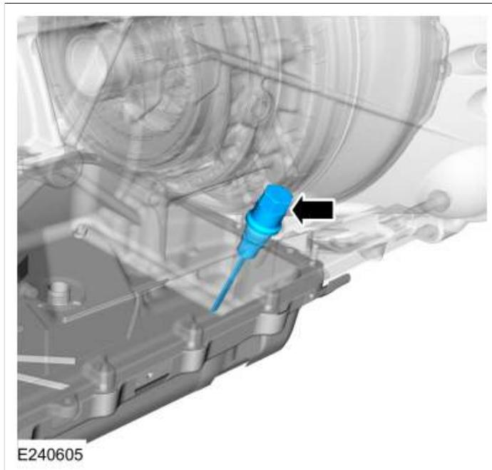
9. **NOTE:** The transmission fluid level indicator uses 1 through 6 to indicate the fluid level. The different numbers are for different vehicle models. Use the area between 4 and 5 when checking the transmission fluid level. The correct transmission fluid level is between 4 and 5 on the transmission fluid level indicator.
