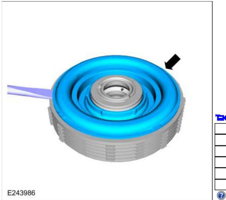
171. Remove the E clutch balance dam and discard the E clutch piston.
