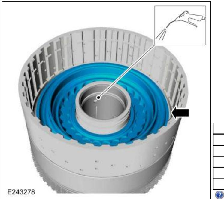
107. Remove and discard the C clutch piston inner and outer seals.
