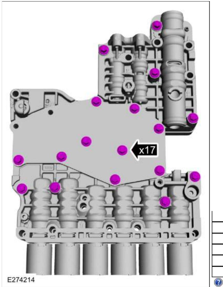
10. Remove and discard the valve channel plate.
