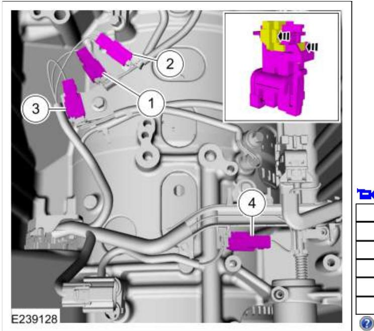
306. If removed, install the transmission fluid pump driven gear inner cover and the bolts.
