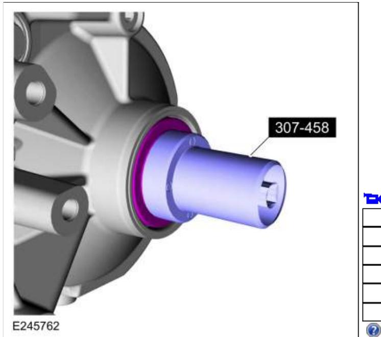
230. If removed, install the anti-ting ring.
