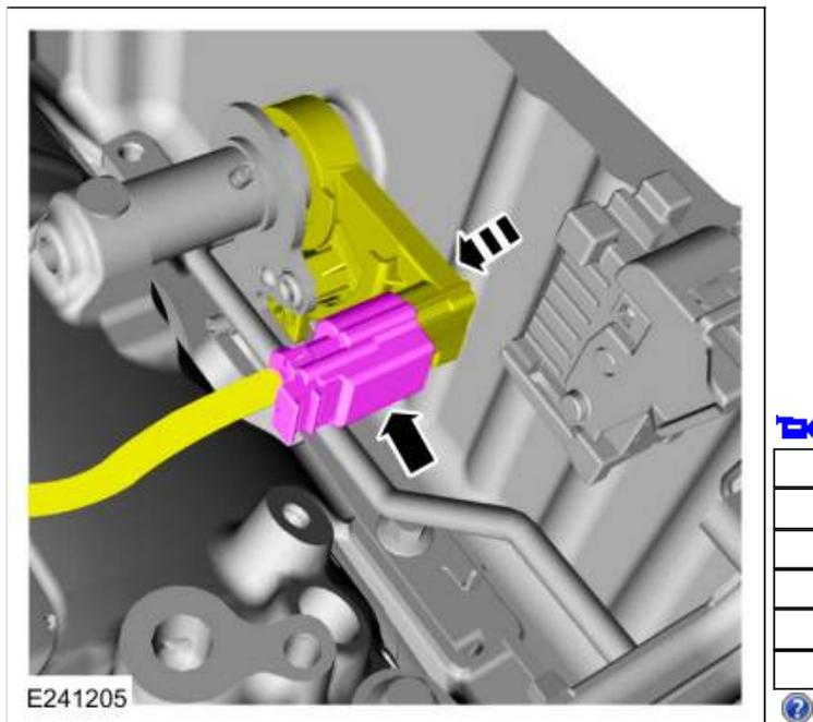
4. **NOTE:** After connecting the electrical connectors, slide the plastic lock to the locked position.
