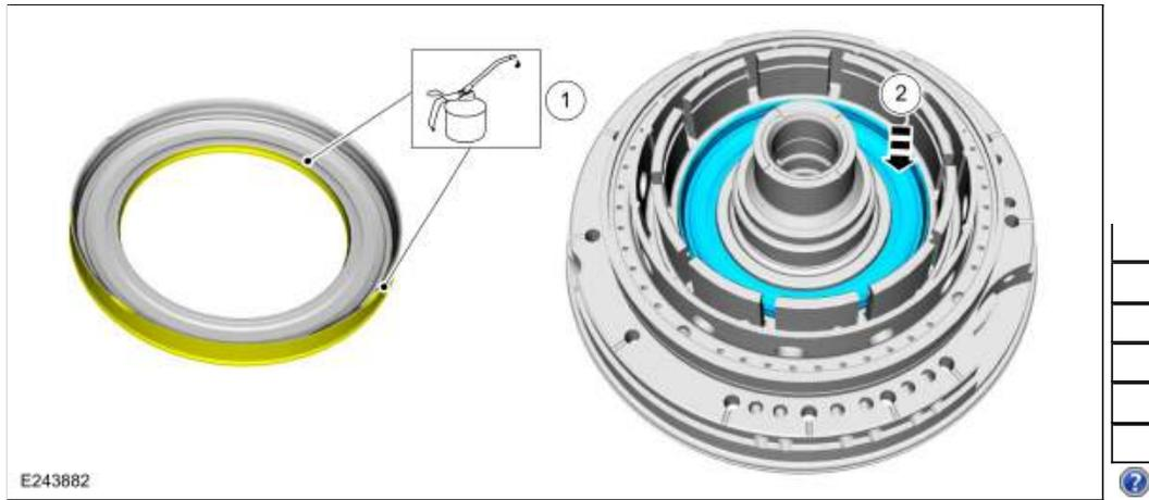
271. Install the B clutch apply plate.
