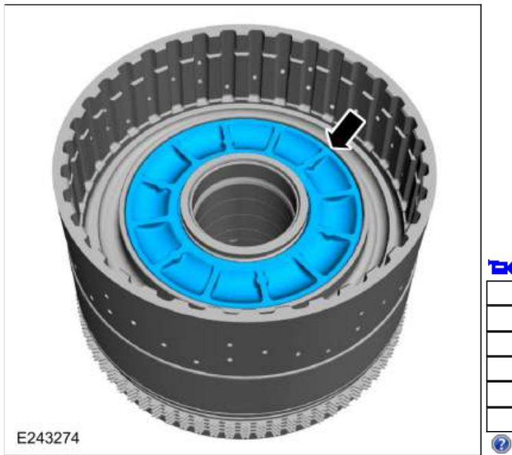
104. Remove the C clutch piston return spring.
