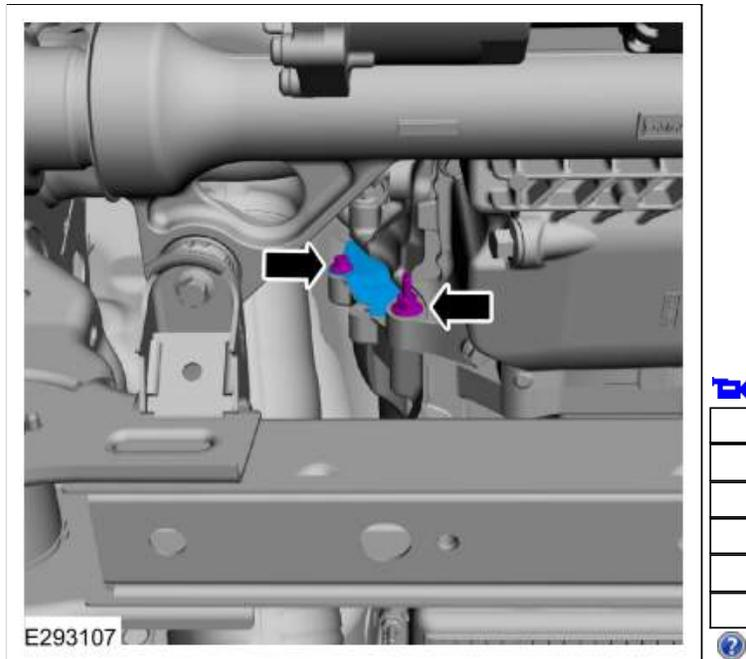
21. **NOTICE:** Do not pull on the wire harness to disconnect the electrical connector or damage to the electrical connector will occur.
