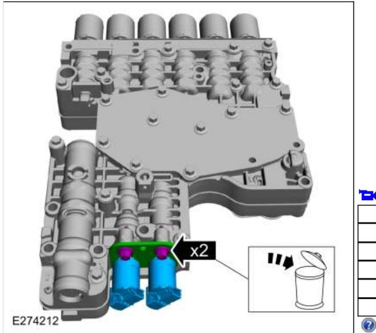
8. Remove bolts and the shift solenoid retaining plate.
