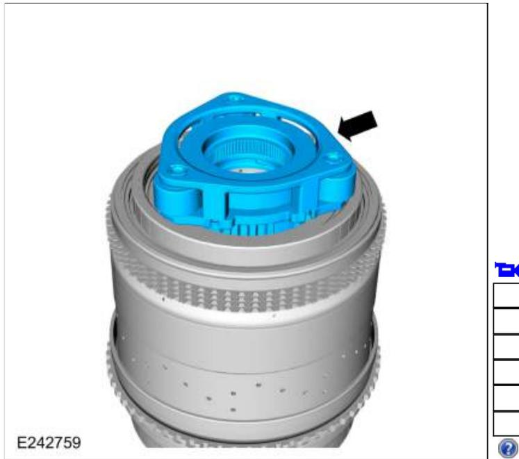
72. Inspect the No. 3 planetary carrier and the No. 3 sun gear.
