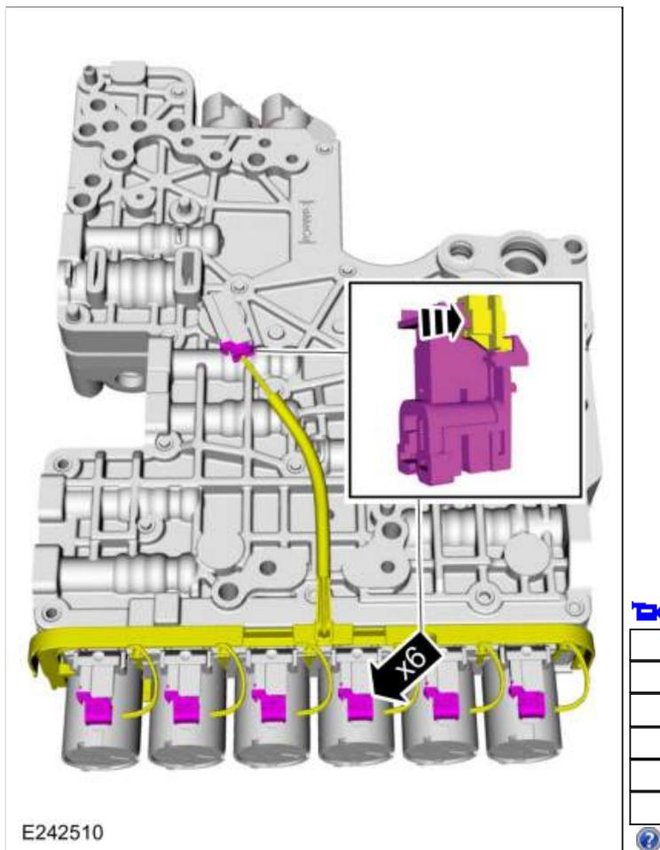
8. Connect the internal wiring harness.
