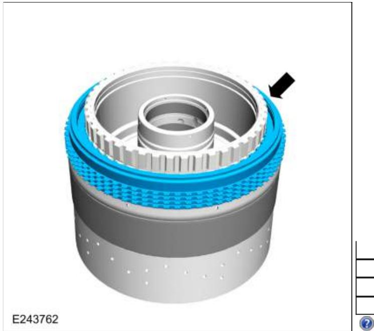
117. Remove the F clutch apply ring.
