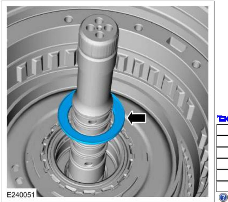
284. Using the special tools and a depth gauge, measure the distance from the top of the special tool to top of the (T3) thrust bearing in 2 different places. Average the measurements. Record this as measurement A. Use Special Service Tool: [307-661 Gauge, End Play.](#)
