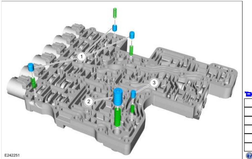
14. **NOTICE:** Note the location of the retaining clips, caps, valves and valve springs for assembly. Failure to install the components in the correct location will result in harsh/soft or no shifts or damage to the transmission.
