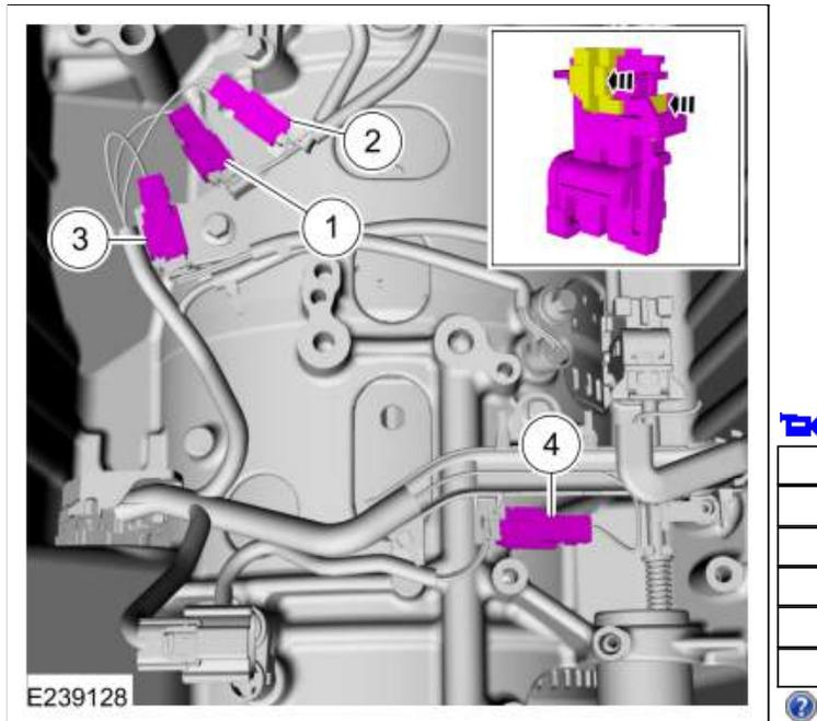
39. Remove the speed sensors.
