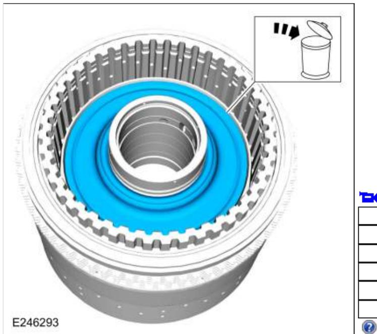
112. Remove the D clutch piston return spring.
