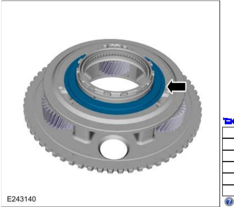
88. Remove the ring gear No 1 snap ring.
