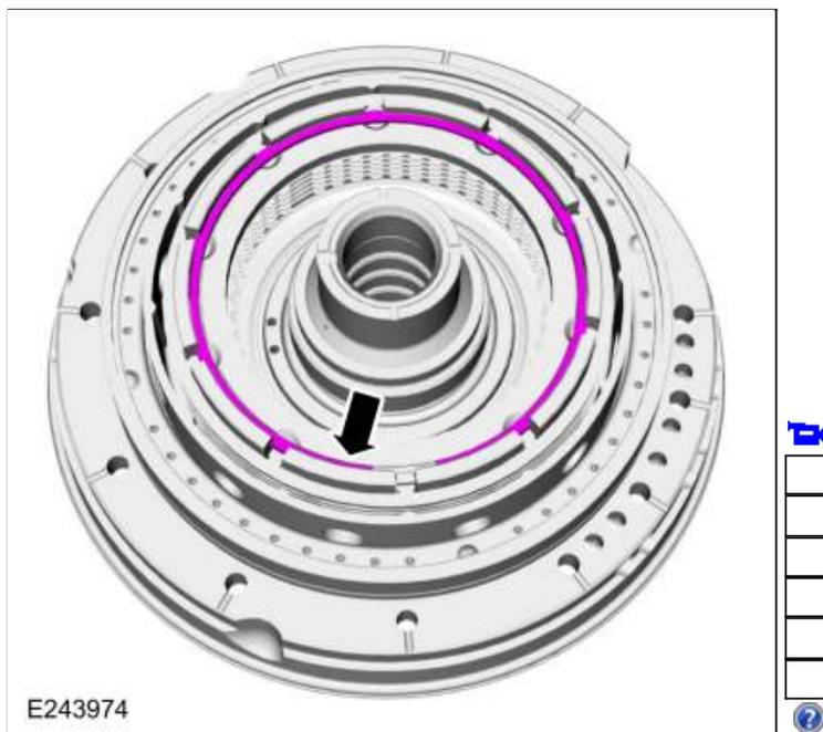
277. Remove the B clutch assembly.
