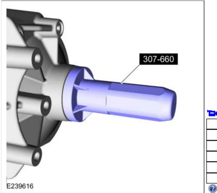
226. Install new seals on the output shaft.
