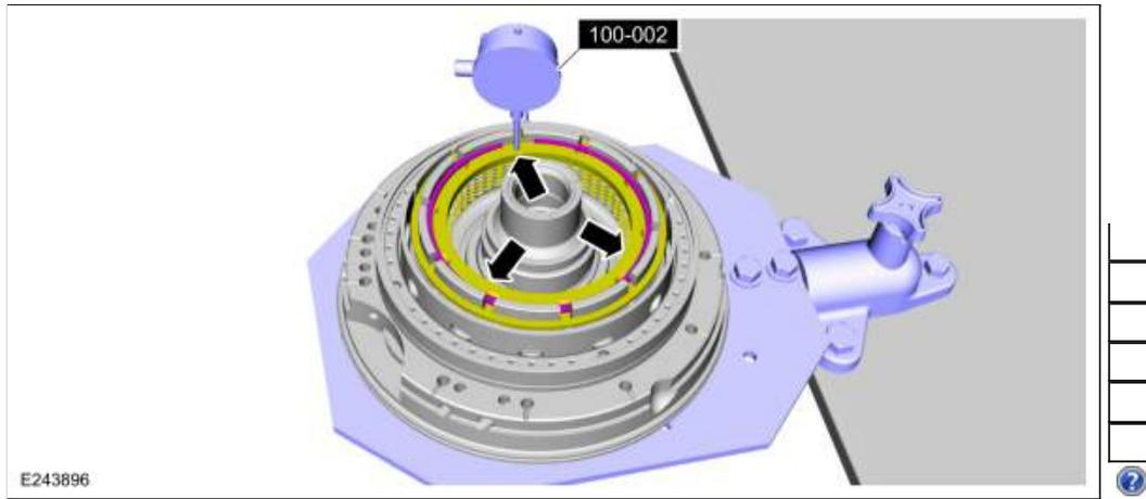
276. Remove the B clutch snap ring.
