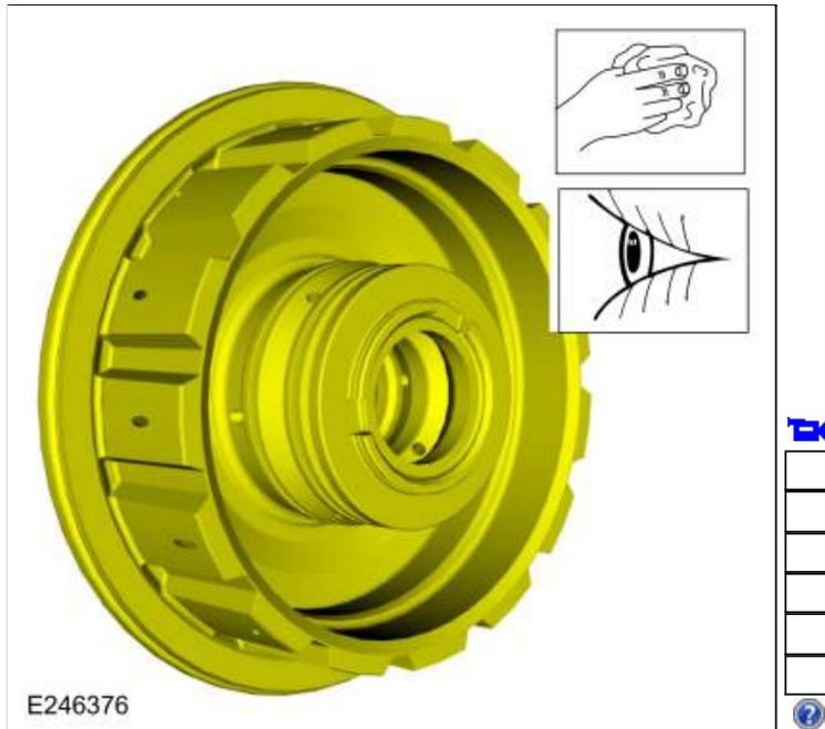
177. Install the new E clutch piston and balance dam inner seals. Lubricate the seals with petroleum jelly.
