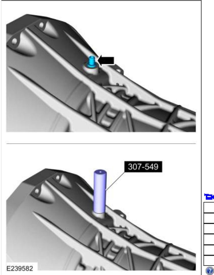
2. **NOTE:** *This step is only necessary if the transmission case is being replaced.*
