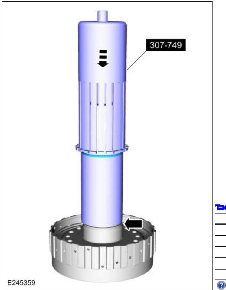
100. Install the special tool to size the 4 Teflon® seals. Allow the special tool to stay on the No 3 sun gear shaft for 5 minutes prior to final assembly.
