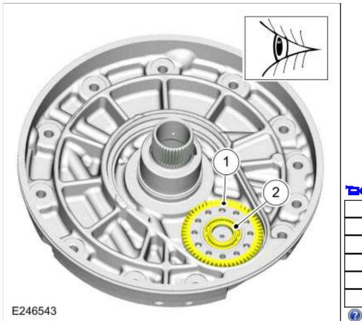
252. **NOTE:** Tighten the special tools evenly to remove the transmission fluid pump idler gear.
