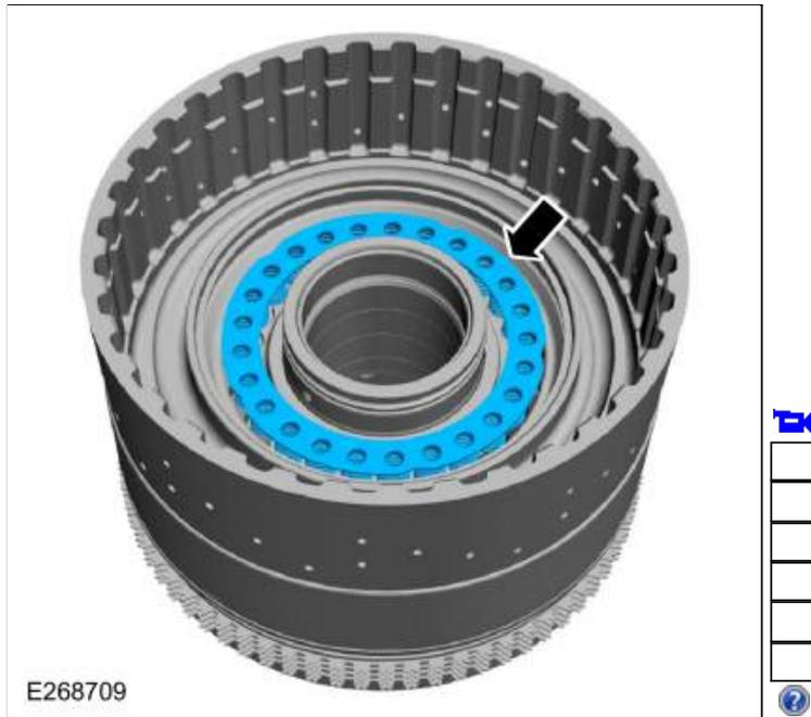
105. Remove and discard the C clutch balance dam inner and outer seals.
