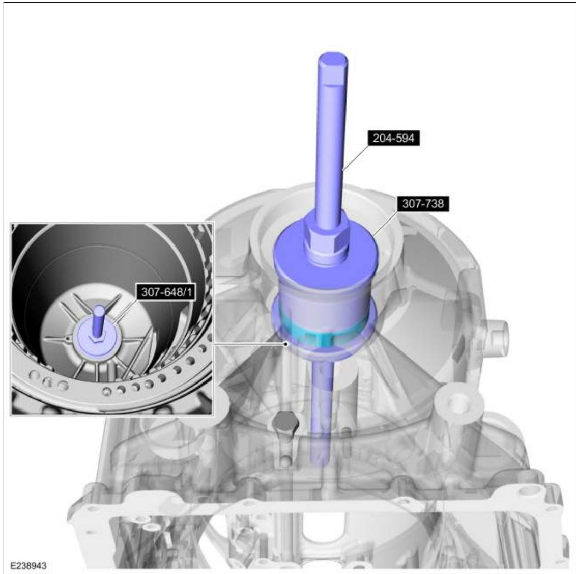
4. Using the special tools, install the fluid passage sleeve.
