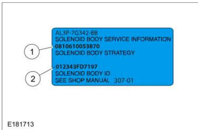
2. Using the scan tool, select module Programming and Programmable Parameters under the toolbox icon and select transmission. Follow the instructions displayed on the scan tool. There are fields to enter the solenoid body 12-digit identification and 13-digit strategy recorded from the solenoid body.
