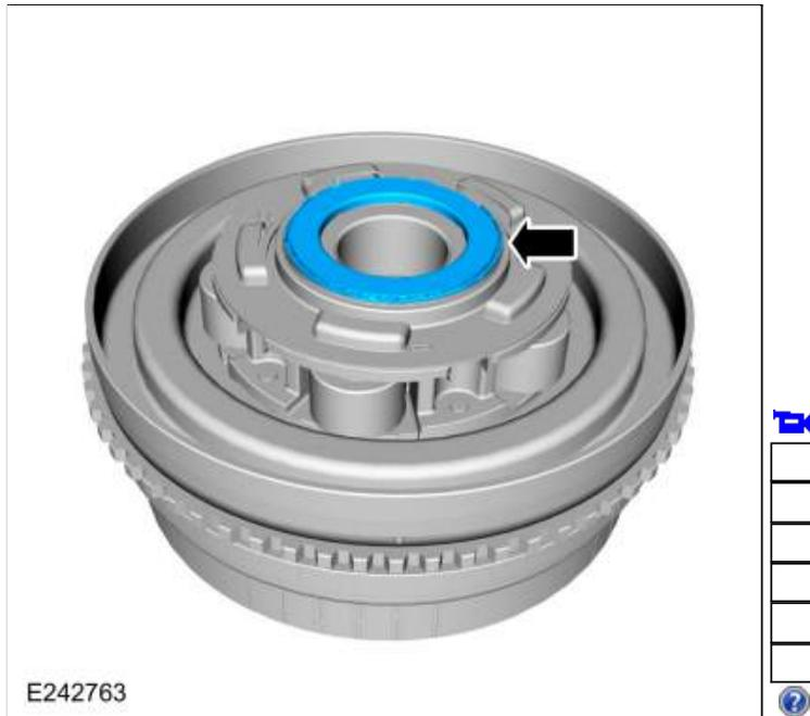
202. Remove Special Service Tool: [307-749 Installer/Sizer, R2-S3 Shaft Solid Seal](#).
