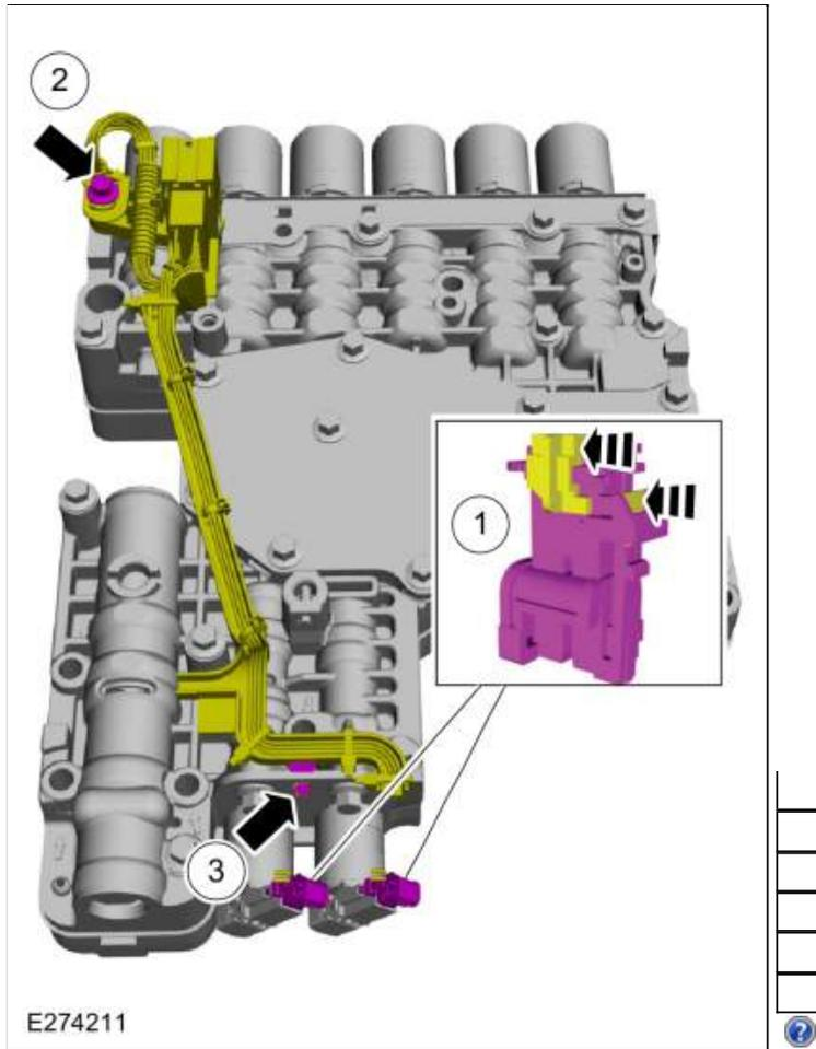
3. Disconnect the internal wiring harness electrical connectors.
