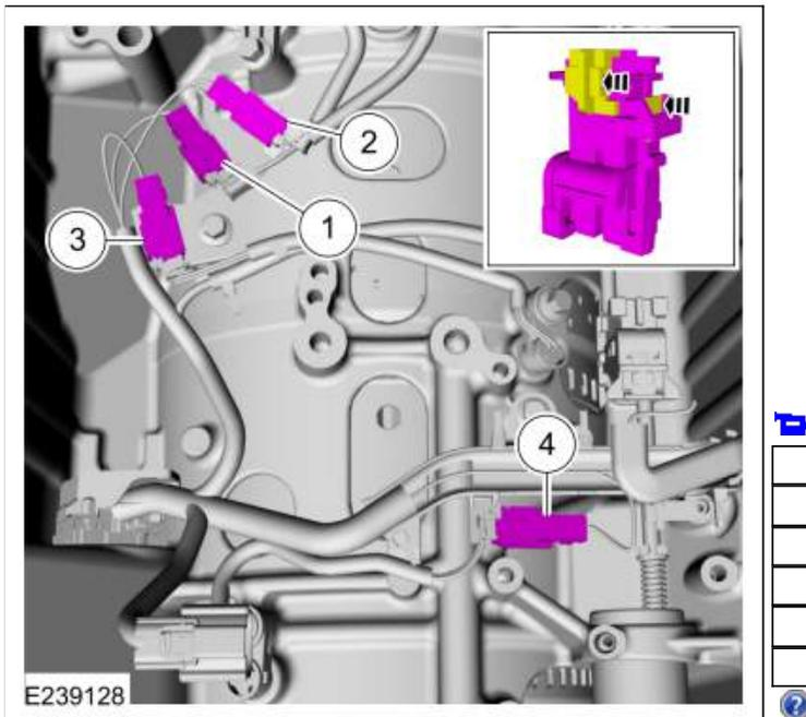
7. Disconnect the IR sensor electrical connector.
