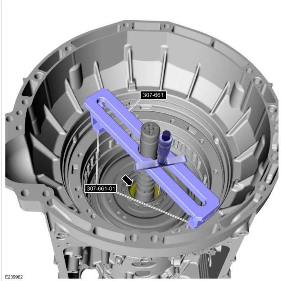
285. Using the special tools and a depth gauge, measure the distance from the top of the special tool to front support mating surface in 2 different places. Average the measurements. Record this as measurement B.
