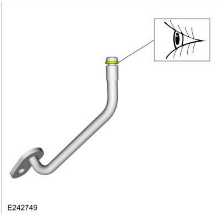
4. Install the transmission fluid auxiliary pump tube and loosely install the bolt.
