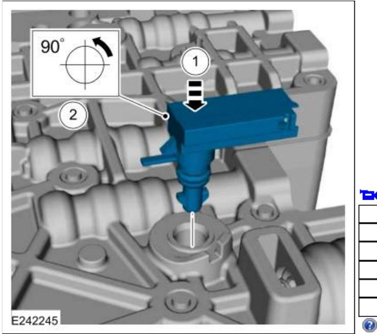
33. Connect the internal wiring harness electrical connectors.
