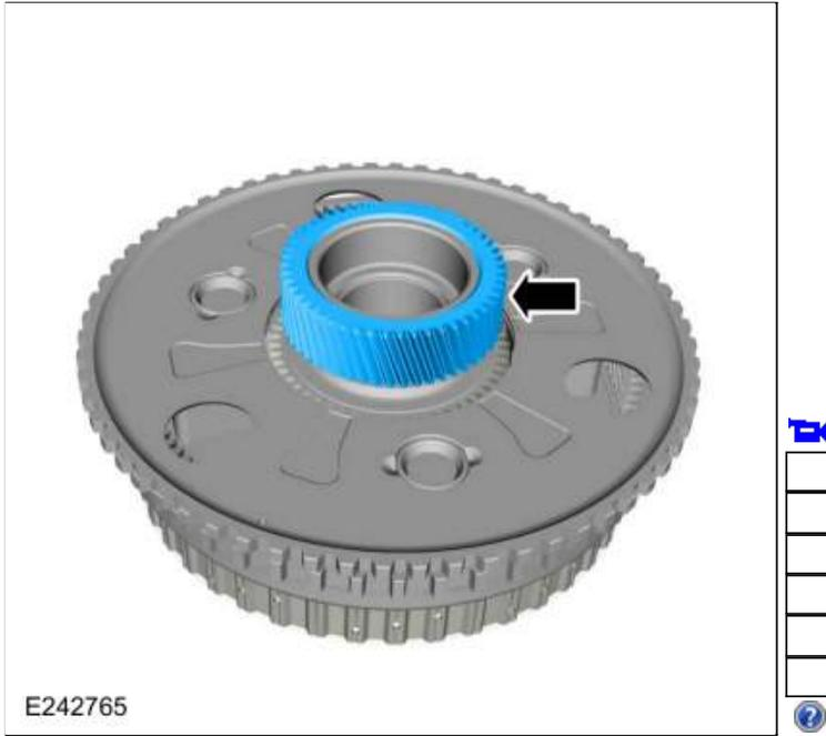
200. Install the No. 2 planetary carrier.
