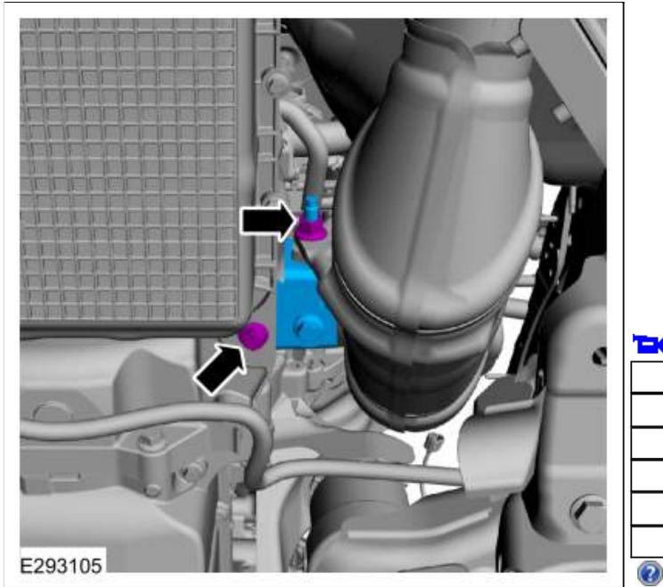
19. If equipped , position aside the engine block heater cable.
