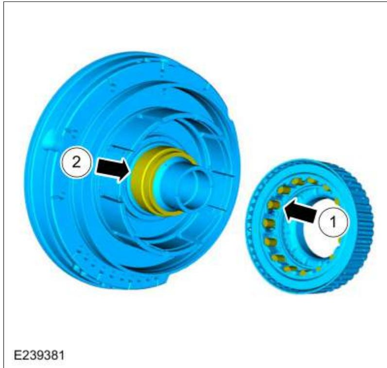
The One-Way Clutch (OWC) is a brake clutch that holds the sun gears No. 1&2 in one direction and allows it to freewheel in the opposite direction eliminating engine braking in 1st gear when the transmission is in drive. The rollers of the One-Way Clutch (OWC) lock to a inner race that is part of the front support assembly.
