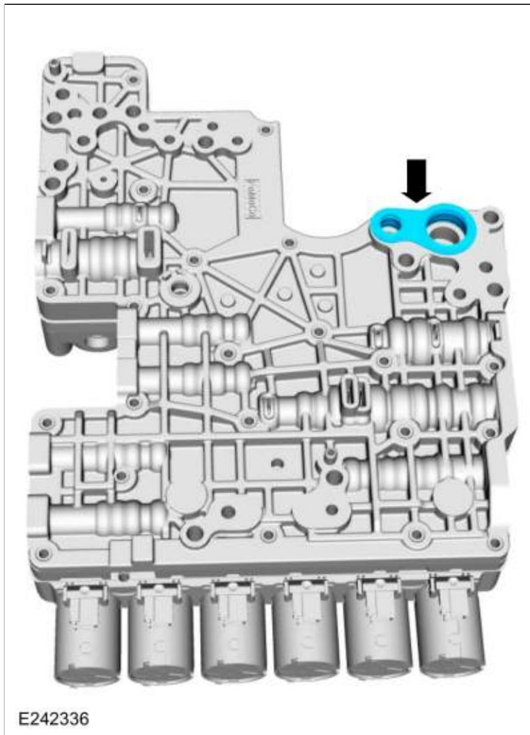
2. **NOTICE:** Do not install a 71 mm length bolt in the location shown or the transmission clutch and planetary container will be damaged and result in transmission failure.
