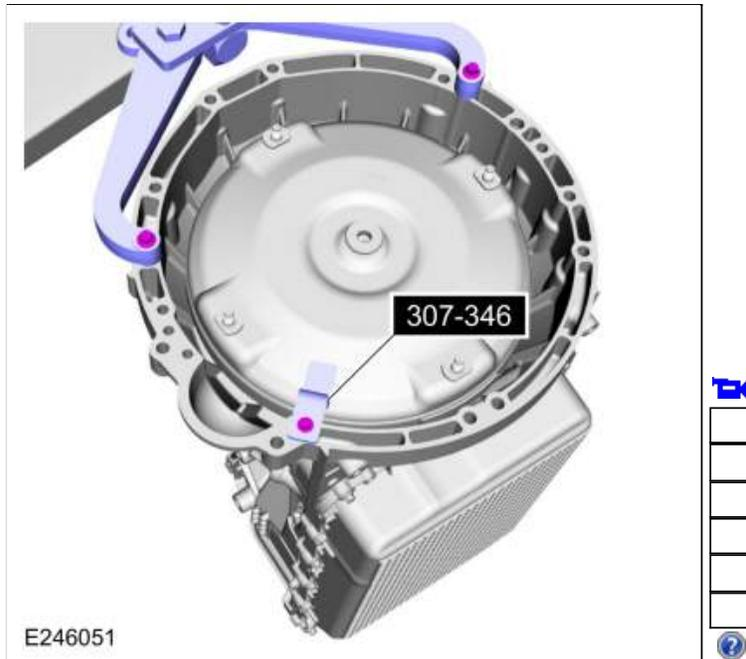
5. Using the special tool, remove the torque converter.
