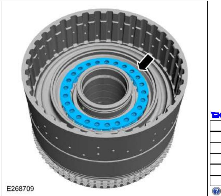
151. Install the C clutch balance dam.
