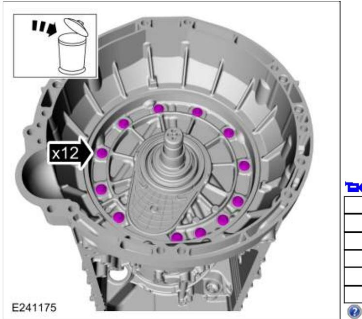
55. **NOTICE:** Be careful not to contact the transmission fluid pump drive gear, or damage to the gear can occur.
