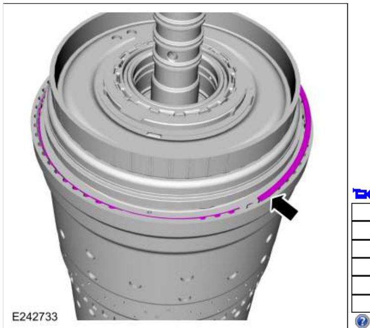
67. Flip the clutch and planetary assembly over with the input shaft through a hole in the bench. Remove the No. 1 planetary carrier snap ring and remove the clutch and planetary container cylinder.
