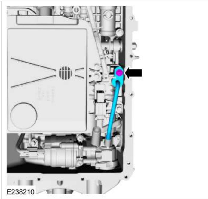
30. Remove and discard the transmission fluid auxiliary pump tube seal.
