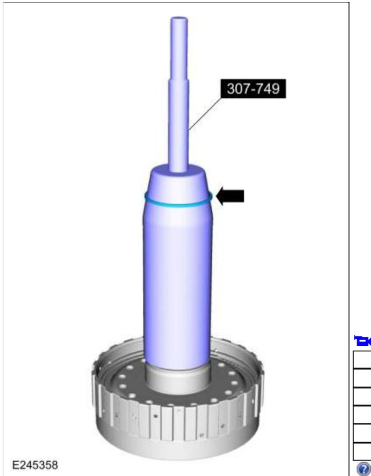
99. Using the top half of the special tool, slide the Teflon® seal into the groove. Remove the special tools and repeat the steps for the other 3 Teflon® seals.
