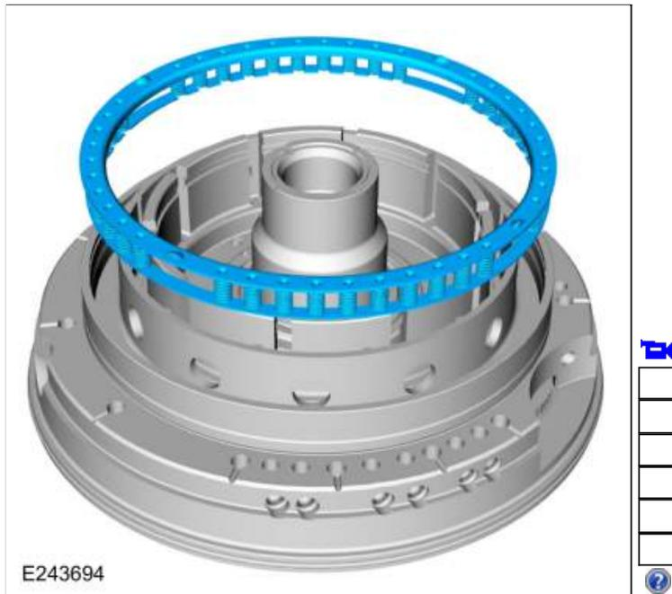
244. Use compressed air into the oil passage hole and remove the A clutch piston.
