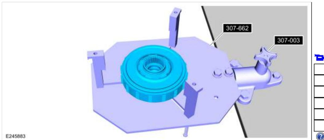
186. Using the special tool, measure the E clutch clearance. Position the plunger so it rests on the top surface of the pressure plate. Zero the dial indicator. Pull up on the pressure plate and measure and record the clutch clearance in 3 different places. Average the 3 recorded clutch clearance measurements and compare the measurement to the clutch clearance chart in specifications to determine the correct size pressure plate. Install the correct E clutch pressure plate.
