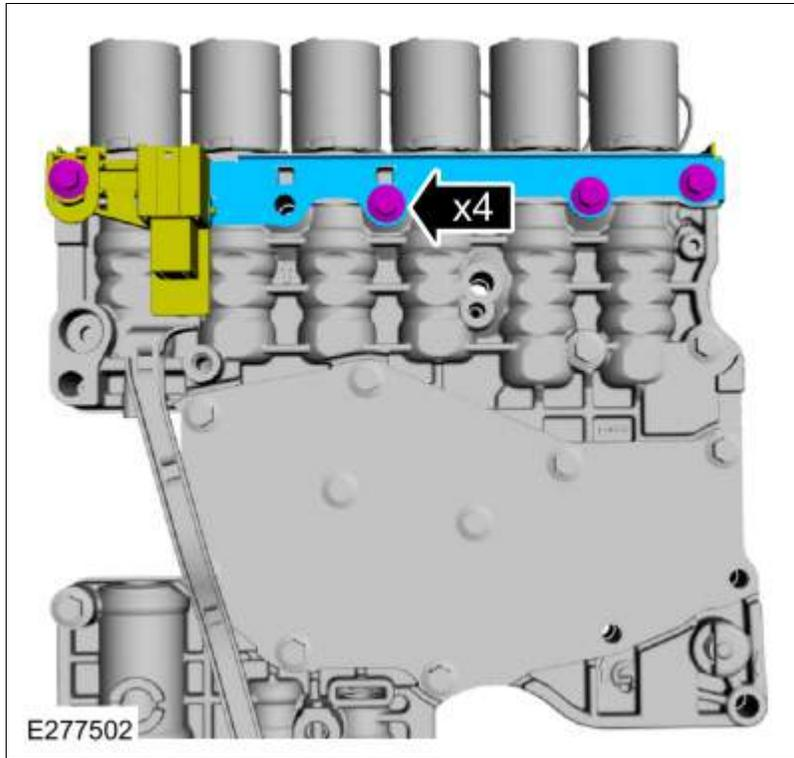
12. If replacing more than one solenoid, number the solenoids and number the main control valve body solenoid ports to correspond to the solenoid.
