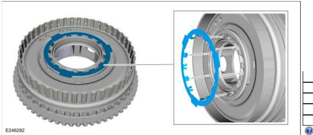
96. Remove and discard the sun gear No. 3 shaft Teflon® seals.
