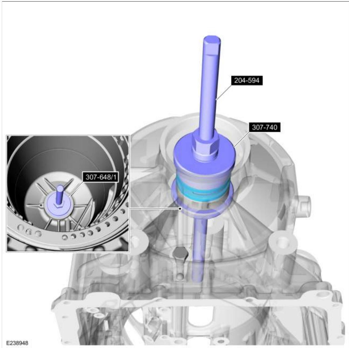
5. Using the special tools, install the outer output shaft bearing.
