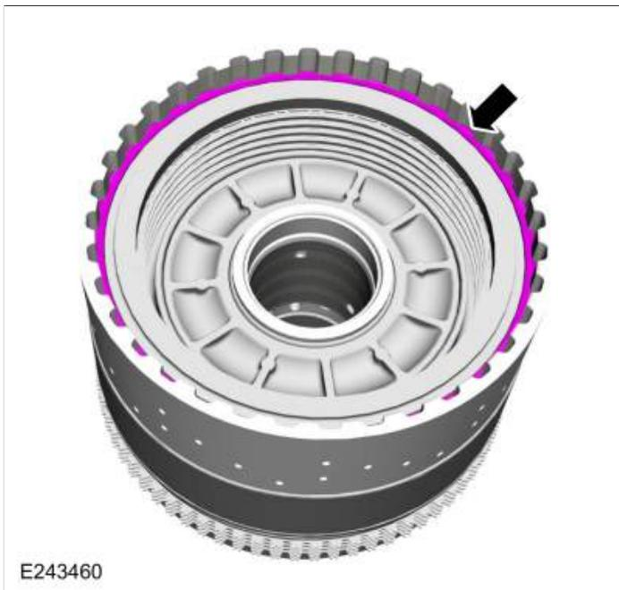
155. Assemble the special tools and position the CDF clutch cylinder with the C clutch facing up.
