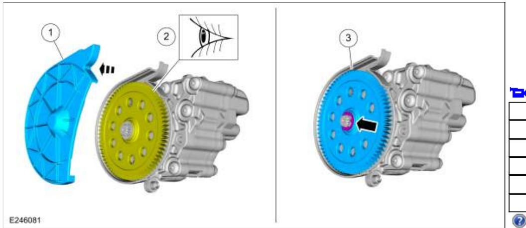
45. If necessary, remove the bolts and the transmission fluid pump driven gear inner cover.
