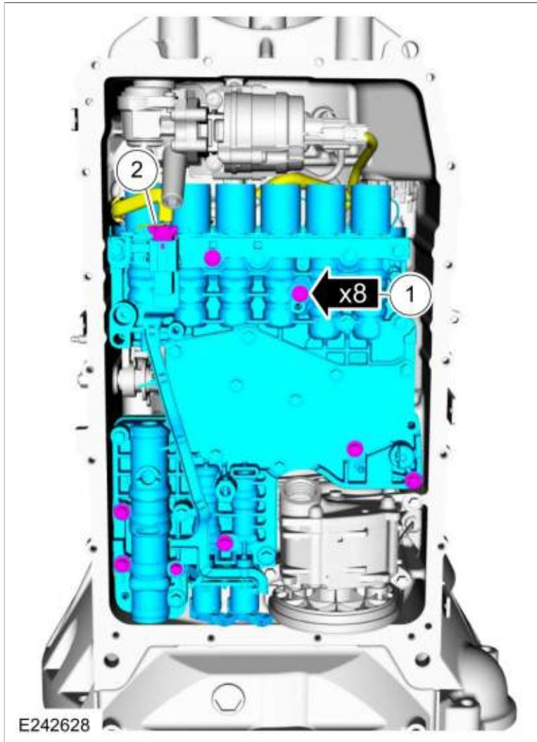
6. Remove the main control assembly to transmission fluid pump seal.
