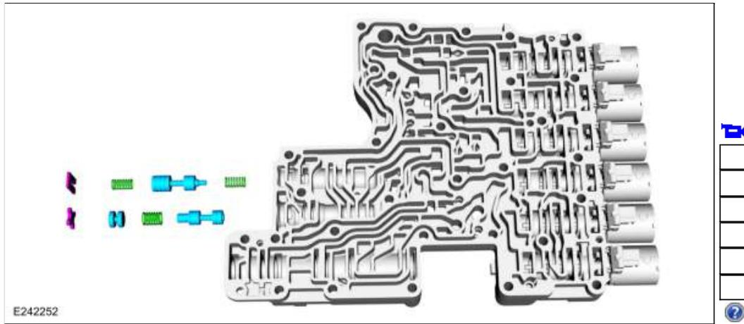
22. **NOTICE:** Solenoids are calibrated from the factory and are not all the same. To replace a solenoid, match the band number with the original solenoid or harsh shifts or damage to the transmission can occur.
