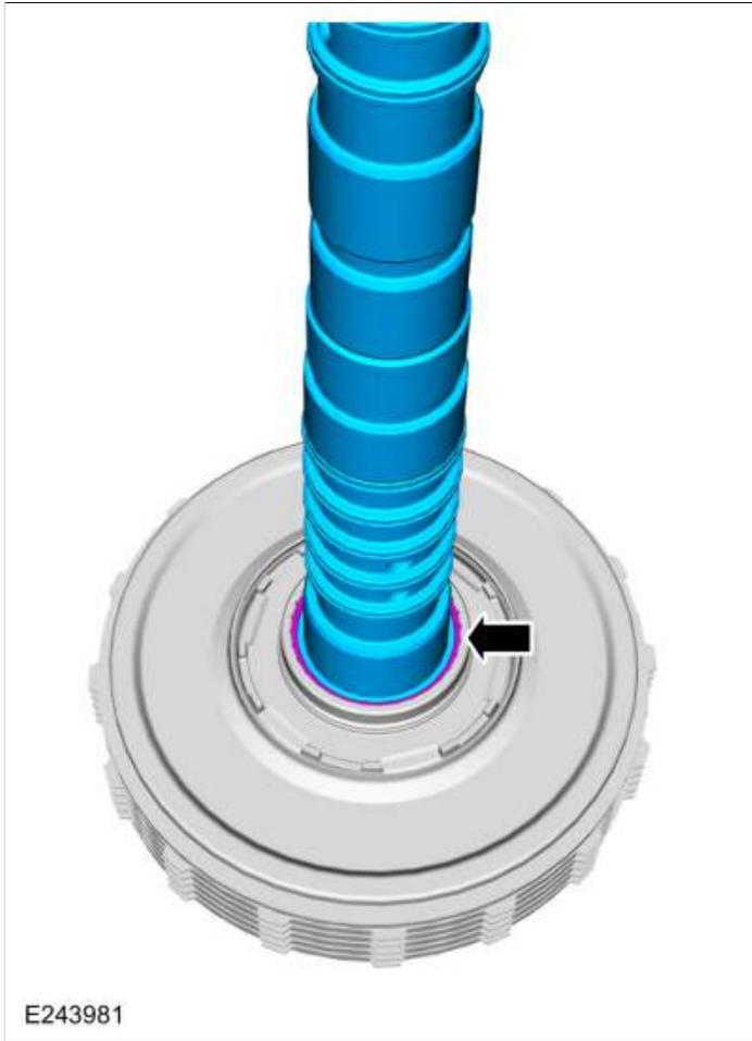
165. Remove and discard the input shaft-to-sun gear No. 3 shaft Teflon® seals.
