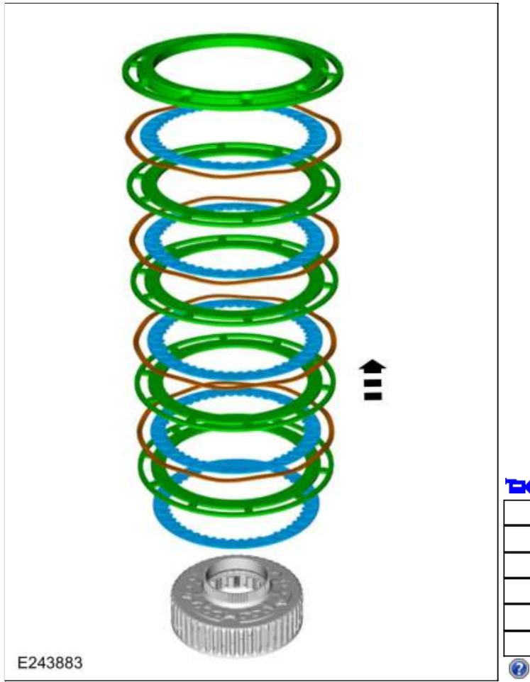
240. Remove the B clutch apply plate and the one remaining B clutch separating spring.
