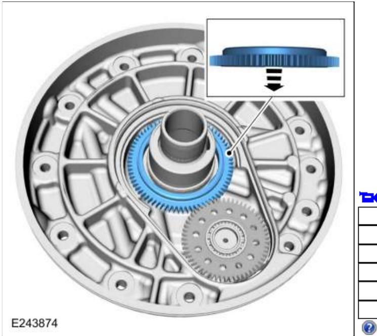
260. Install the front support cover by pressing down evenly by hand.
