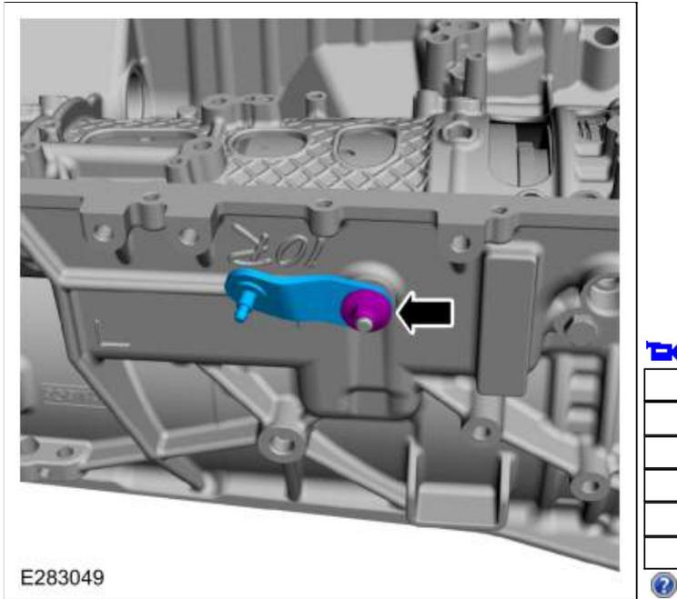
51. Remove the manual control shaft, the IR sensor and the park pawl actuator rod.
