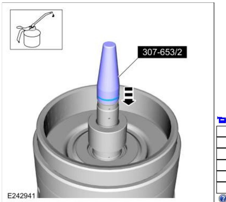
213. Using the special tool, size the Teflon® seal. Allow the special tool to stay on the input shaft for 5 minutes prior to final assembly. Use Special Service Tool: [307-653 Sizer, Input Shaft Teflon Seal](#).
