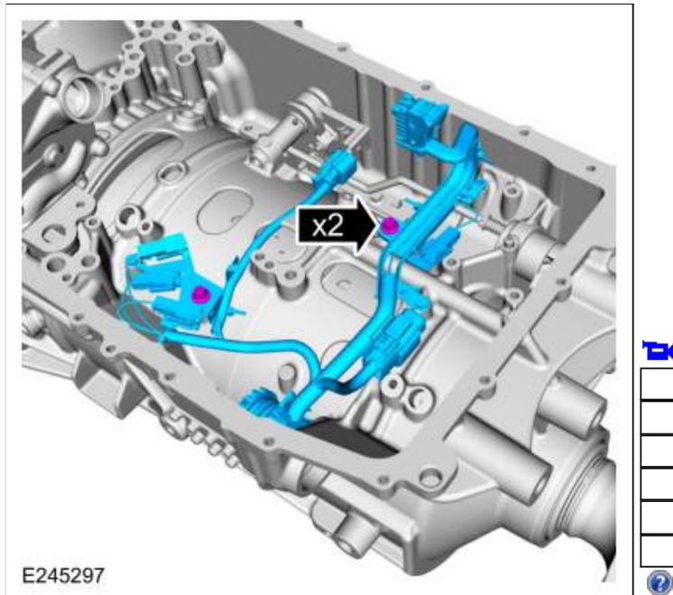
43. Remove the bolts and the transmission fluid pump.
