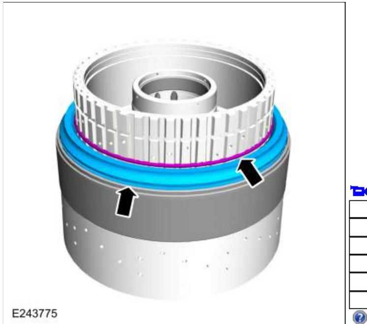
131. Using the special tools and a press, compress the F clutch balance dam and install the retainer into the groove.
