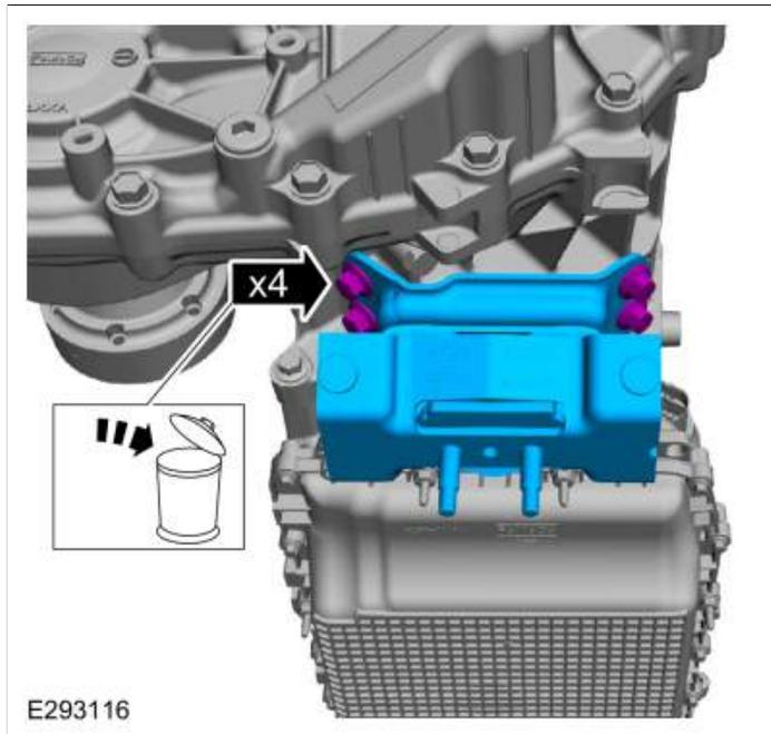
31. **NOTE:** If the transmission is to be overhauled or if installing a new or re-manufactured transmission, remove the transfer case.
