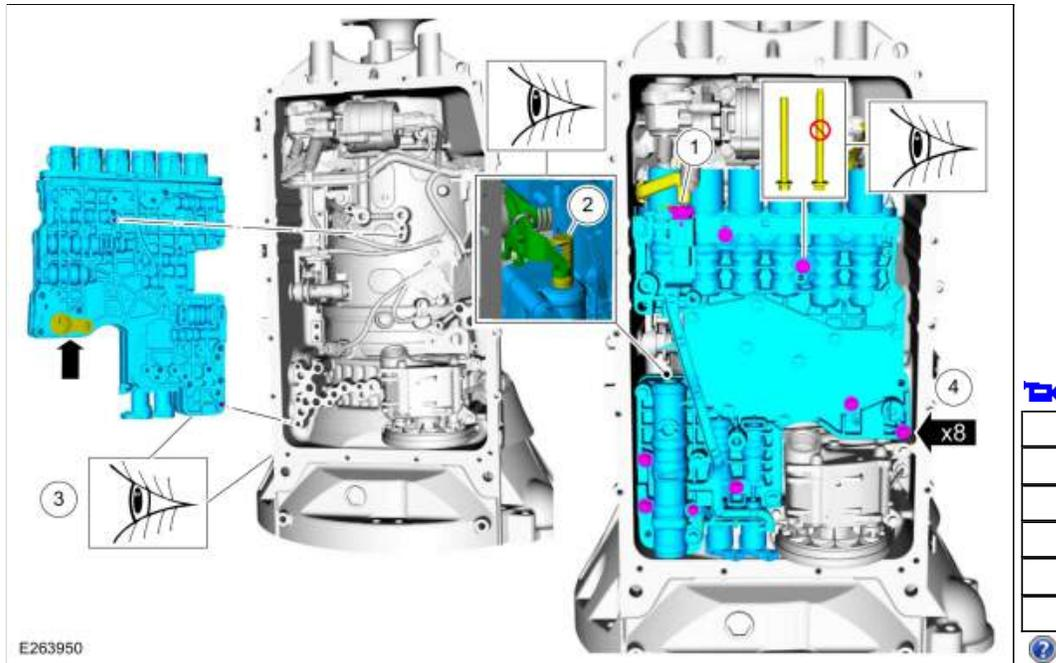
310. Tighten the bolts in the sequence shown.
