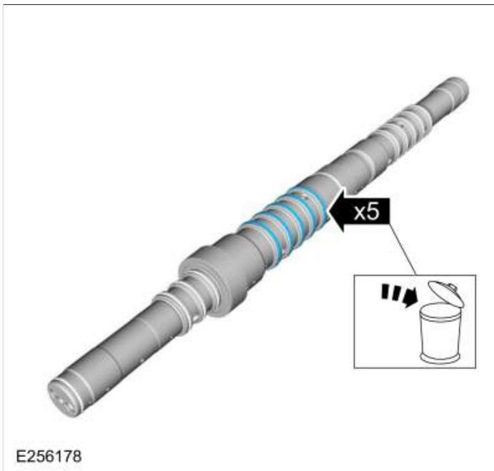
166. Remove and discard the input shaft D-ring seals.
