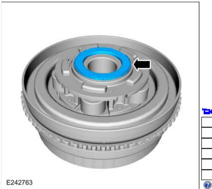
77. Remove the No. 2 planetary carrier.
