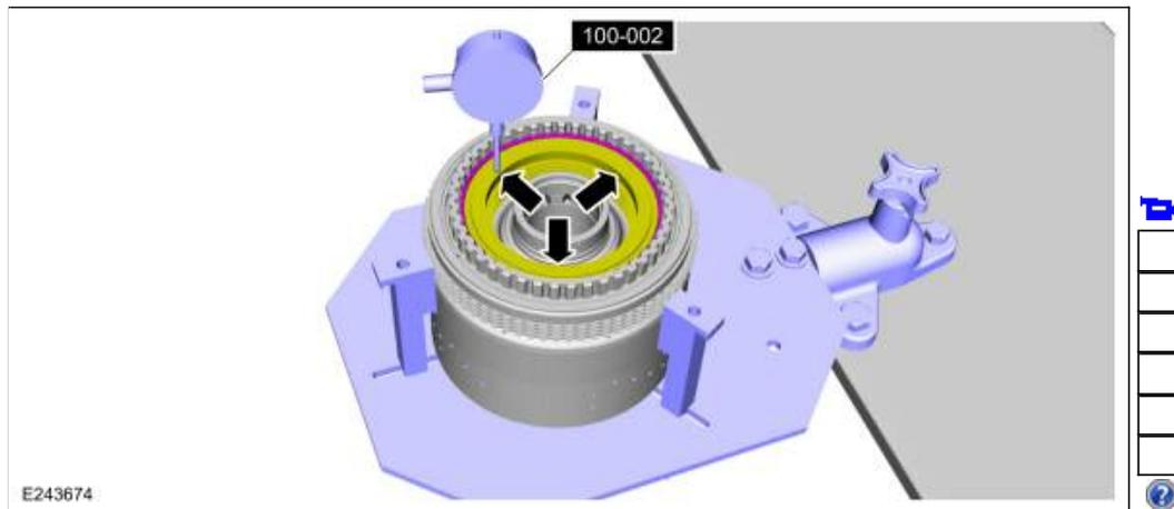
147. Install the new C clutch piston inner and outer seals. Lubricate the seals with petroleum jelly.
