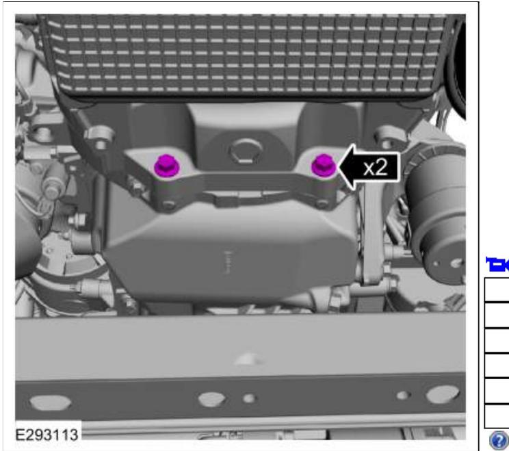
12. Install the RH bellhousing bolts.
