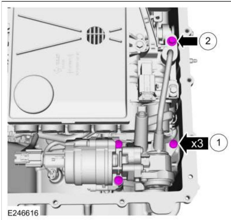
6. Connect the transmission fluid auxiliary pump electrical connector.
