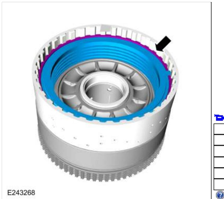
102. Using the special tools and a press, remove the C clutch balance dam retainer.
