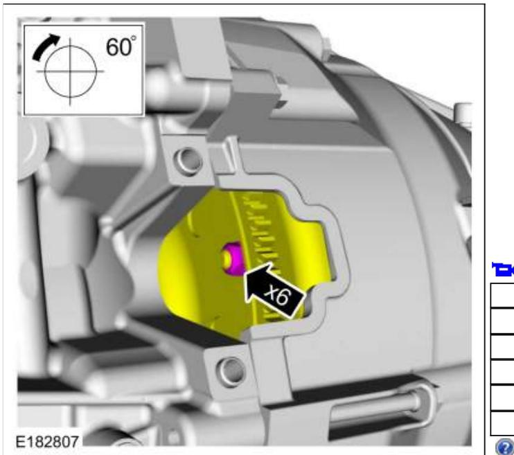
18. Install the starter motor insulator.
