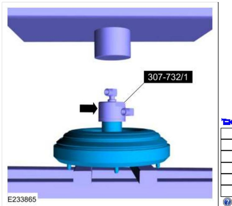
13. Using the special tool, install the slotted cap.
