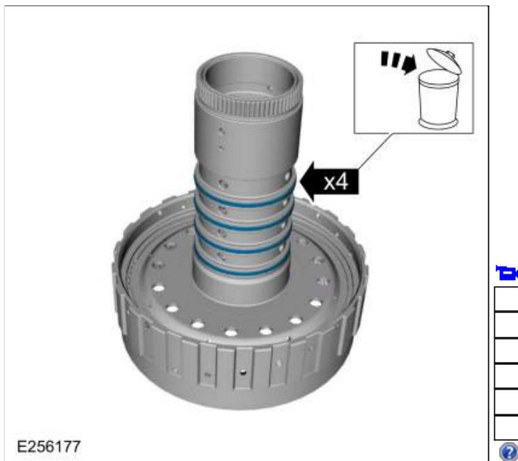
97. Install the special tool and adjust the special tool to align the bottom edge of the tool with the top edge of the bottom Teflon® seal groove.
