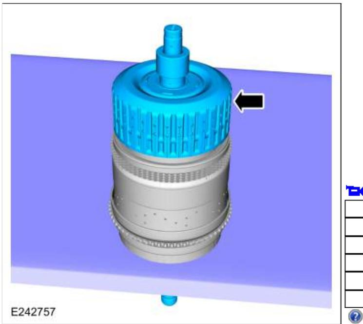
71. Remove the No. 3 planetary carrier and the No. 3 sun gear.
