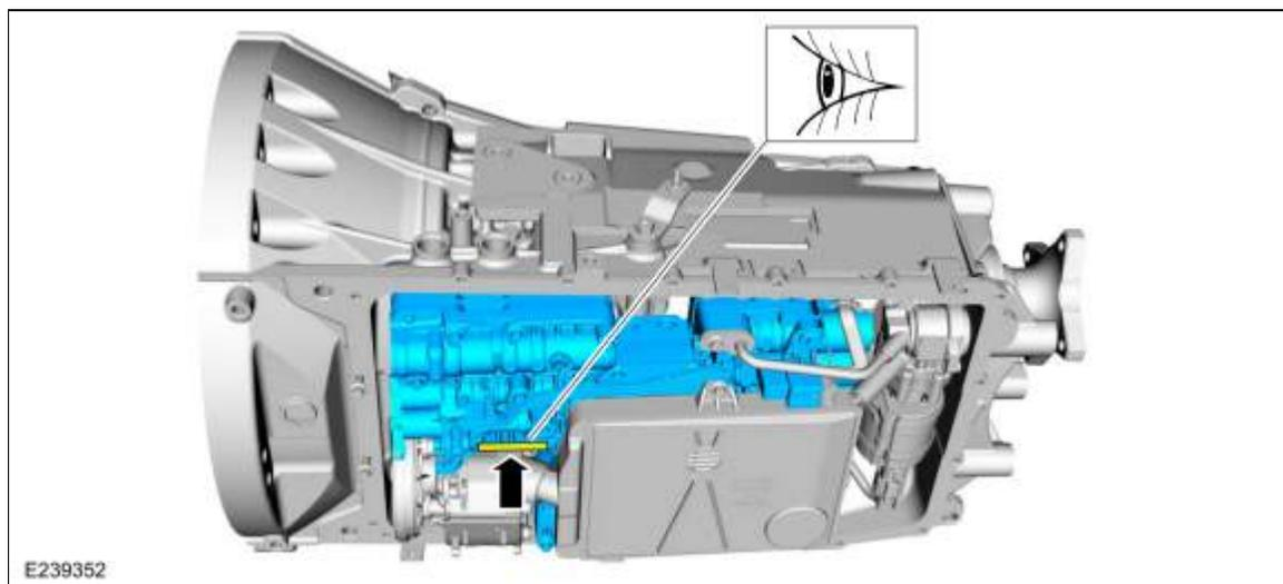
If the solenoid body strategy etched on the main control does not match what the scan tool displays, the solenoid body strategy must be downloaded into the PCM or TCM or harsh shifts will result.
