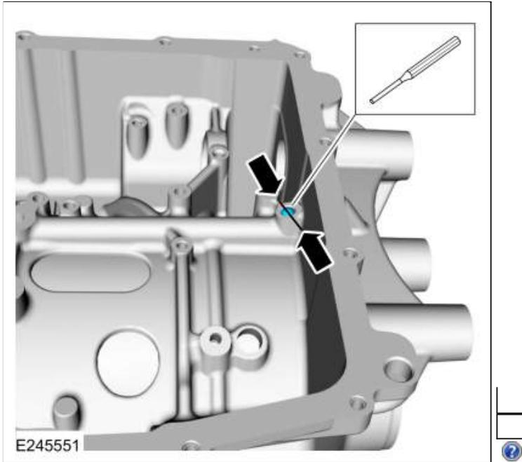
3. Using the special tools, install the inner output shaft bearing.
