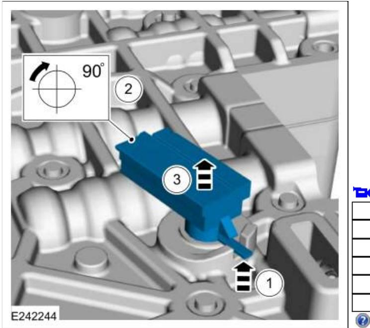
6. Remove the main control assembly to transmission fluid pump seal.
