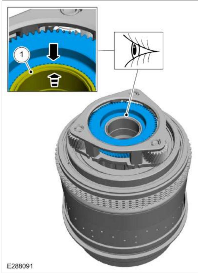
207. Remove Special Service Tool: [307-747 Installer/ Sizer , Input Shaft Solid Sealing Rings: Large.](#)
