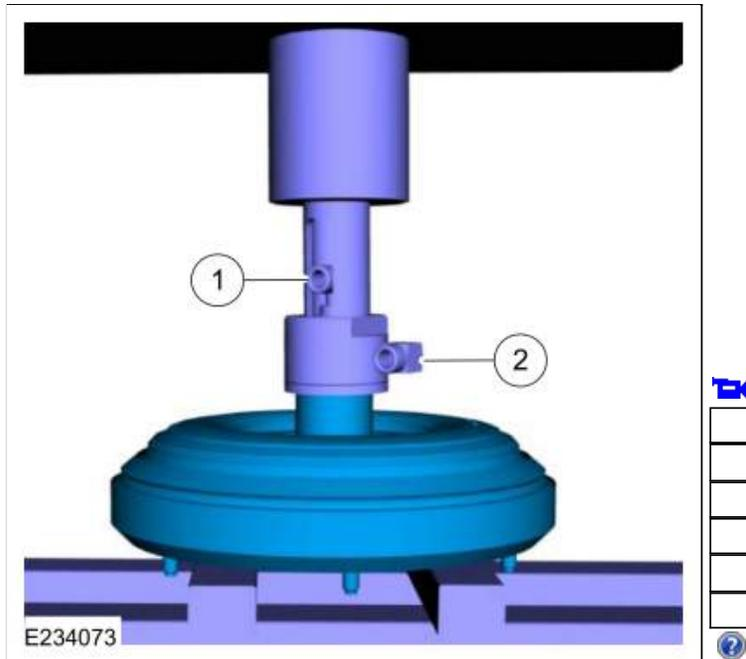
16. Follow the equipment instructions to purge transmission fluid from the torque converter prior to starting the flushing procedure.
