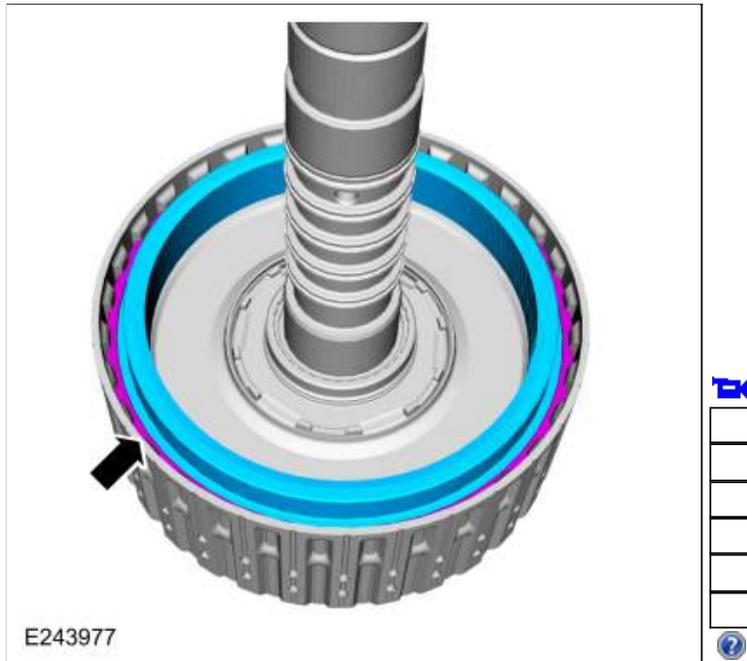
194. Install the special tool and adjust the special tool to align the bottom edge of the tool with the top edge of the bottom Teflon® seal groove.
