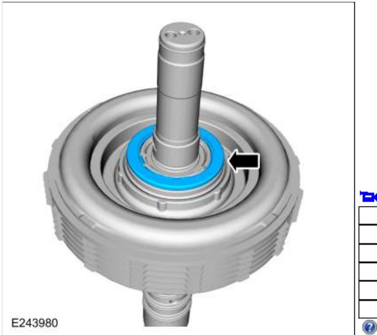
164. Remove the snap ring and remove the input shaft from the E clutch assembly.
