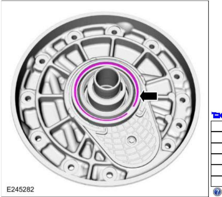
265. Install the new front support-to-case seal with the seal color visible from the outside.
