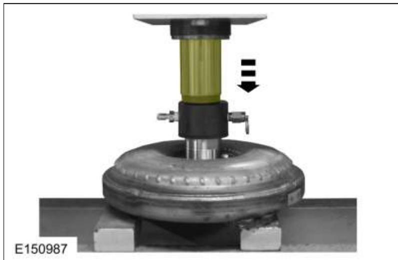
19. Connect a compressed air supply to the torque converter leak tester (307-421).
