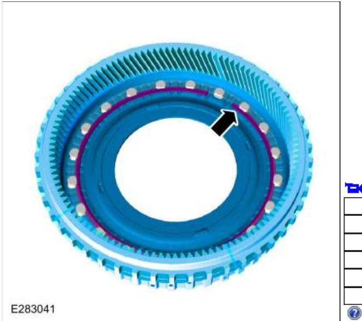
91. Install the ring gear No. 1 bearing.
