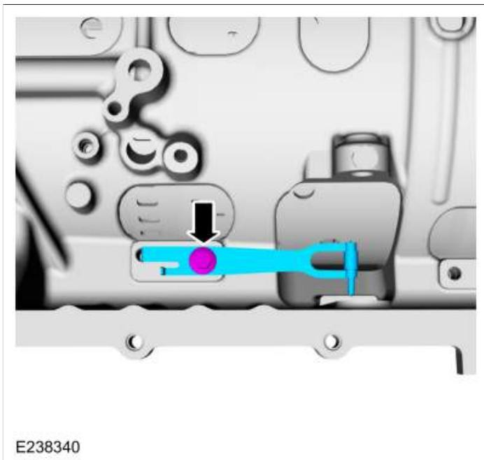
219. Install the park pawl actuator rod, manual shaft and the TR sensor.
