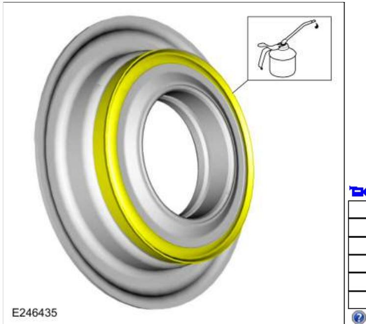
183. Install the new E clutch piston and balance dam in the E clutch hub.
