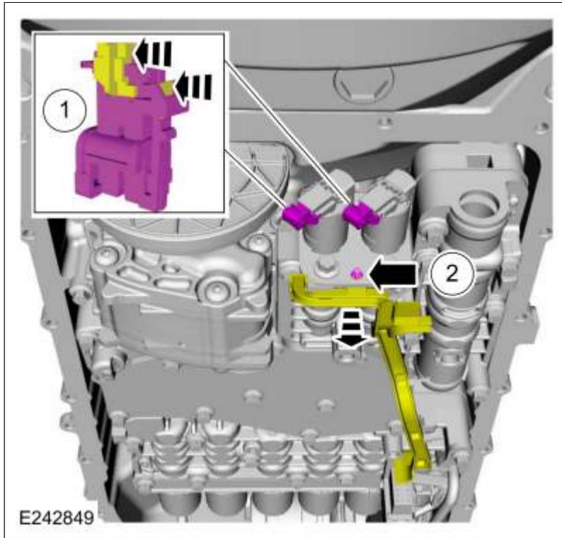
3. Remove and discard the bolts and remove the solenoid retaining plate.
