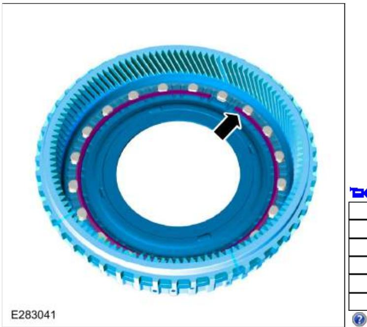
89. Inspect the A clutch hub, No. 1 ring gear and the No. 1 planetary carrier.
