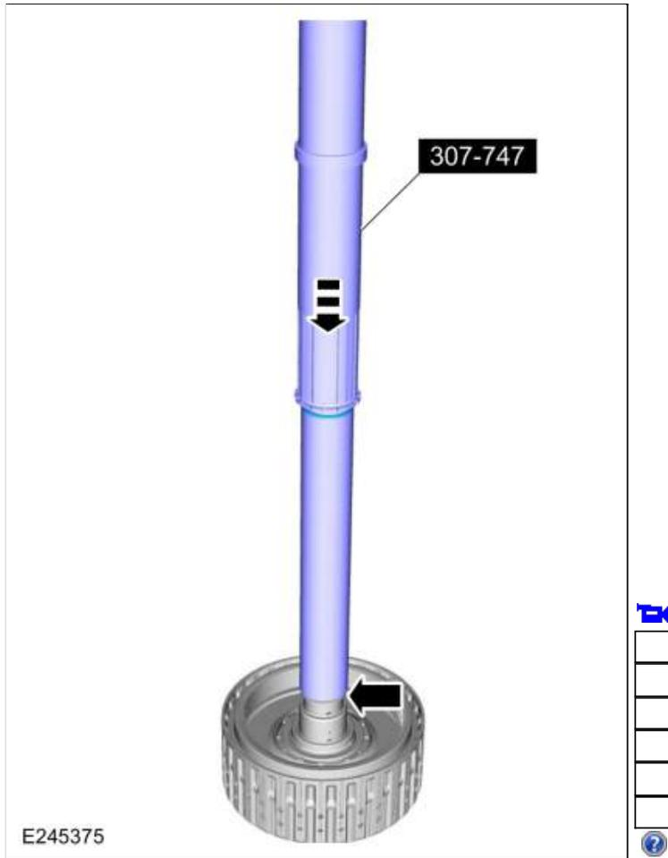
197. Install the special tool to size the 5 Teflon® seals. Allow the special tool to stay on the input shaft for 5 minutes prior to final assembly.
