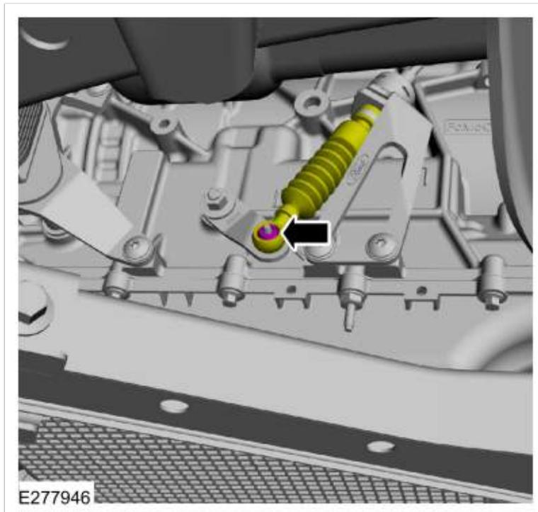
3. Disconnect the TR sensor electrical connector and position the transmission wiring harness aside.
