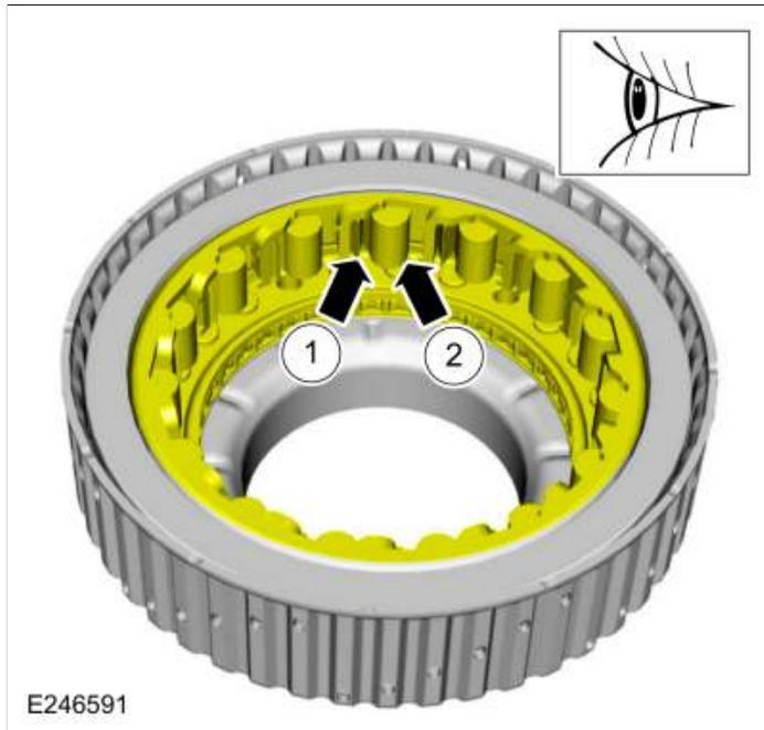
279. **NOTE:** The One-Way Clutch (OWC) hub should rotate counter-clockwise freely when installed correctly.
