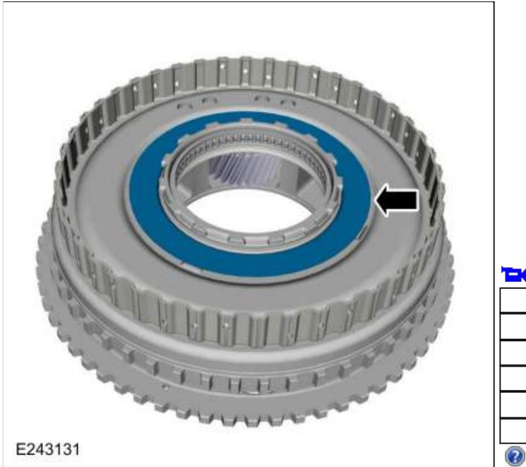
94. Install the ring gear No. 1 bearing support and rotate it counter clockwise to lock it.
