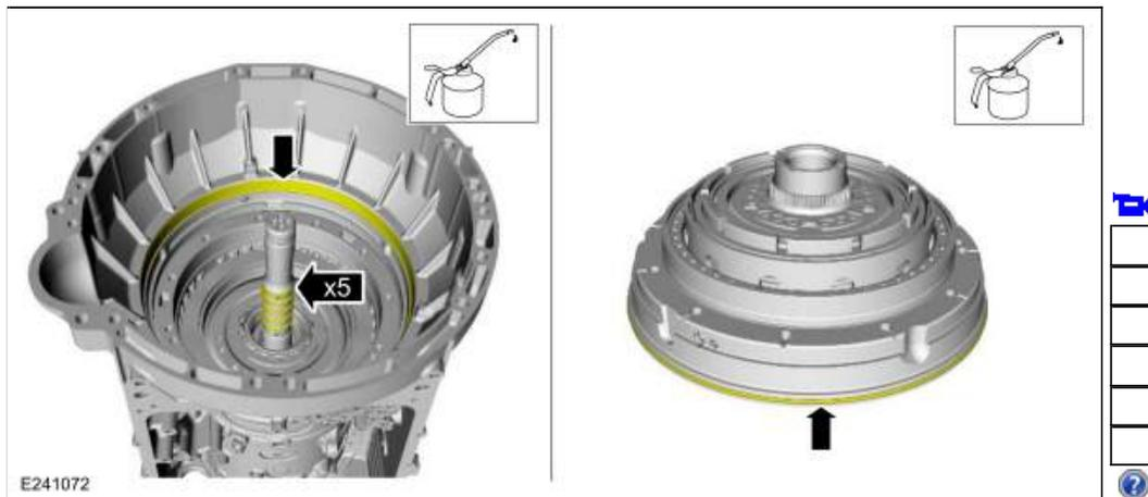
298. Install the front support into the transmission case. Align the pump gear to the pump drive gear pocket area. Rotate the input and output shafts to align the one-way clutch splines with the No. 1 sun gear.
