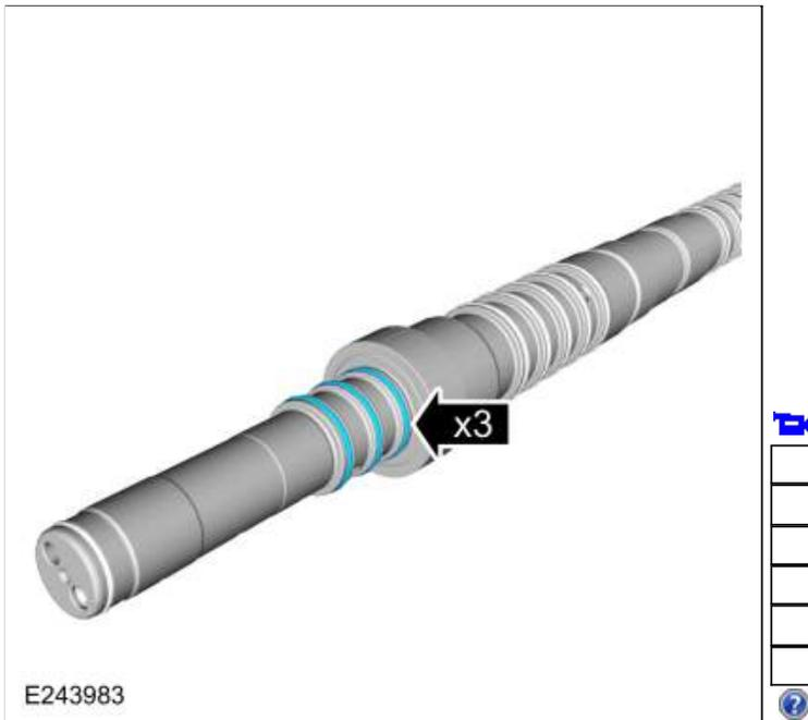
188. Install the input shaft in the E clutch and install the snap ring.
