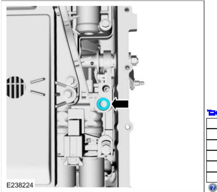
316. Inspect the transmission fluid auxiliary pump tube O-ring.
