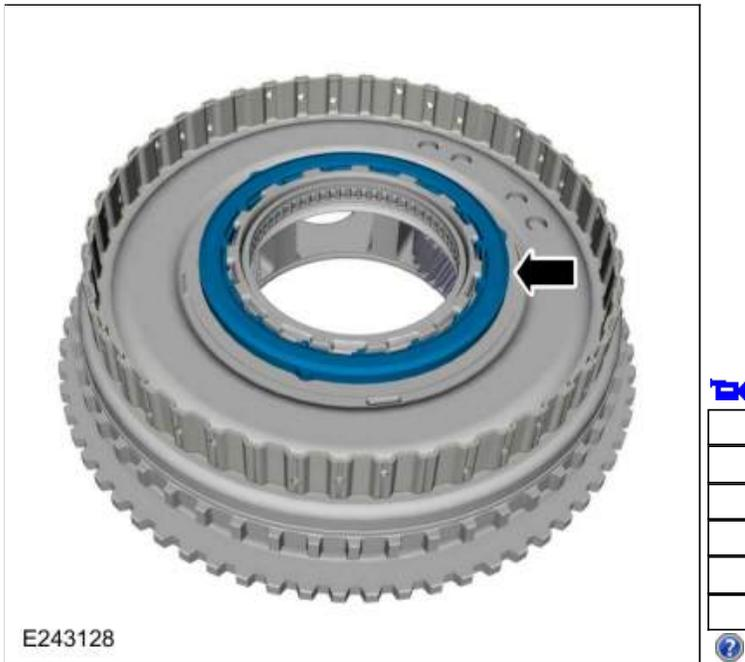
95. Align the tabs with the slots and install the No. 1 bearing support locking ring.
