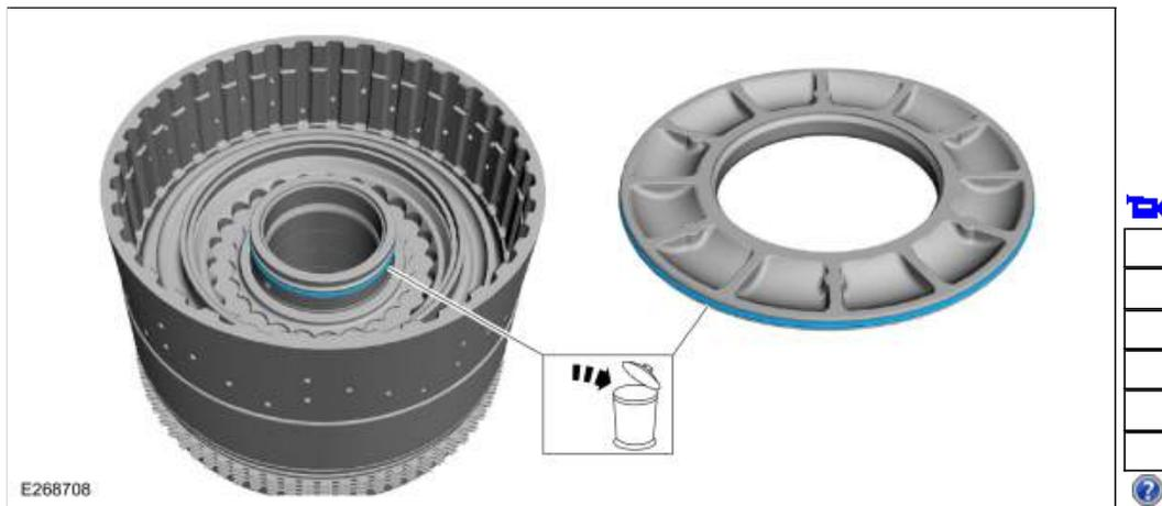
106. Remove the C clutch piston. Use compressed air into one oil passage hole while plugging the hole on the opposite side.
