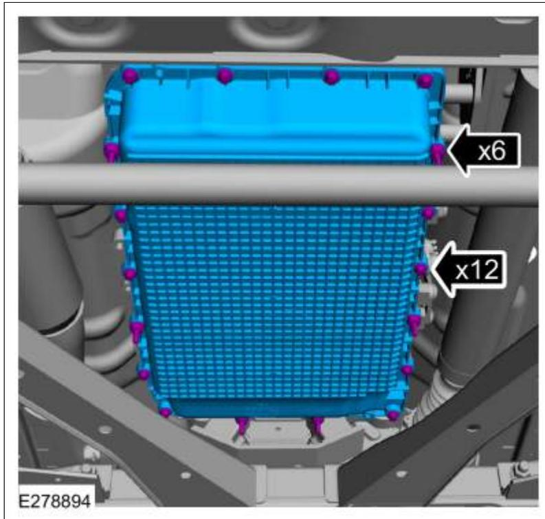
4. **NOTE:** *The transmission fluid pan gasket can be reused if not damaged.*
