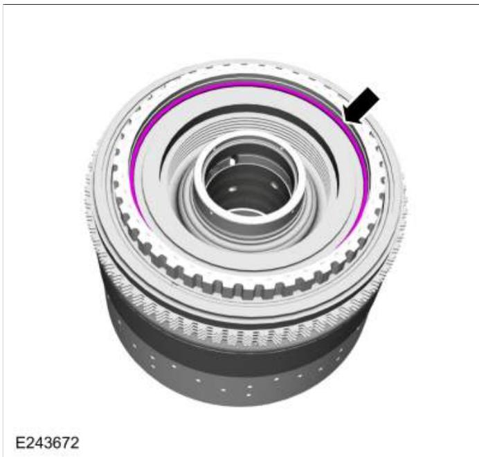
145. Assemble the special tools and position the CDF clutch cylinder with the D clutch facing up.
