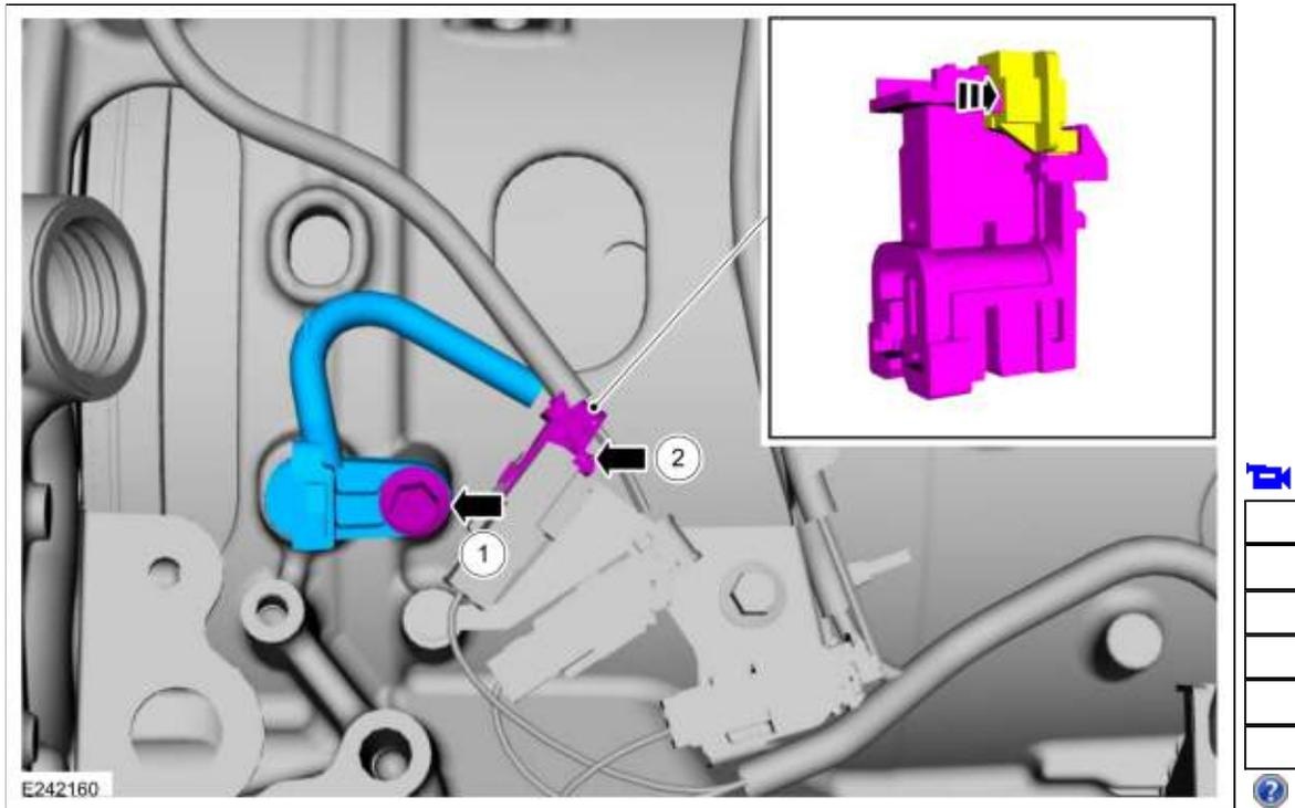
2. Install the main control valve body.
