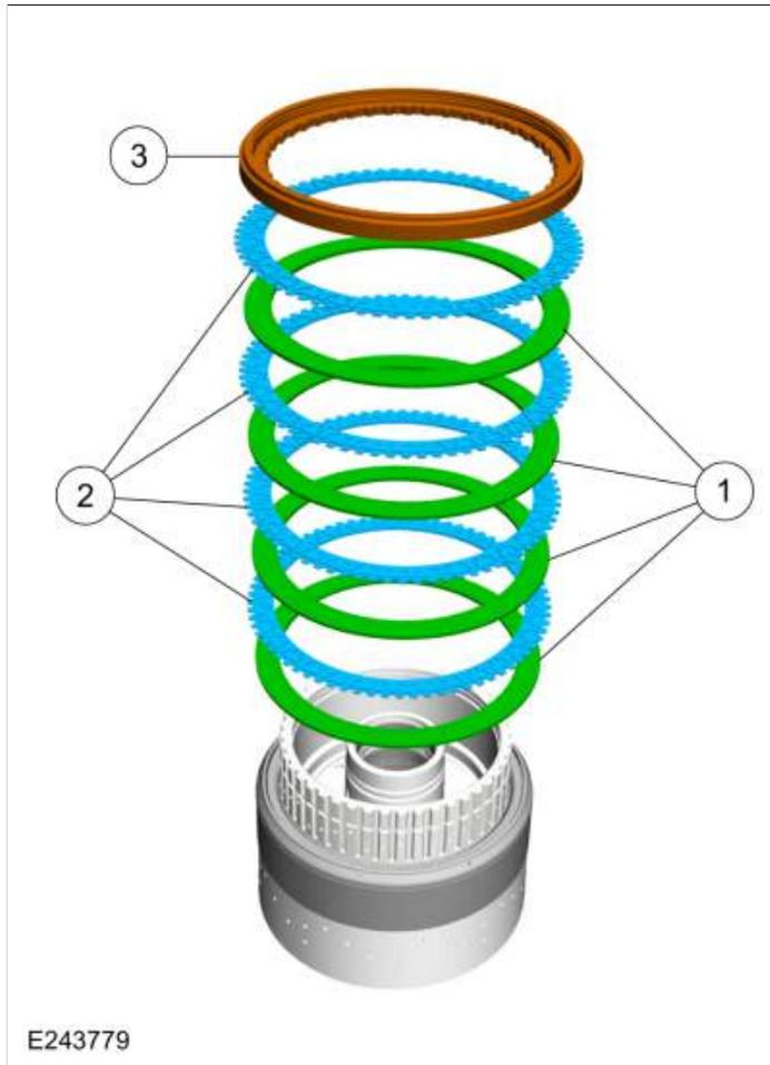
134. Install the F clutch snap ring, F clutch snap ring keeper and the F clutch keeper snap ring .
