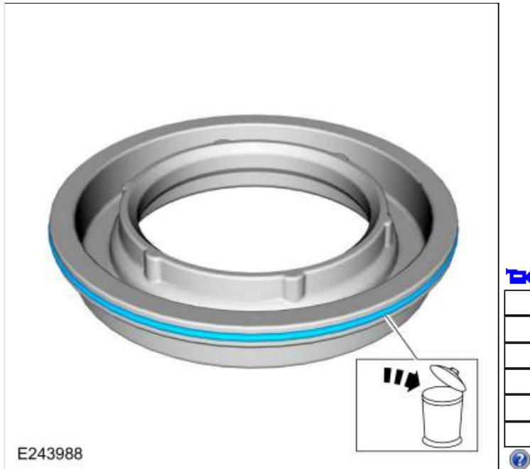
173. Remove the E clutch piston return spring.
