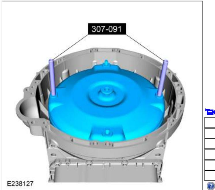
301. Install the special tool to hold the torque converter.
