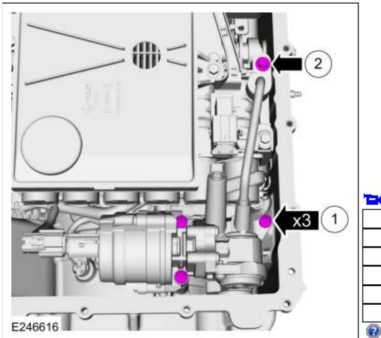
319. Connect the transmission fluid auxiliary pump electrical connector.
