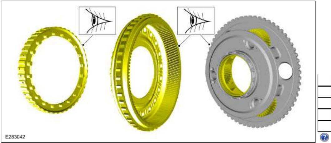
90. Install the ring gear No 1 snap ring.
