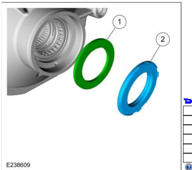
225. Using the special tool, install the output shaft seal.
