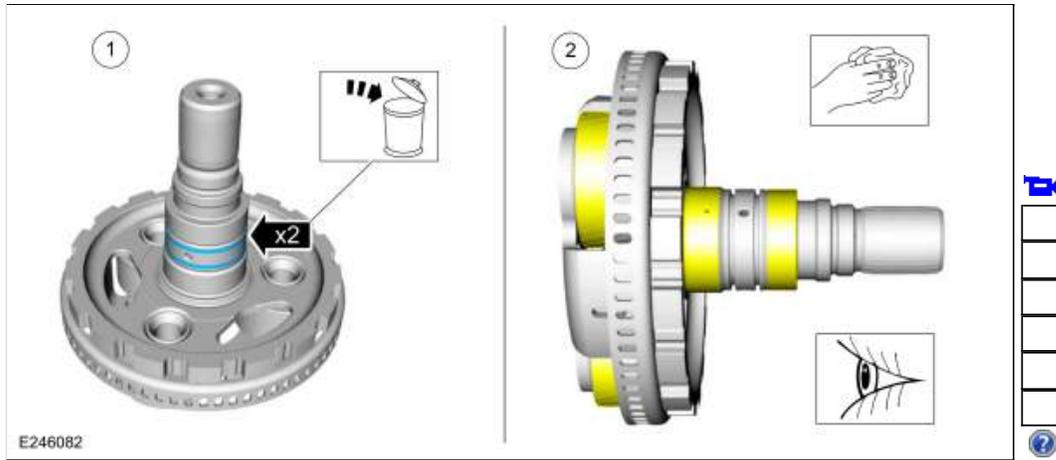
60. Using the special tools, remove and discard the output shaft seal.
