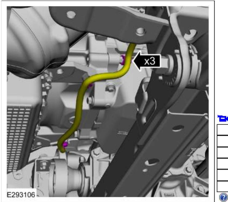
23. Inspect the transmission fluid cooler O-ring seals and install new O-ring seals if necessary. Lubricate the O-ring seals.
