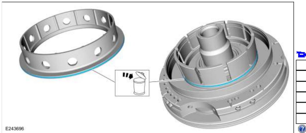
246. Remove and discard the front support-to-case seal.
