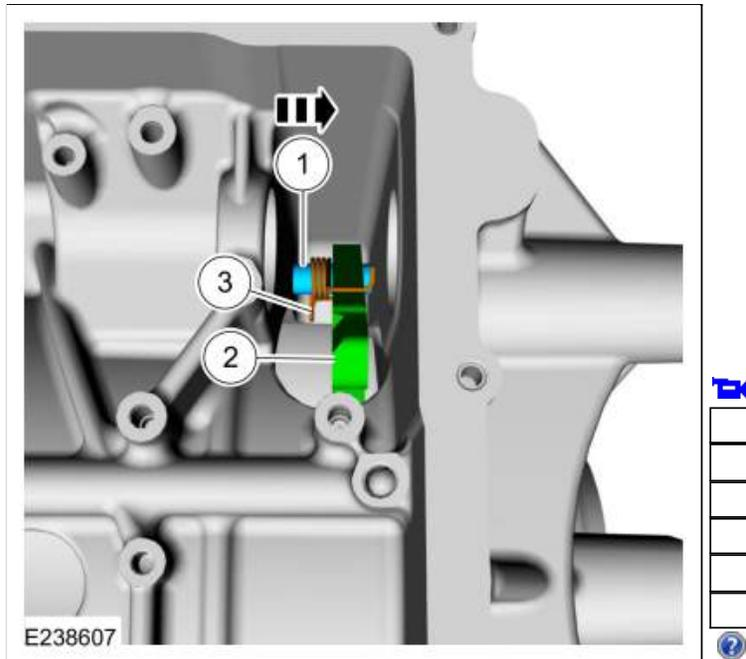
5. Remove the line pressure port and rear case plugs.
