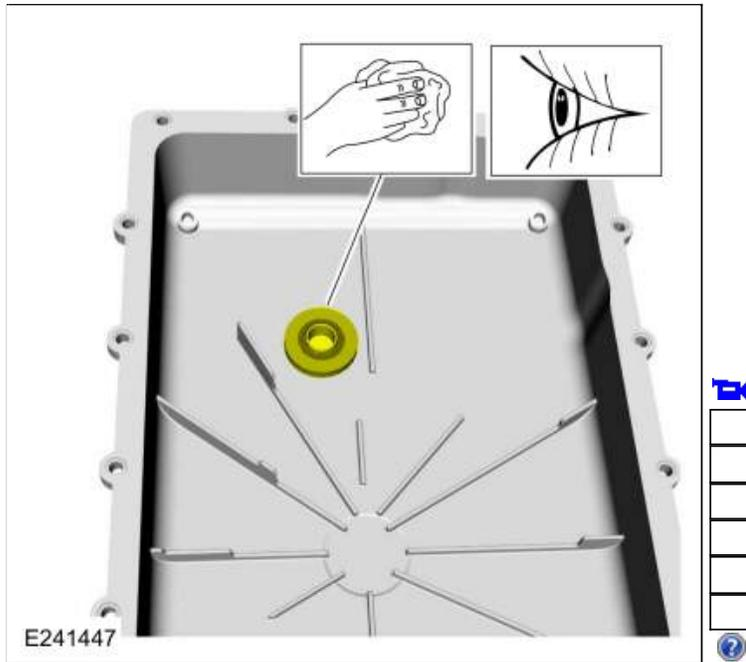
321. **NOTE:** *The transmission fluid pan gasket can be reused if not damaged.*
