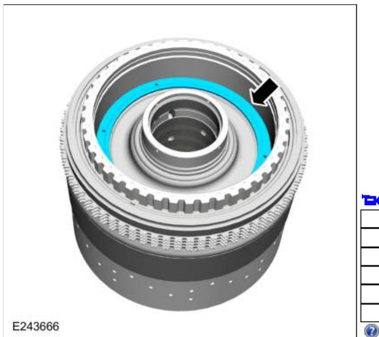
110. Using the special tools and a press, remove the D clutch balance dam retainer.
