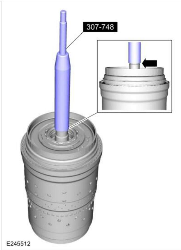
215. Install a new Teflon® seal on the special tool.
