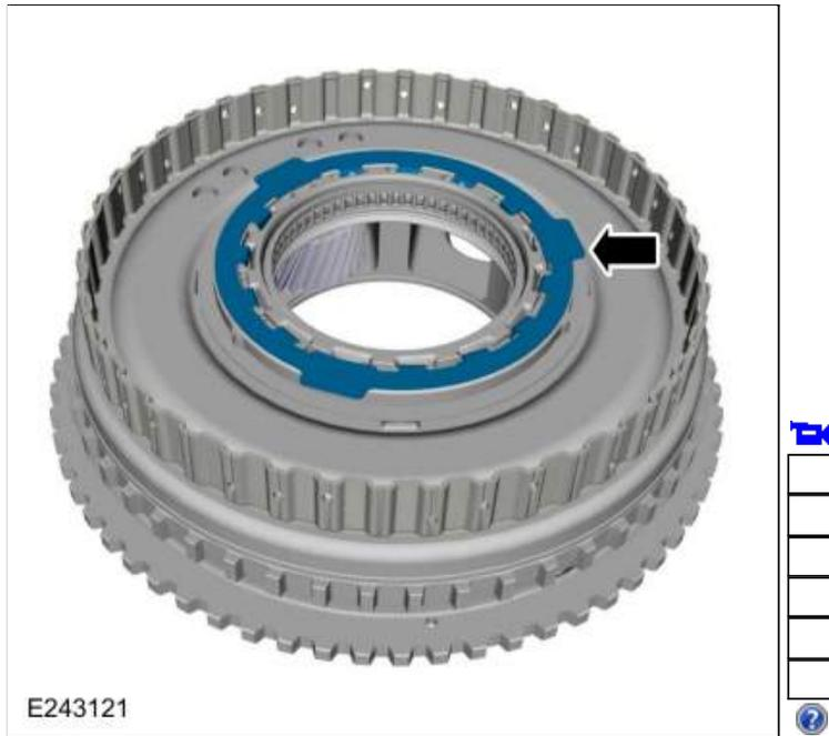
84. Rotate the No. 1 bearing support clockwise and remove the bearing support.
