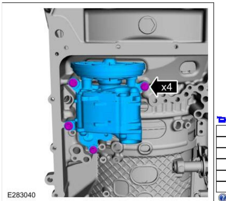
309. **NOTICE: Do not install a 71 mm length bolt in the location shown or the transmission clutch and planetary container will be damaged and result in transmission failure.**
