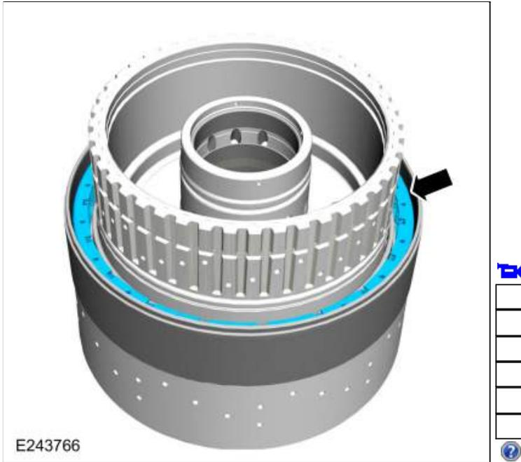
129. Install the new F clutch balance dam outer seal. Lubricate the seal with petroleum jelly.
