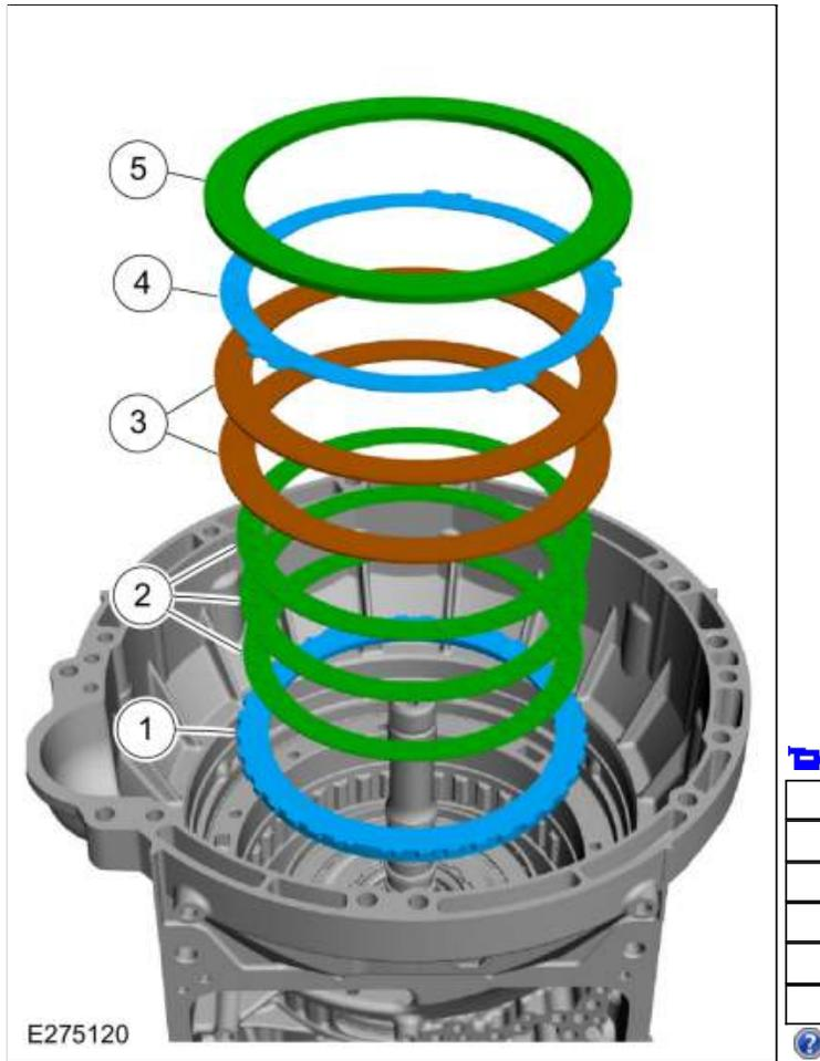
291. Using the special tools and a depth gauge, measure the distance from the top of the special tool to the top of the A clutch apply plate in 2 different places. Average the measurements. Record this as measurement A. Use Special Service Tool: [307-661 Gauge, End Play](#).
