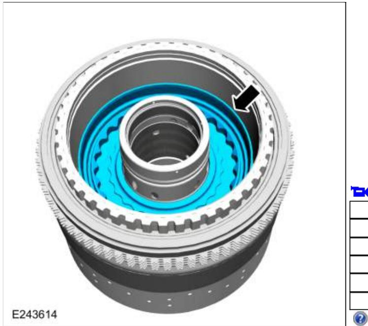
139. Install the D clutch piston return spring.
