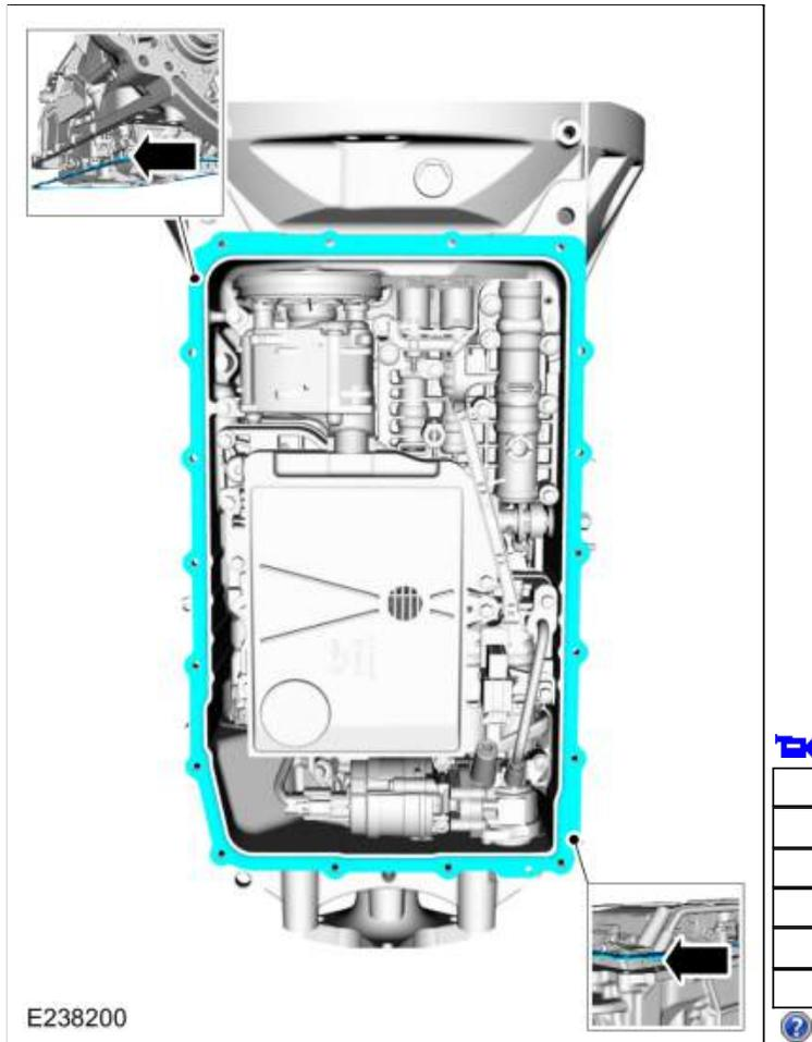
322. Install the transmission fluid pan and tighten the bolts in a crisscross pattern.
