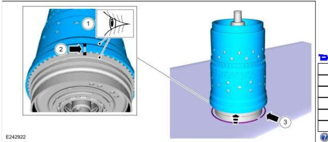
212. Using the special tool, install a new Teflon® seal in the groove on the input shaft. Use Special Service Tool: [307-653 Sizer, Input Shaft Teflon Seal](#).
