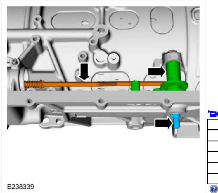
220. Install the new manual control shaft-to-TR sensor roll pin to the specified height.
