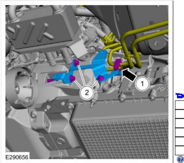
18. Remove the nut, bolt and the catalytic converter bracket.
