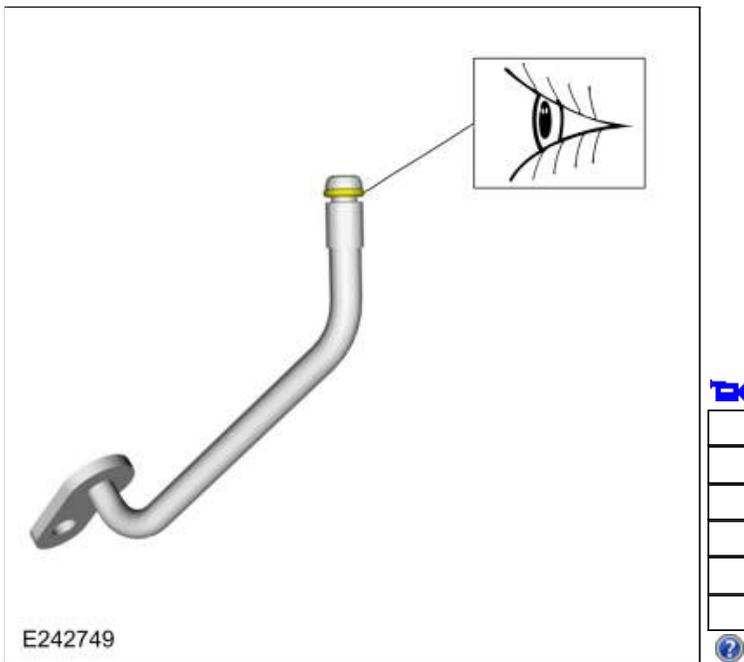
317. Install the transmission fluid auxiliary pump tube and loosely install the bolt.
