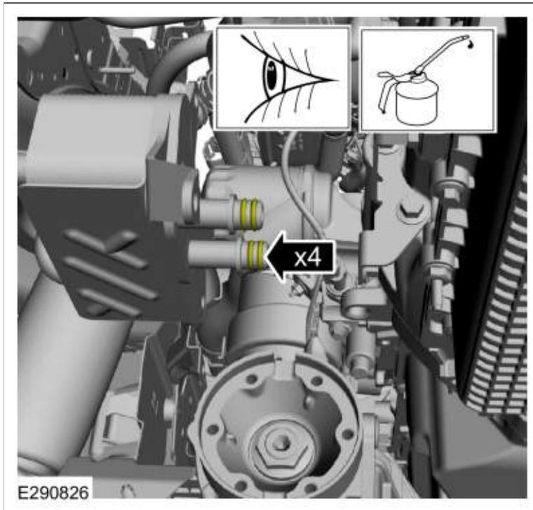
9. Install the transmission fluid cooler and loosely install the bolts.
