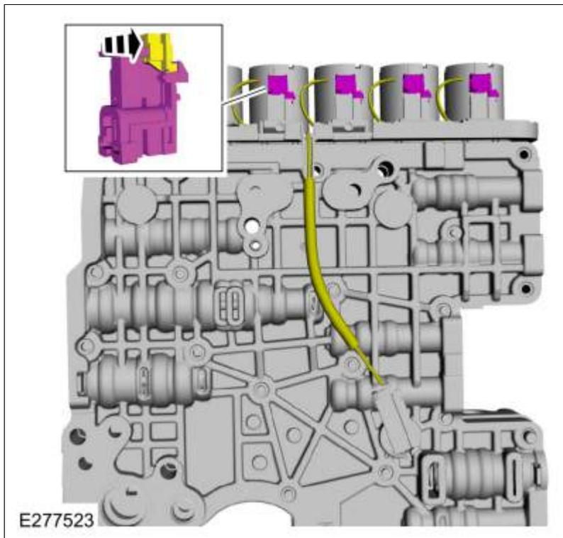
4. Install the shift solenoid retainer(s) with the flat side towards the solenoids.
