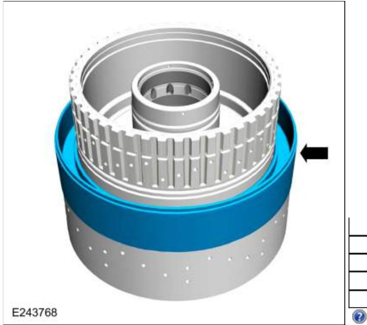
127. Install the new F clutch balance dam inner seal. Lubricate the seal with petroleum jelly.
