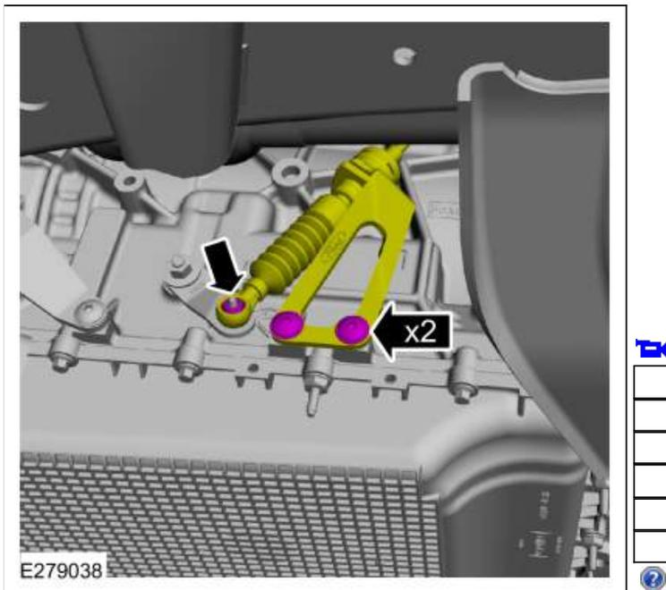
26. Install the heatshield and the retainers.
