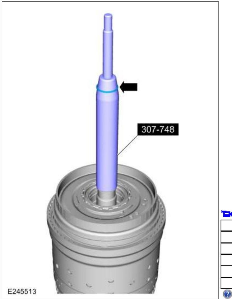
216. Using the top half of the special tool, slide the Teflon® seal into the groove. Remove the special tools and repeat the steps for the other 4 Teflon® seals.
