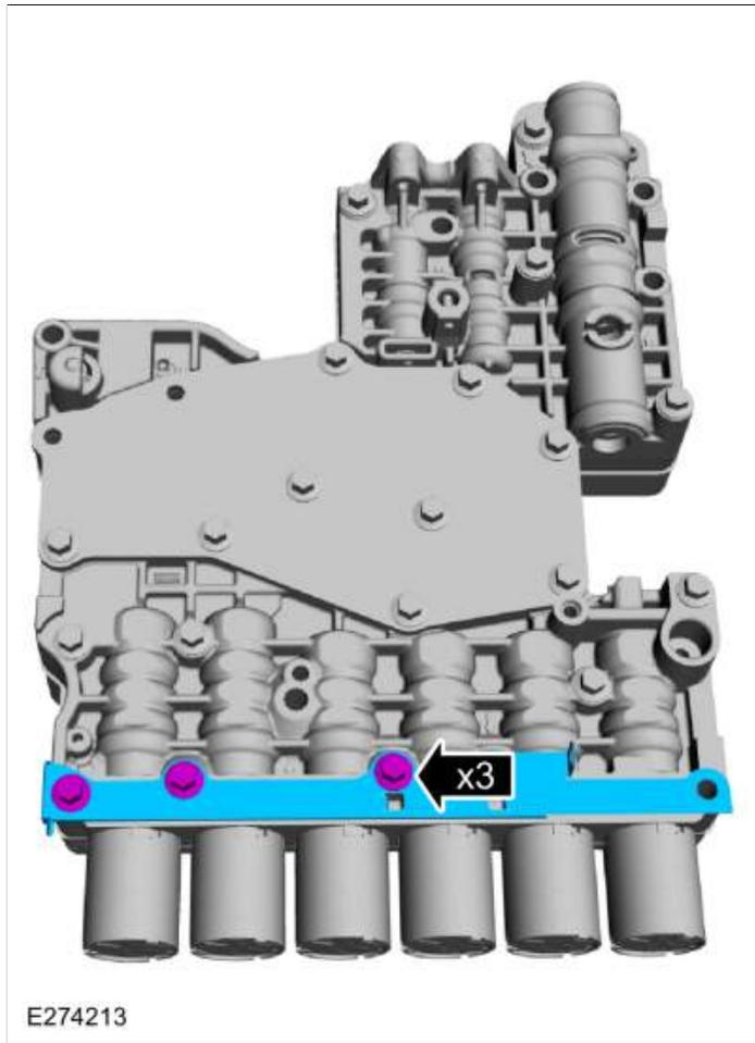
9. Remove the valve body bolts.
