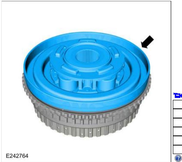
78. **NOTE:** It is not necessary to remove the fluid collector from the No. 2 planetary carrier.
