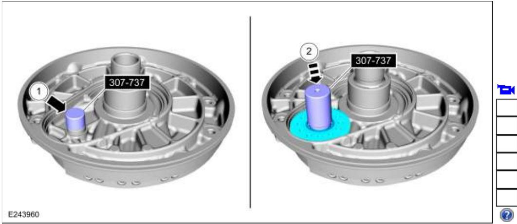
259. Install the transmission fluid pump drive gear with the flat side down.
