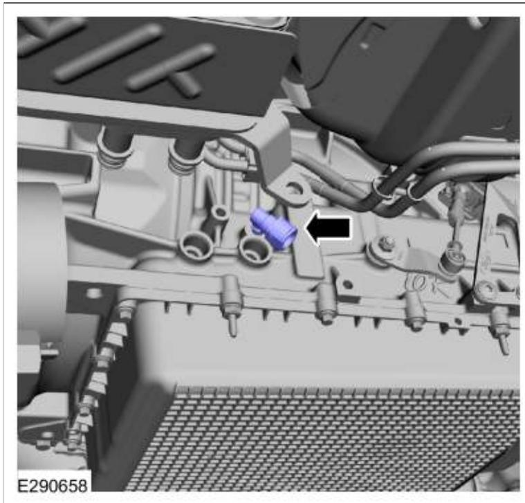
7. Install the transmission fluid cooler bracket and loosely install the bolts.
