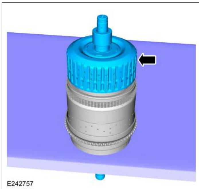
209. Install the (T8) thrust bearing.
