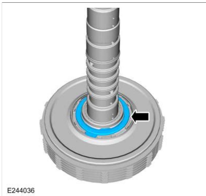
190. Install the (T7) thrust bearing onto the E clutch with the tab locators up. Snap the bearing into place.
