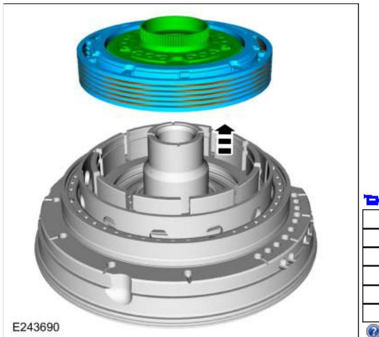
239. **NOTICE:** If replacing B clutch separating springs, all separating springs must be replaced as a matching set or damage can occur.
