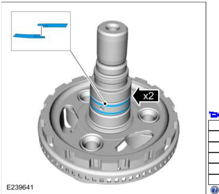
227. Install the (T10) thrust bearing on the output shaft.
