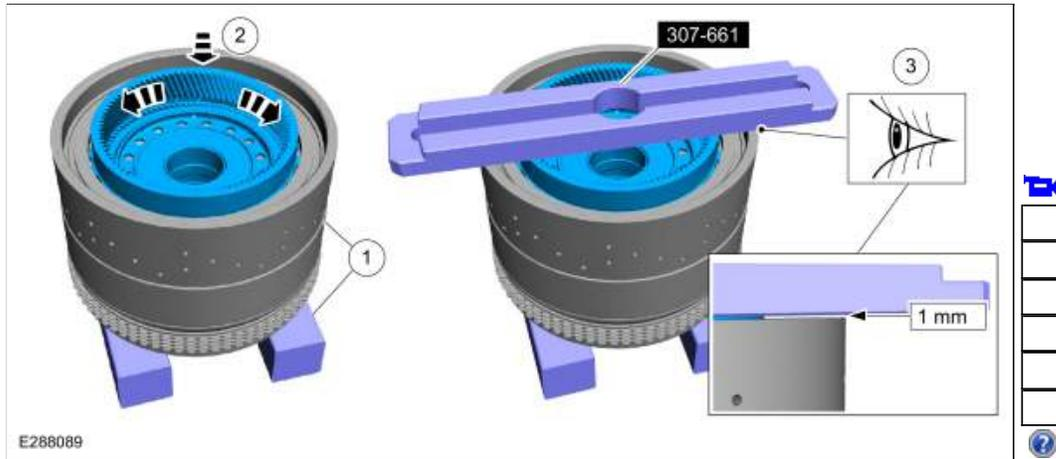
204. While holding the sun gear No. 3 shaft, flip the CDF clutch assembly over and install it on to the No. 2 planetary carrier.
