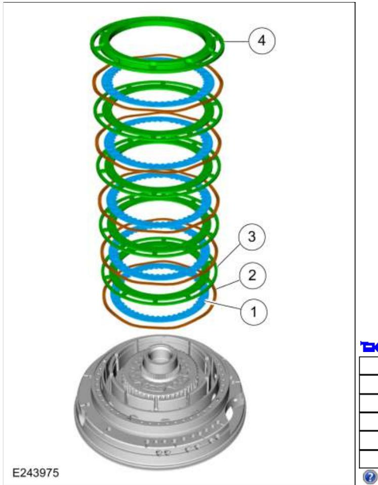
281. **NOTICE:** Be sure to align the top B clutch friction to the One-Way Clutch (OWC) hub or damage can occur.
