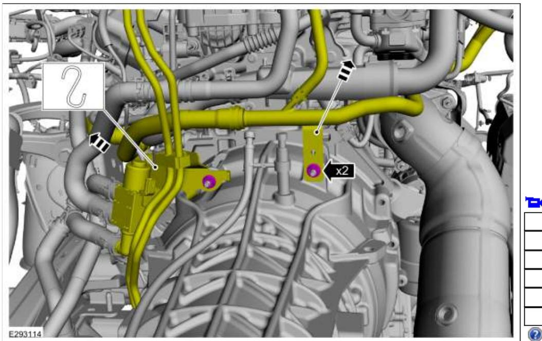
27. Remove the upper bellhousing bolt and studbolts.
