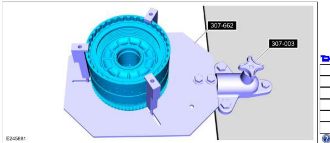
156. Using the special tool, measure the C clutch clearance. Position the plunger so it rests on the top surface of the pressure plate. Zero the dial indicator. Pull up on the pressure plate and measure and record the clutch clearance in 3 different places. Average the 3 recorded clutch clearance measurements and compare the measurement to the clutch clearance chart in specifications to determine the correct size snap ring. Install the correct C clutch snap ring.
