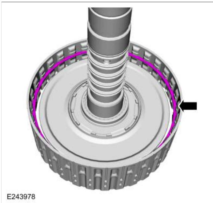
193. Install the No. 3 ring gear and the snap ring. Align the snap ring gap 180° from the bottom snap ring gap.
