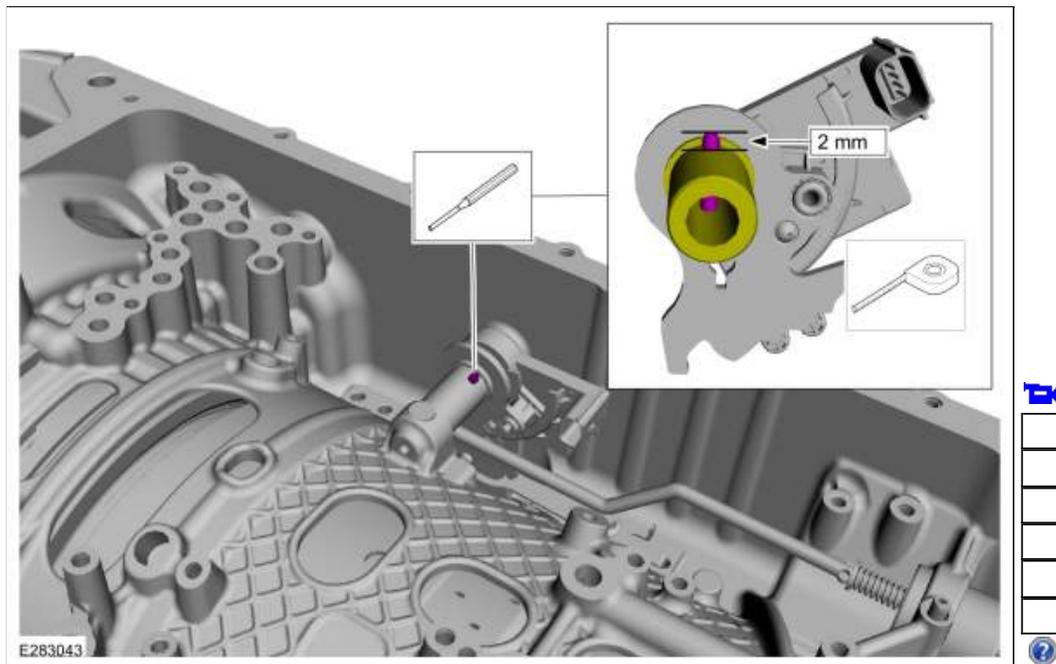
221. Install the manual shaft seal on the manual shaft. Using the special tool install the manual shaft seal in the transmission case.
