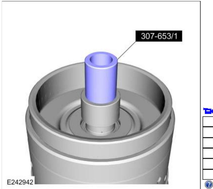
236. Using the special tools and a floor crane, install the clutch and planetary assembly.
