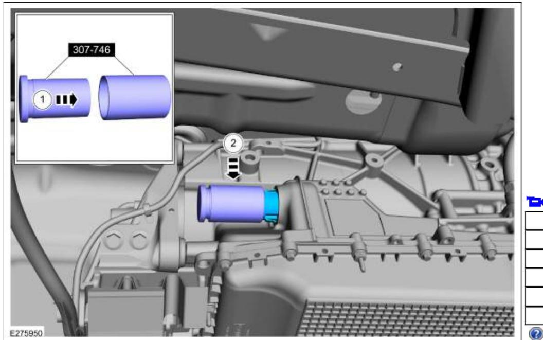
10. Using the special tool, disconnect the transmission internal wiring harness connector from the transmission case.
