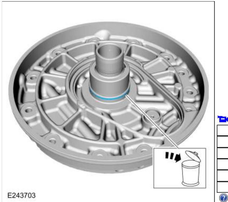
255. **NOTE:** If the One-Way Clutch (OWC) needs to be replaced the front support must be replaced.
