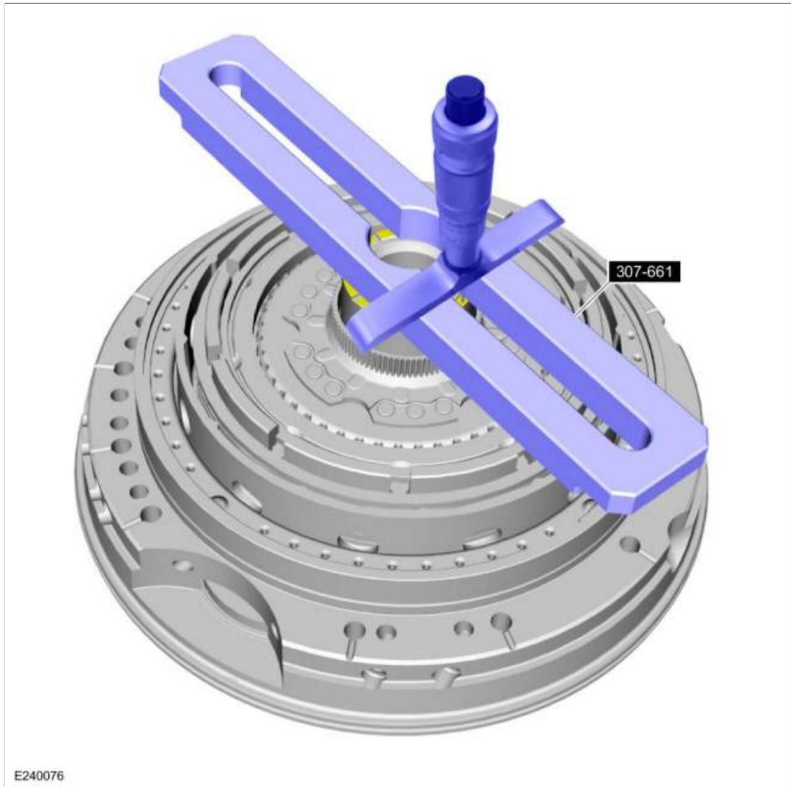
288. **NOTE:** Recorded measurements B and E are included to compensate for the difference in height of the special tool.
