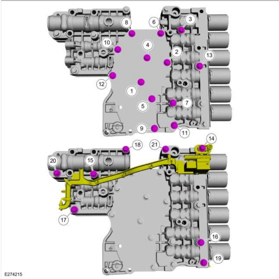
31. Push the internal wiring harness into the retainer.
