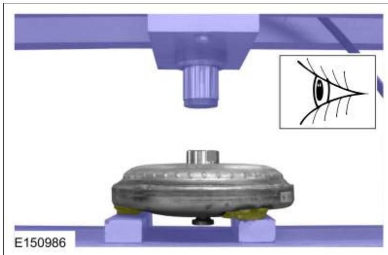
17. Install the torque converter leak tester (307-421) into the torque converter hub.
