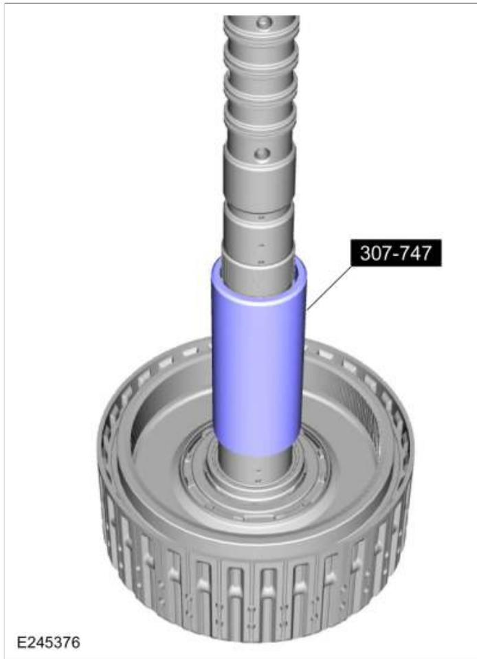
208. Install the E clutch and input shaft assembly.
