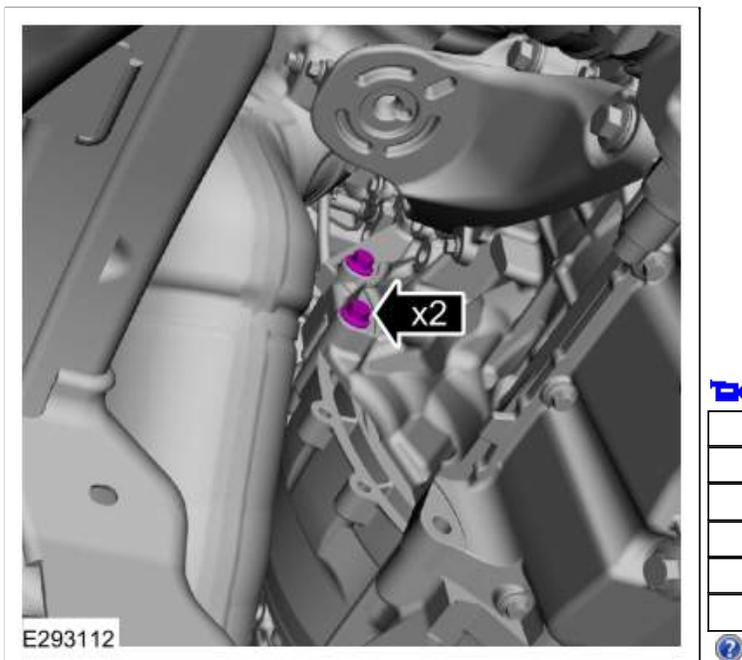
25. Remove the lower bellhousing bolts.
