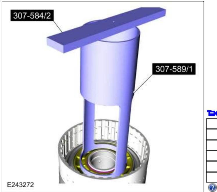
103. Remove the C clutch balance dam.
