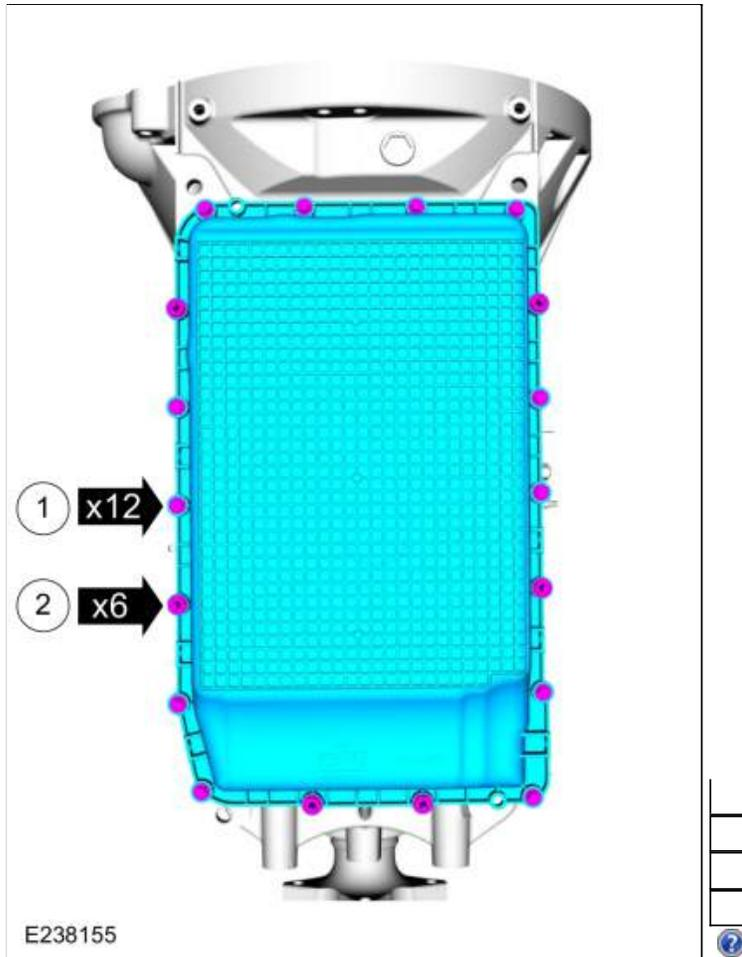
28. **NOTE:** *The transmission fluid pan gasket can be reused if not damaged.*
