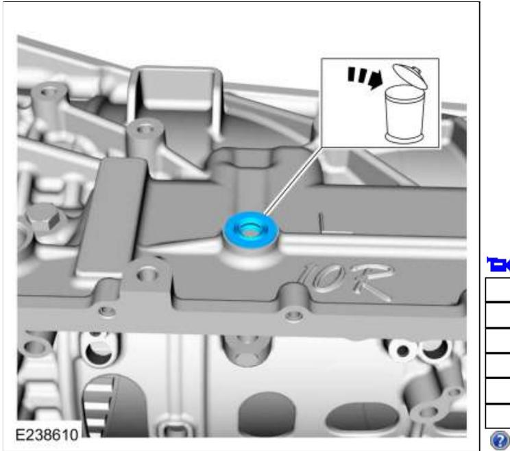
53. Remove the bolt and the TR sensor detent spring.
