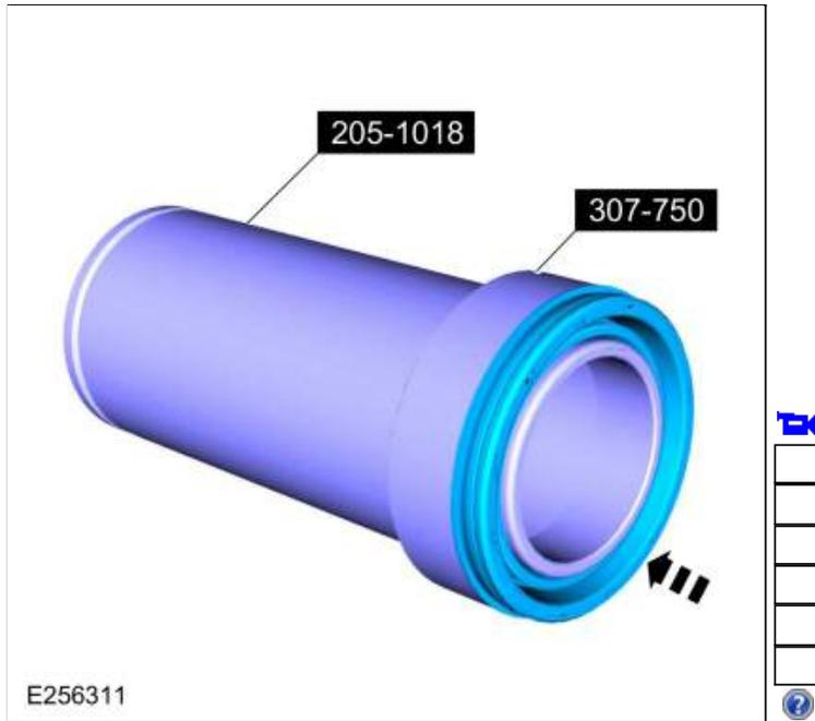
263. Using the special tools, install the new torque converter hub seal.
