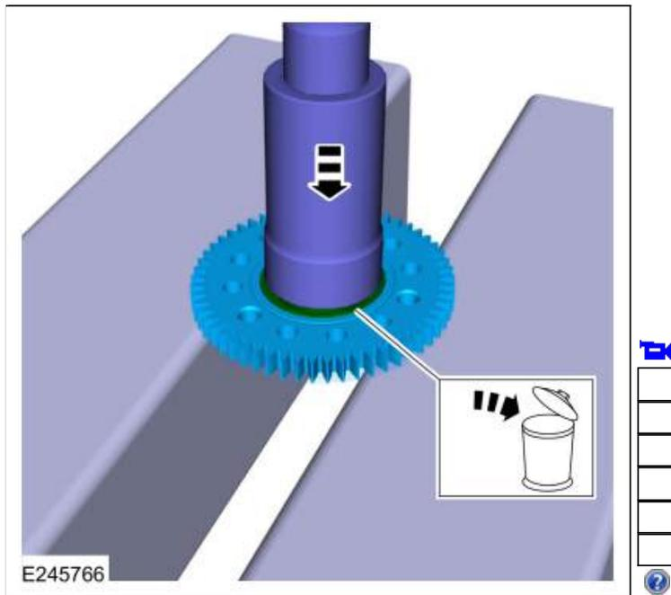
254. Remove and discard the stator support seal.
