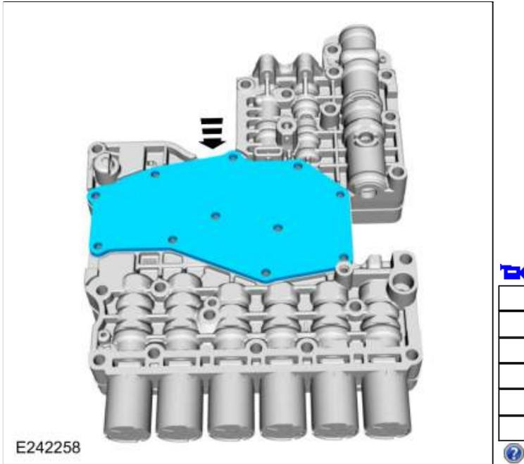
28. Loosely install the valve body bolts.
