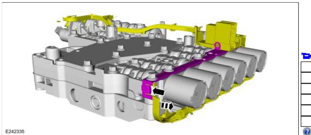
5. Remove the TFT sensor.
