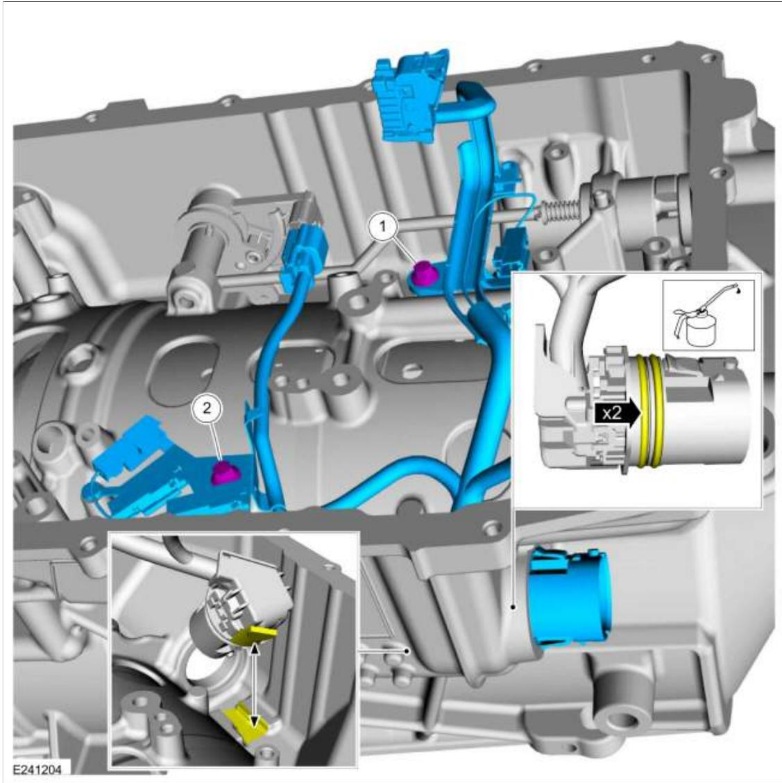
303. Support the opposite side of the TR sensor and connect the electrical connector.
