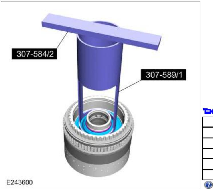
142. Install the D clutch apply ring.
