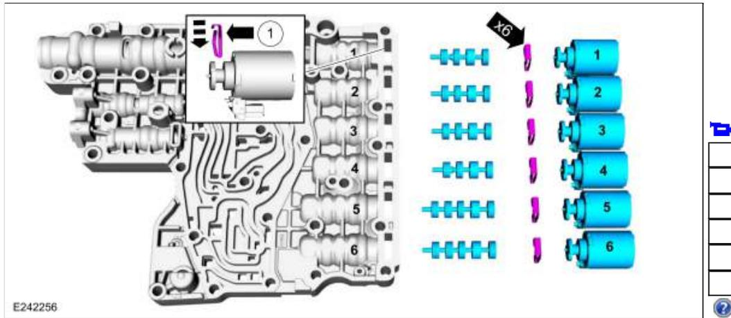
24. **NOTE:** *The orientation of the valves and springs.*
