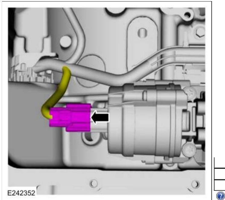
3. Support the opposite side of the TR sensor and connect the electrical connector.
