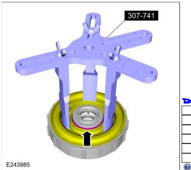
170. Pry the E clutch piston and balance dam upward and remove the piston and balance dam from the E clutch hub.
