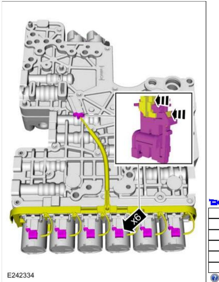
4. Release the retainer and remove the internal wiring harness assembly.
