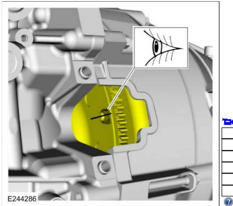
10. **NOTE:** Make sure the torque converter is fully seated in the transmission before aligning the transmission to the engine.
