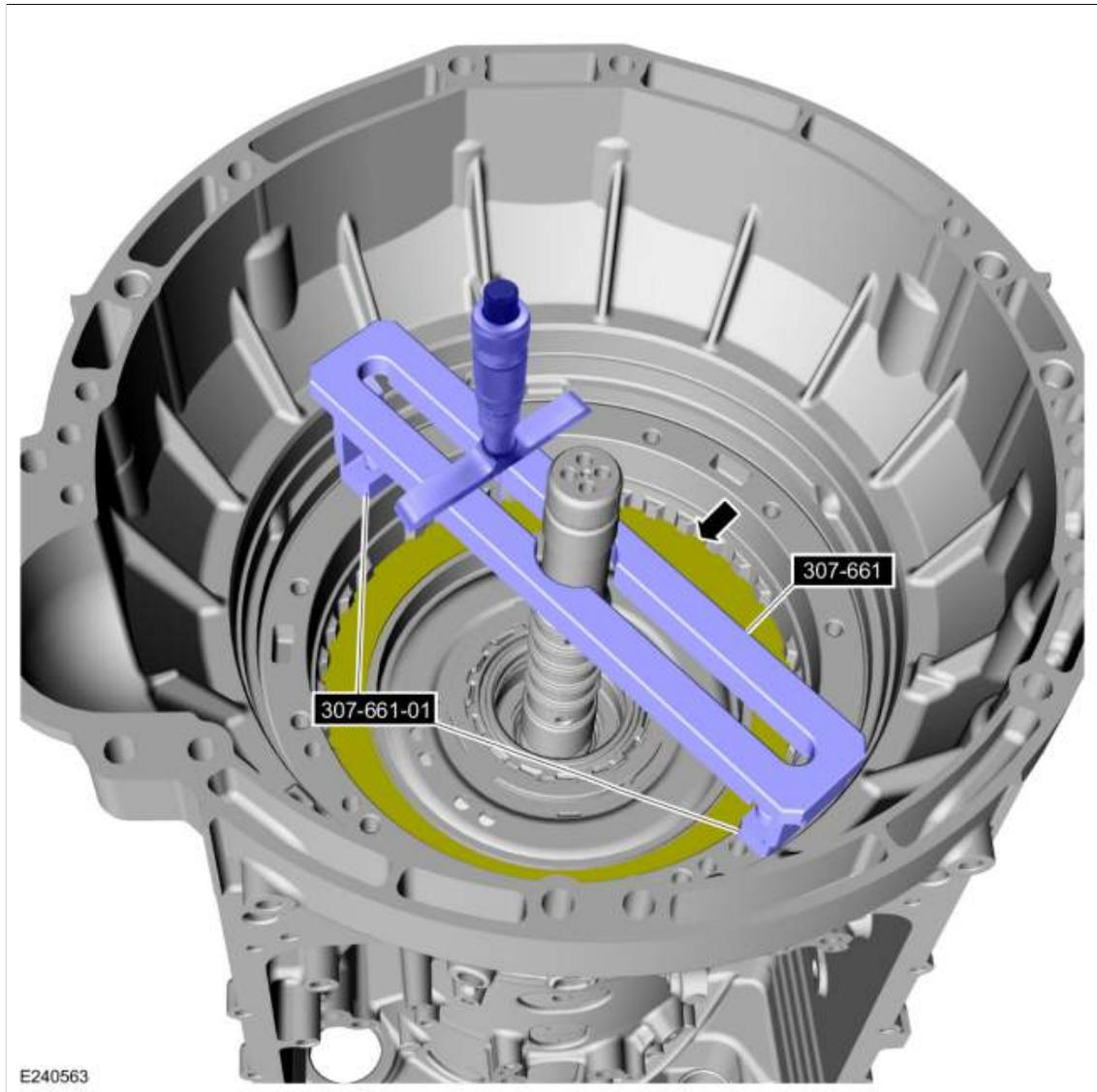
292. Using the special tools and a depth gauge, measure the distance from the top of the special tool to the front support mating surface in 2 different places. Average the measurements. Record this as measurement B.
