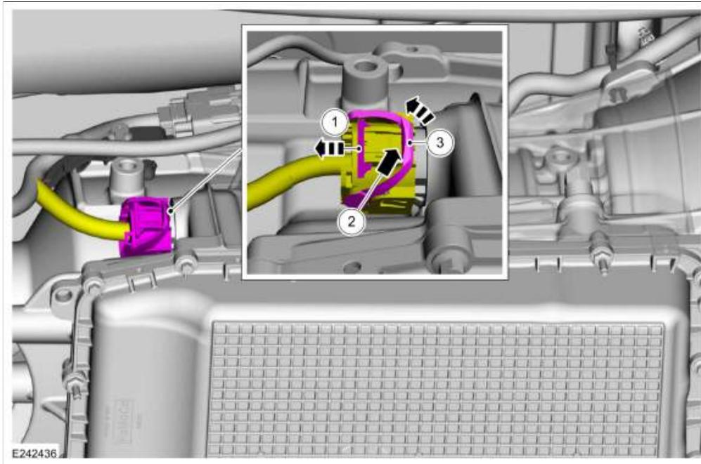
6. **NOTE:** To disconnect the electrical connectors, slide the plastic lock to the unlocked position. While pressing the plastic tab, disconnect the electrical connector.
