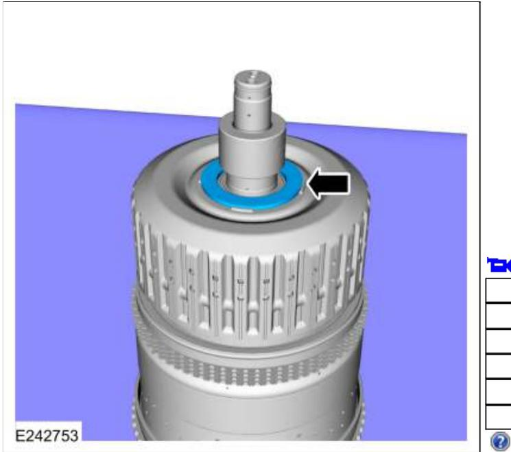
70. Remove the E clutch and input shaft assembly.
