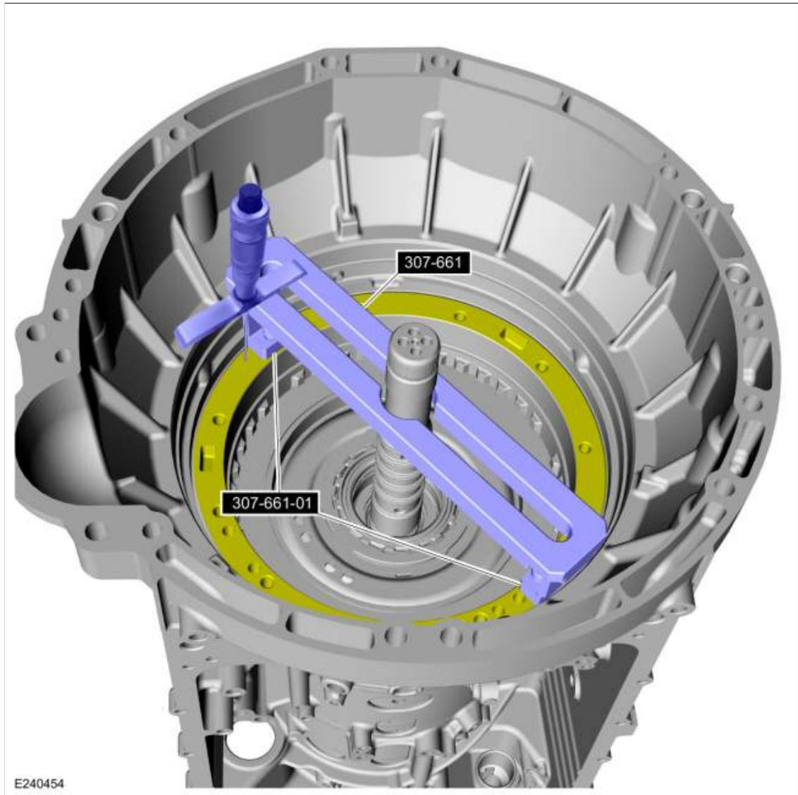
293. Using the special tool and a depth gauge, measure the distance from the top of the special tool to the transmission deck mating surface in 2 different places. Average the measurements. Record this as measurement D. Use Special Service Tool: [307-661 Gauge, End Play](#).
