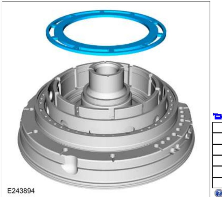
272. **NOTE:** The B clutch separating springs are not installed when measuring the B clutch clearance.
