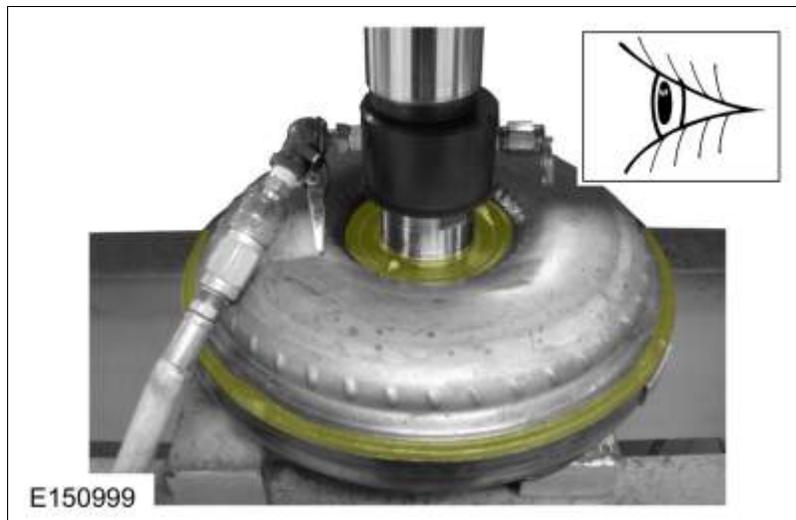
21. Inspect for leaks at the stud or mounting pad and balance weight welds. A soap bubble solution can be applied around those areas to aid in the diagnosis. If any leaks are present, install a new torque converter.
