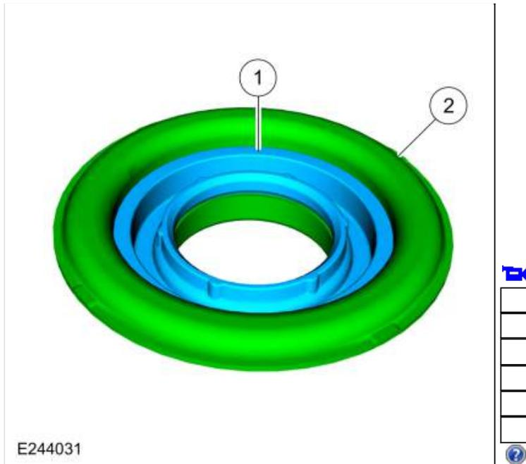
182. Lubricate the new E clutch piston seal with petroleum jelly.
