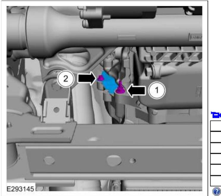
14. Install the transmission fluid cooler bracket.
