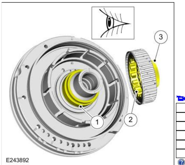
256. Install the new stator support seal on the front support. Lubricate the stator support seal with petroleum jelly.
