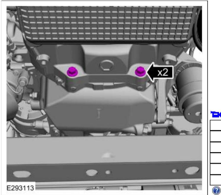
26. Remove the nuts and position aside the brackets.
