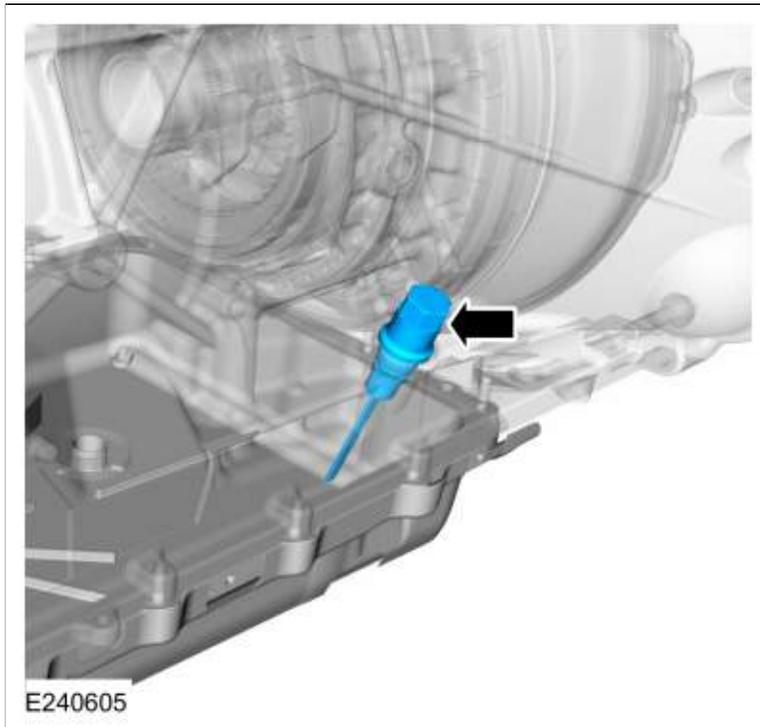
5. **NOTE:** The transmission fluid level indicator uses 1 through 6 to indicate the fluid level. The different numbers are for different vehicle models. Use the area between 4 and 5 when checking the transmission fluid level. The correct transmission fluid level is between 4 and 5 on the transmission fluid level indicator.
