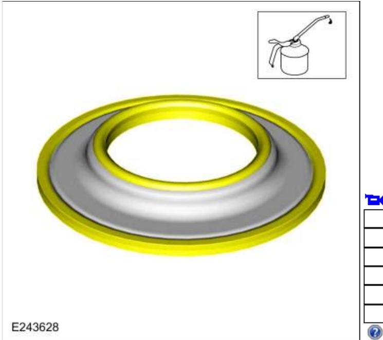
141. Using the special tools and a press, Install the D clutch balance dam and install the retainer.
