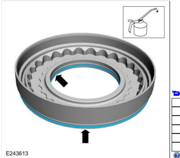
138. Install the D clutch piston.
