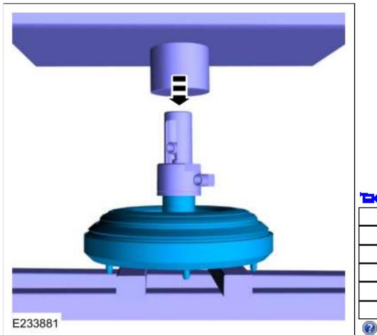
15. Connect the flush machine to the main hub.
