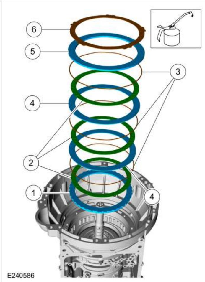
297. Lubricate the transmission case-to-front support sealing surface, the Teflon seals and the front support O-ring with petroleum jelly.
