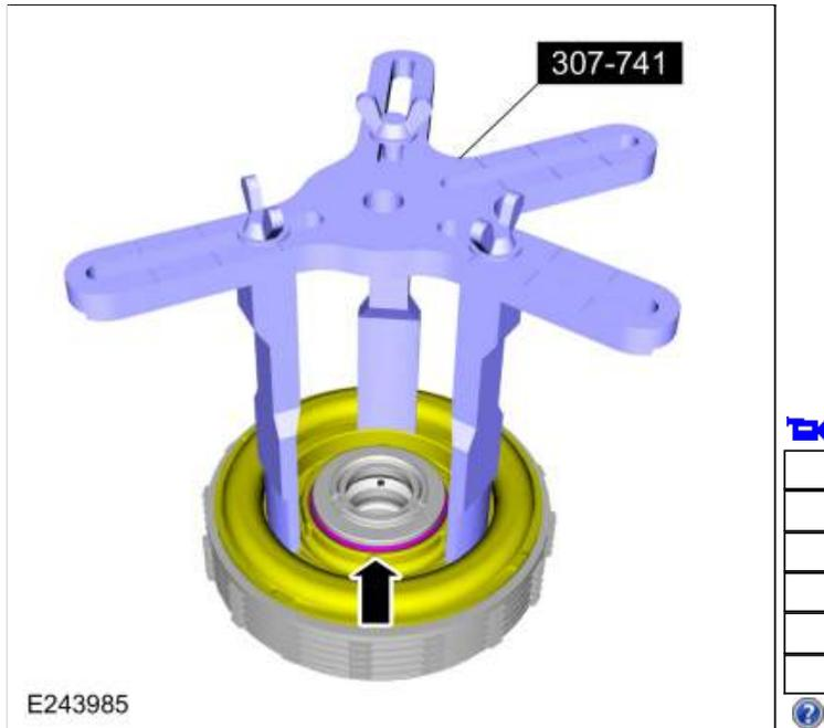
185. Assemble the special tools and position the E clutch assembly on the special tool.
