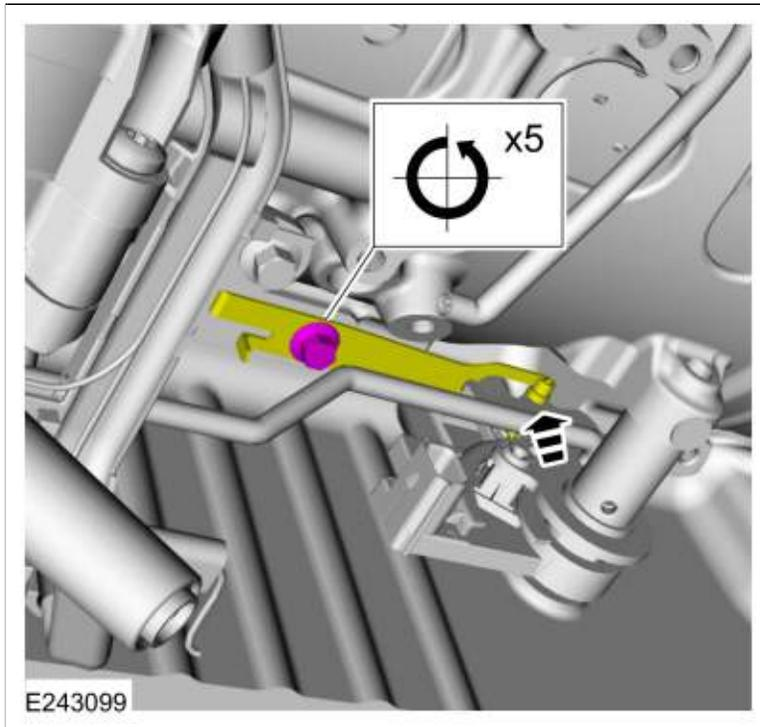
6. Remove the manual shaft and selector lever from the TR sensor.
