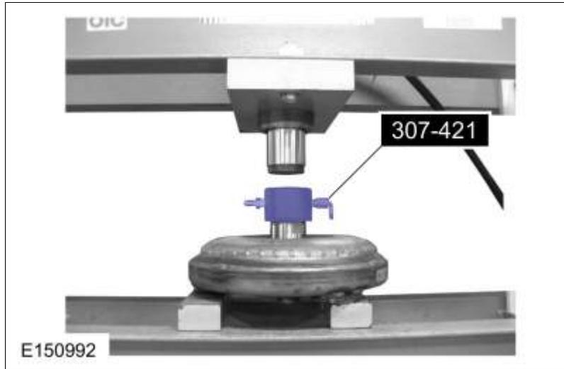
18. Secure the press. Apply enough force from the press to seal the torque converter leak tester (307-421) into the torque converter hub.
