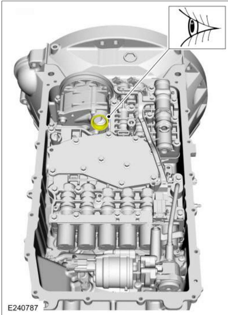
2. Lubricate the transmission fluid filter seal with automatic transmission fluid.
