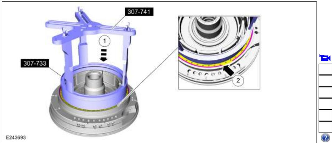
243. Remove the A clutch piston return spring.
