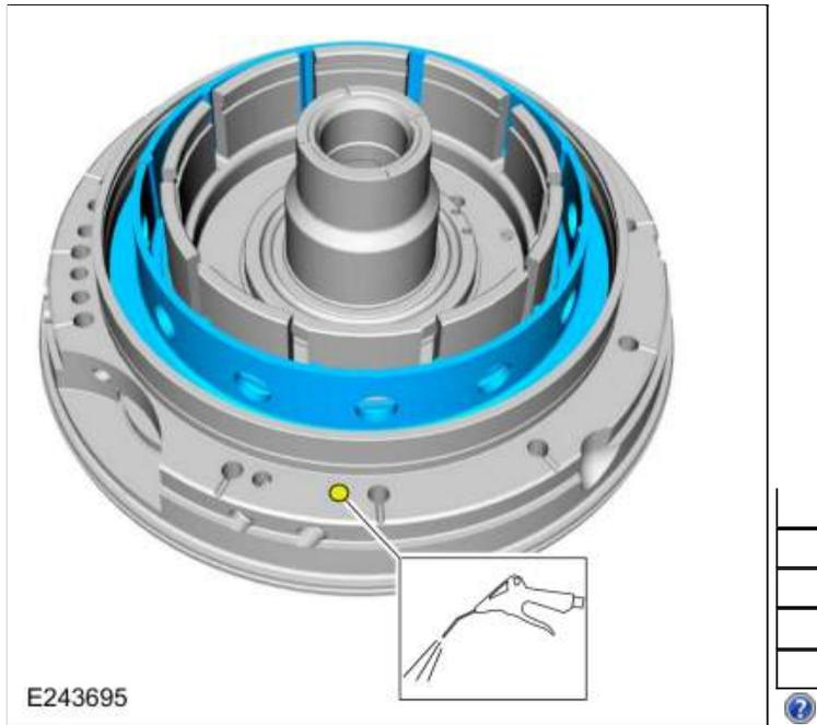
245. Remove and discard the A clutch piston outer seal and the A clutch piston inner seal.
