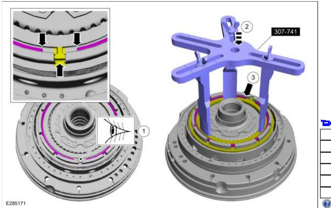
238. **NOTICE:** Remove the One-Way Clutch (OWC) and B clutch assembly gently, as the One-Way Clutch (OWC) rollers and springs could become dislodged.
