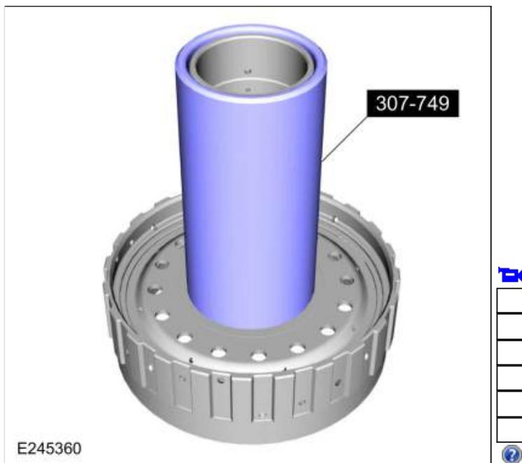
203. Install the No. 3 sun gear shaft into the CDF clutch assembly.
