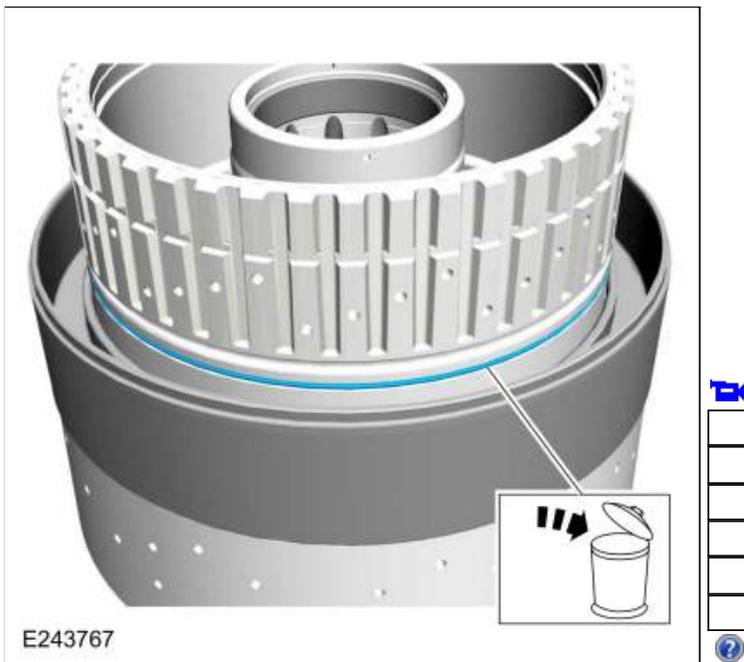
122. Remove the F clutch piston.
