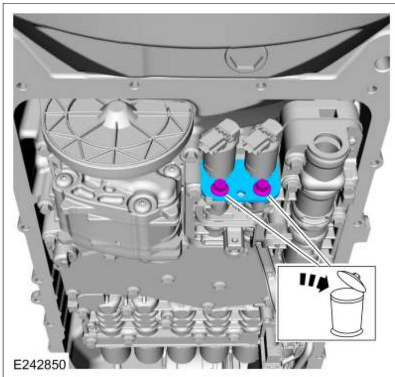
4. Remove the solenoid(s) from the main control valve body.
