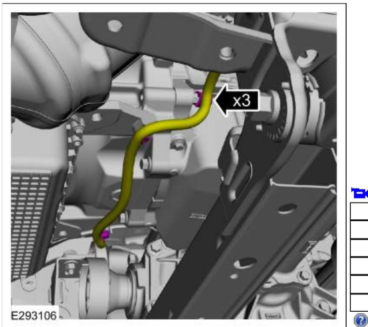
20. Remove the bolt, inspection shield and the oil pan bolt.
