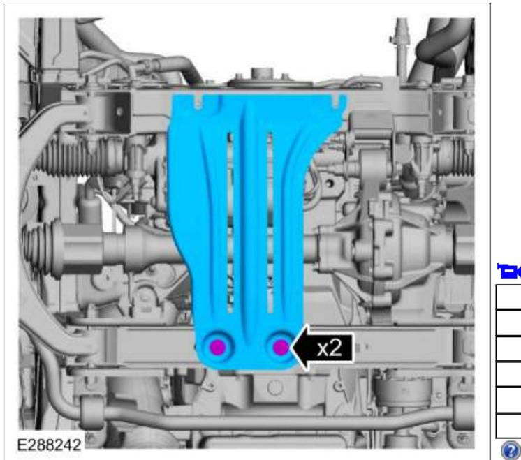
4. Remove the starter motor assembly.
