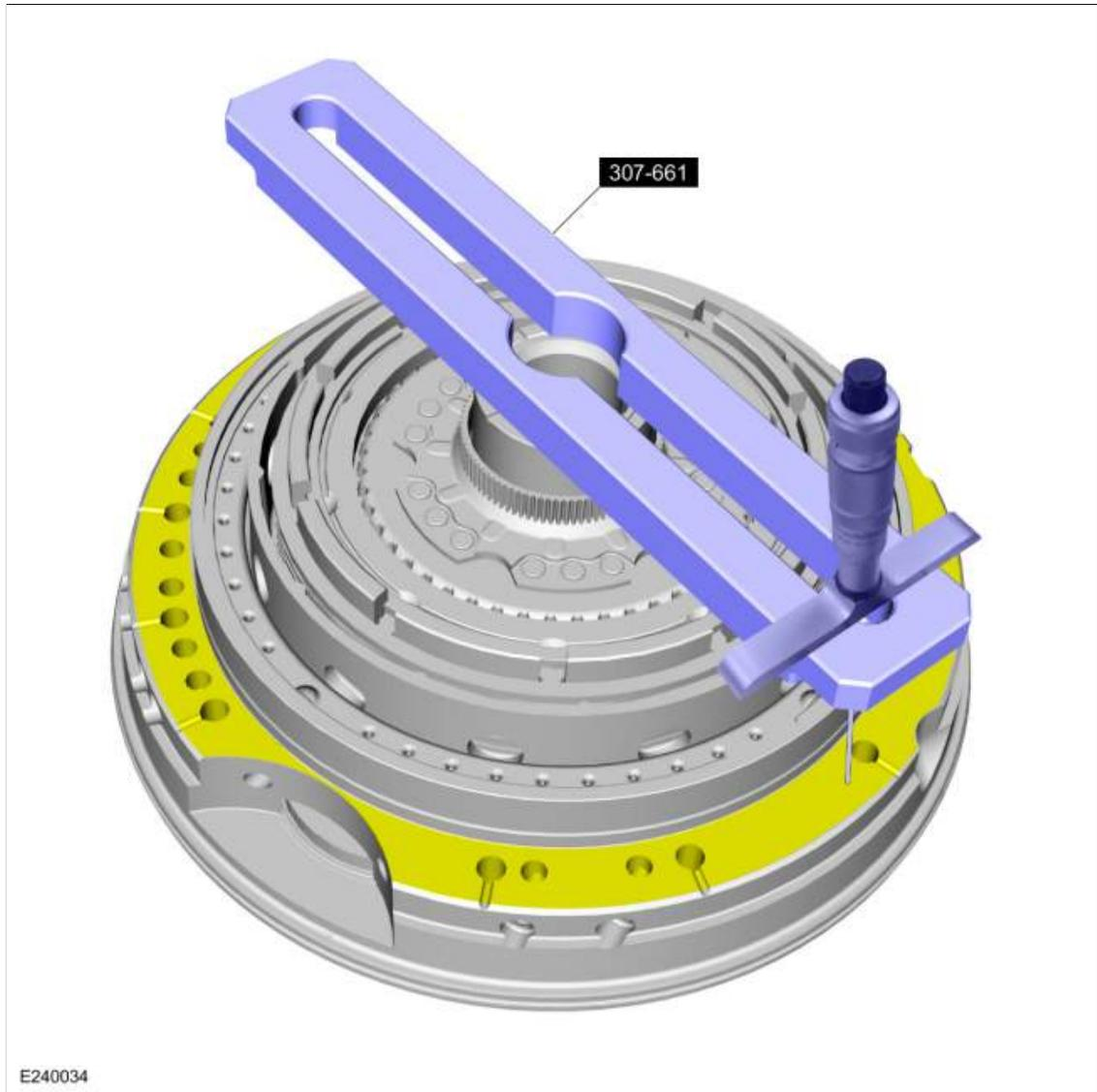
294. Using the special tool and a depth gauge, measure the distance from the top of the special tool to the A clutch piston surface in 2 different places. Average the measurements. Record this as measurement E.
