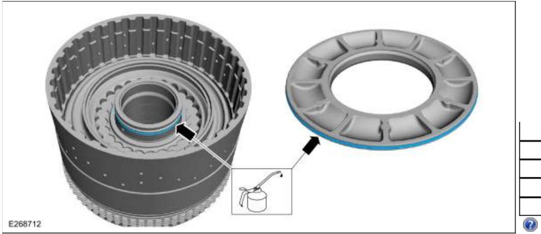
150. Install the C clutch piston return spring.
