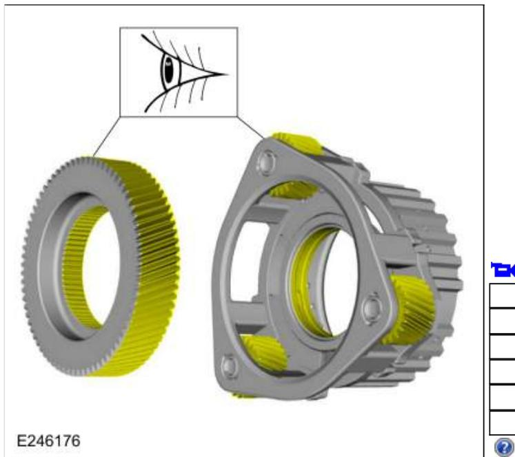
73. Remove the CDF clutch assembly from the planetary carrier assembly.
