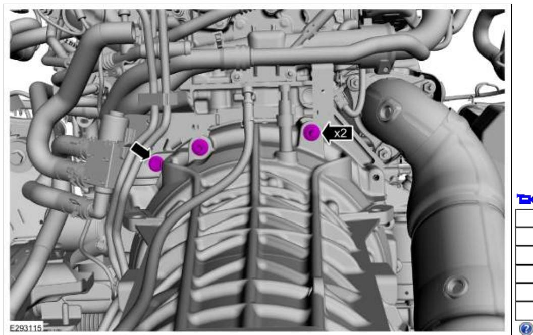
11. Install the lower bellhousing bolts.
