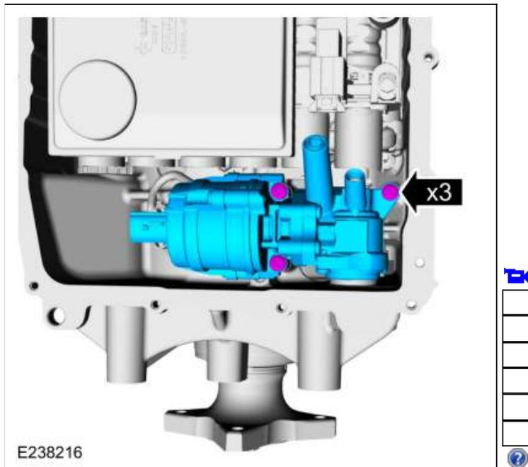
315. Install the new transmission fluid auxiliary pump tube seal.
