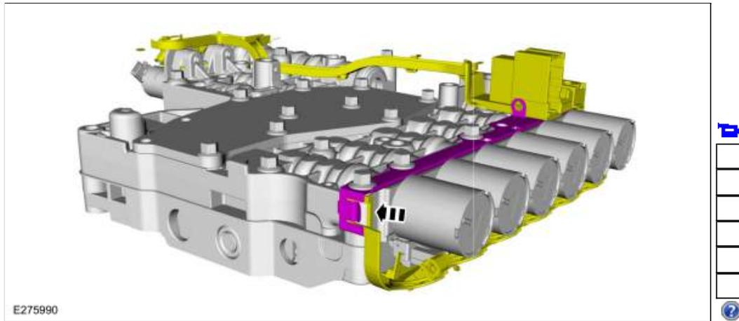
7. Connect the internal wiring harness electrical connectors.
