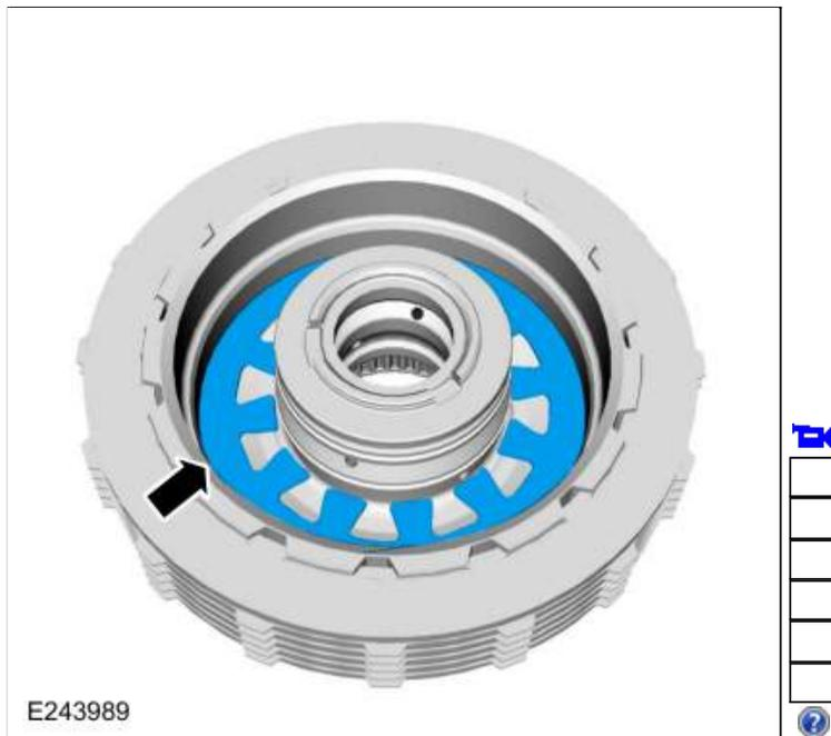
180. Install a new E clutch balance dam outer seal. Lubricate the seal with petroleum jelly.
