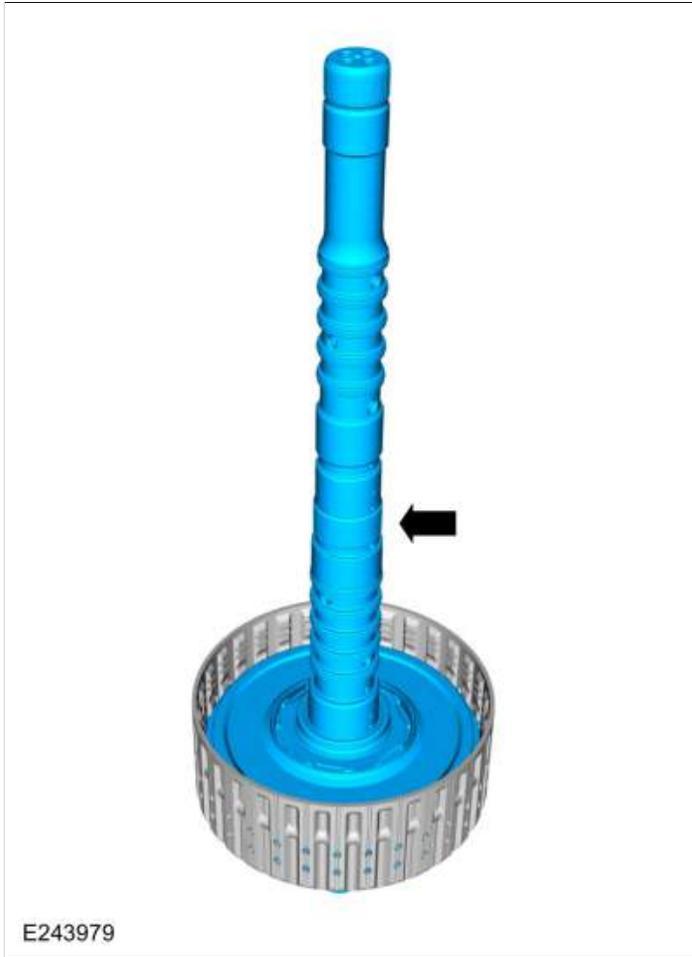
192. Install the lower rear No. 3 ring gear snap ring.
