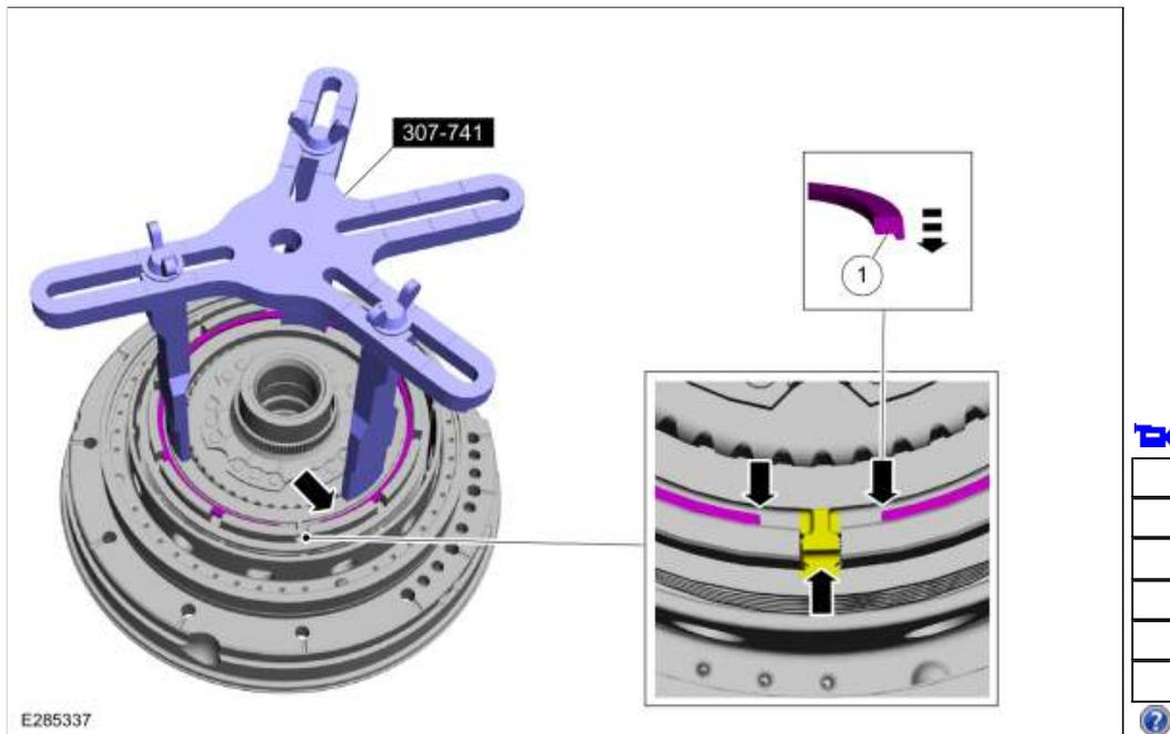
283. Install the (T3) thrust bearing.
