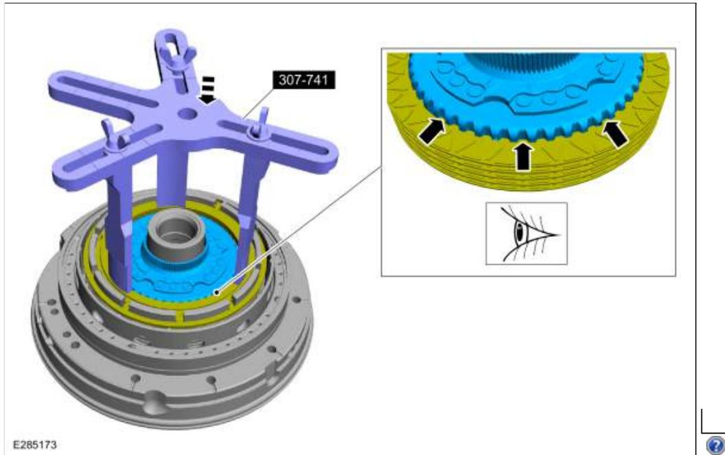
282. Install the B clutch snap ring in the correct location with the grooved side down.
