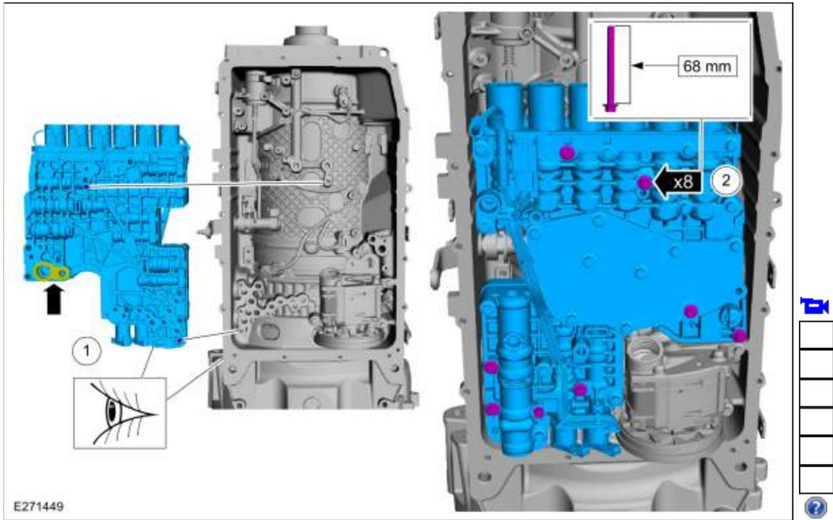
3. Tighten the bolts in the sequence shown.
