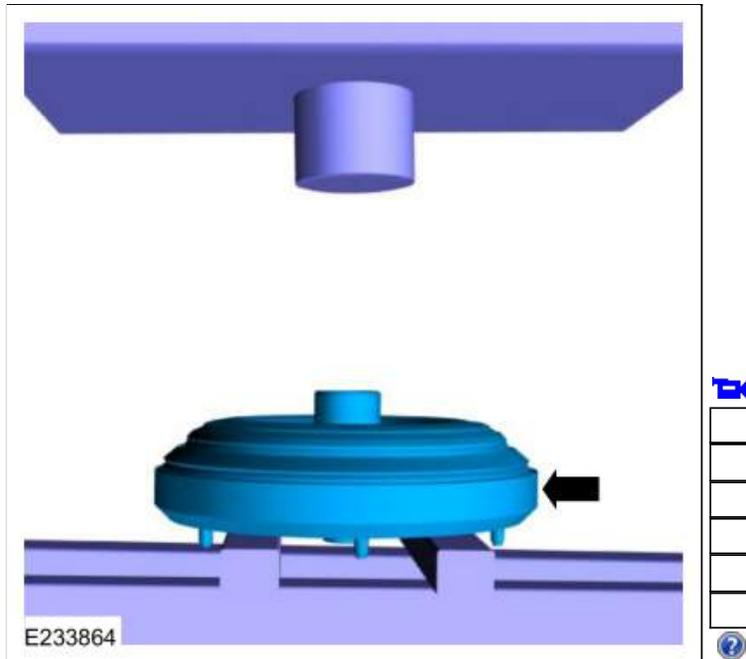
12. Using the special tools, assemble the correct turbine shaft simulator to the torque converter flush main hub and place it on the torque converter hub.
