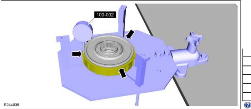
187. Install the new input shaft D-ring seals.
