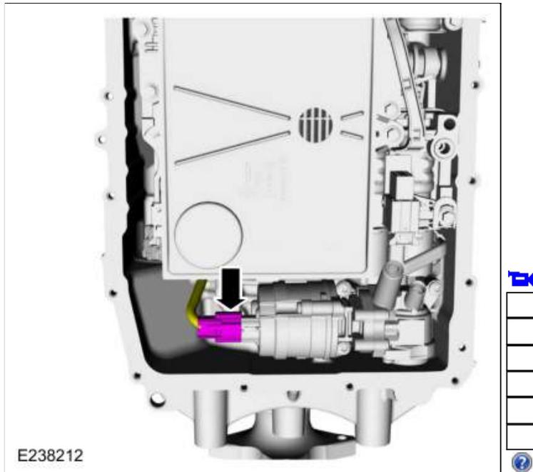
32. Remove the bolts and the transmission fluid auxiliary pump.
