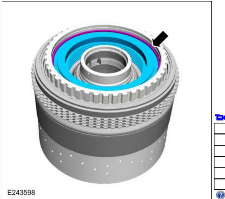
109. Remove the D clutch apply ring.
