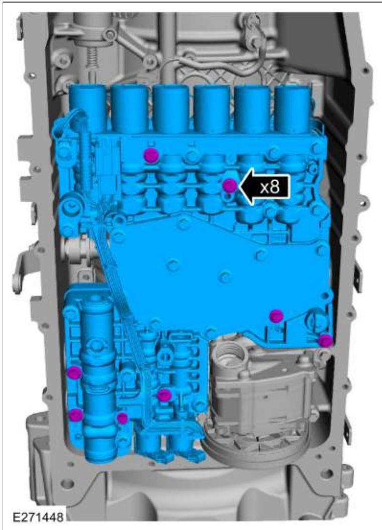
4. Remove the main control assembly to transmission fluid pump seal.
