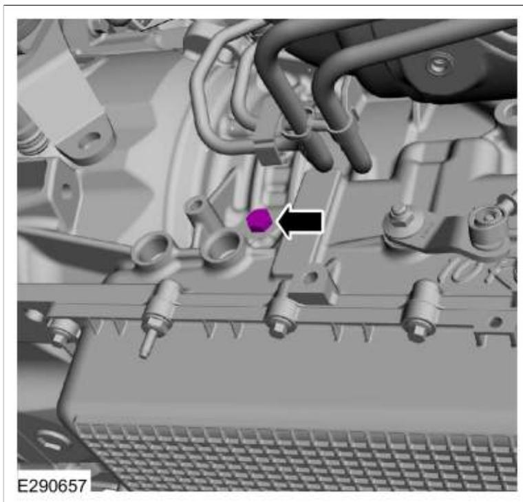
6. **NOTICE:** The line pressure tap is an M10 X 1.00 thread. Do not use a National Pipe Thread (NPT) fitting when installing a pressure gauge. If a NPT fitting is used, damage to the transmission case will occur.
