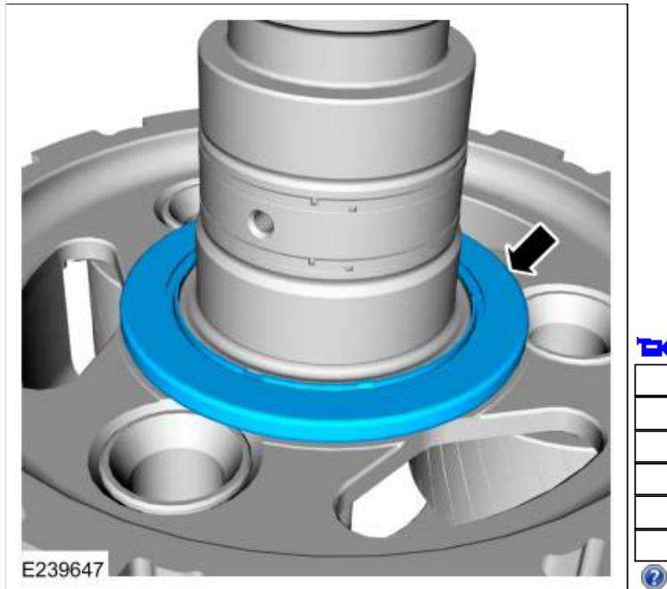
228. Rotate the manual lever to N. Install the output shaft and planetary carrier assembly No. 4.
