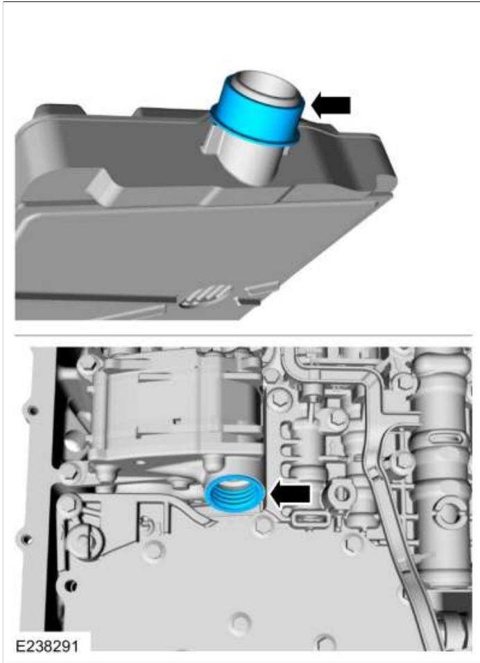
35. Disconnect the main control main electrical connector.
