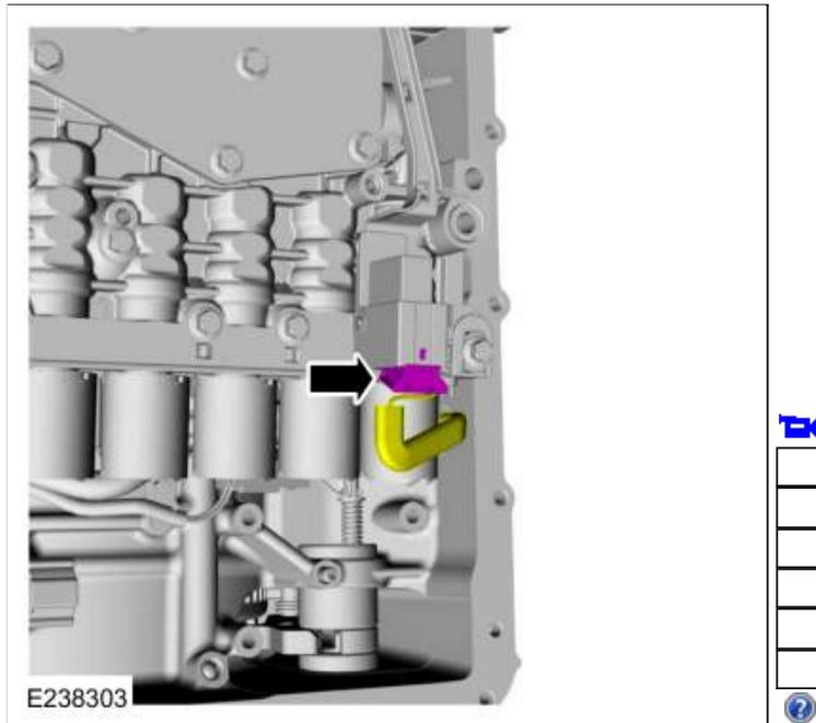
312. Install the filter seal in the pump.
