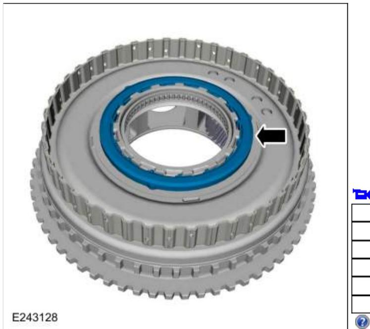
85. Remove the No. 1 ring gear bearing.
