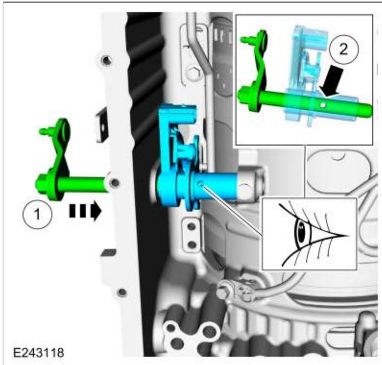
3. Install the new manual shaft-to-TR sensor roll pin to the specified height.
