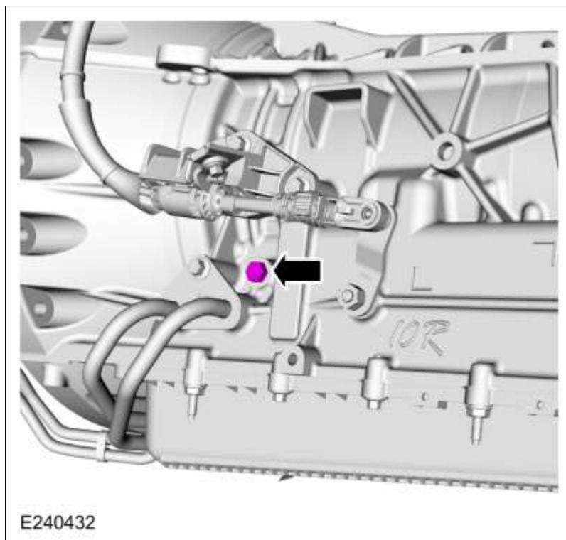
1. **NOTE:** The line pressure tap is an M10 X 1.00 thread. Do not use a National Pipe Thread (NPT) fitting when installing a pressure gauge. If a NPT fitting is used, damage to the transmission case will occur.
