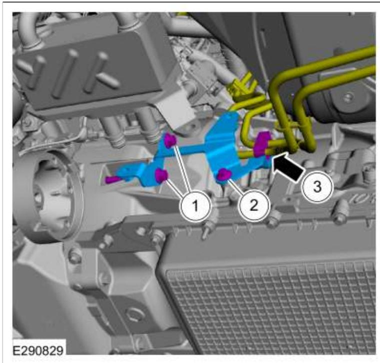
15. Install the transmission fluid cooler and the bolts.
