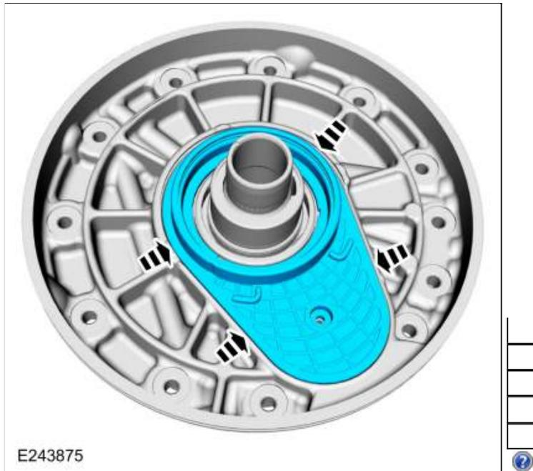
261. **NOTE:** The front support cover snap ring ends are located in the cover alignment features.
