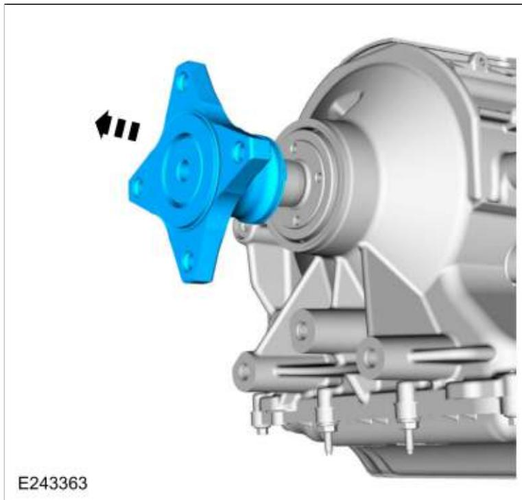
6. Using the special tool, remove and discard the output shaft nut (7085).
