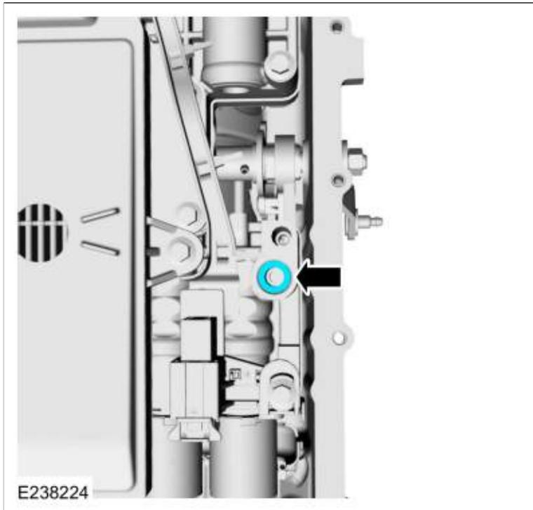
3. Inspect the transmission fluid auxiliary pump tube O-ring.
