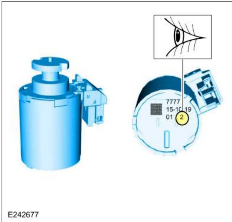
8. Install the solenoid(s) in the main control valve body in the correct port(s) as marked during removal.
