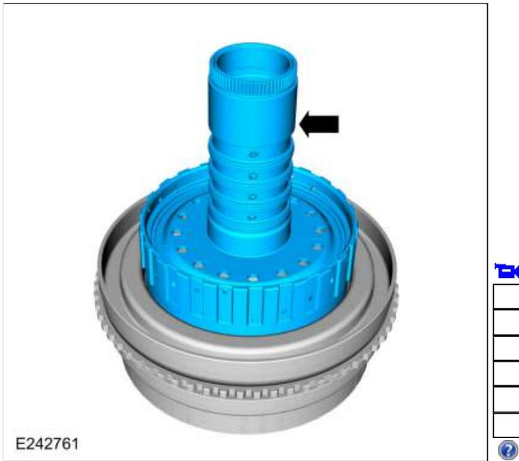
75. Inspect the No. 3 sun gear shaft and No. 2 ring gear assembly.
