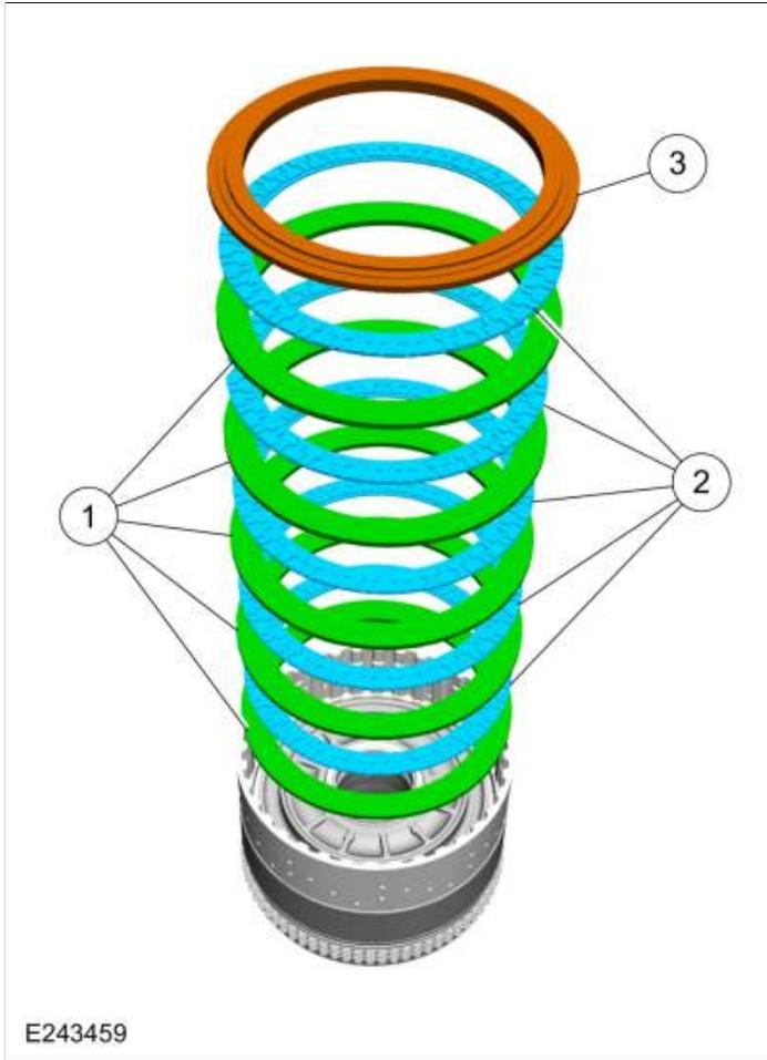
154. Install the C clutch snap ring.
