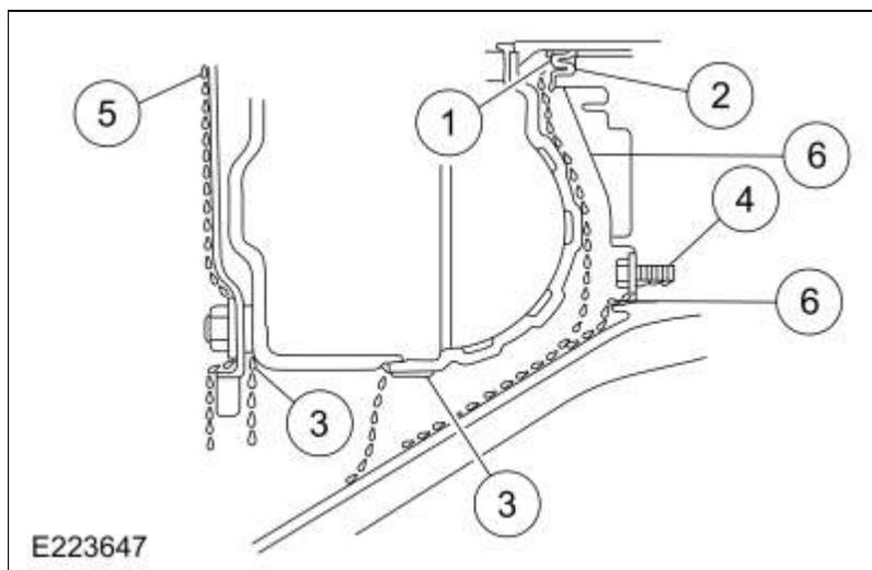
12. Leaks from the torque converter housing can originate from several locations. The paths which the transmission fluid takes to reach the bottom of the torque converter housing is shown in the illustration. The following 6 steps correspond with the numbers in the illustration.
