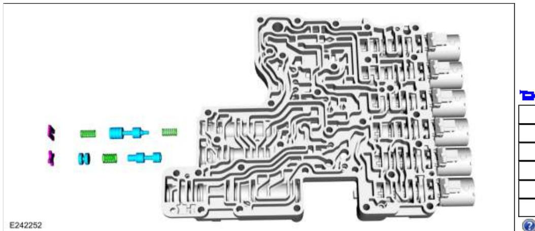
15. **NOTICE:** Solenoids and clutch control valves may visually appear the same but they are calibrated from the factory and are not all the same. Use care not to assemble the main control assembly incorrectly. Incorrect solenoid and clutch control valve installation results in poor transmission shift quality.
