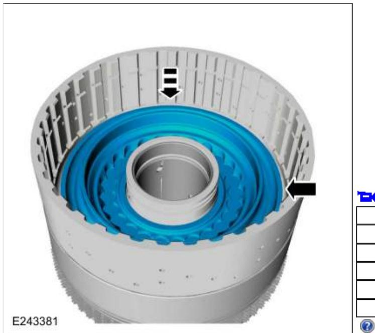
149. Install the new C clutch balance dam seals. Lubricate the seals with petroleum jelly.
