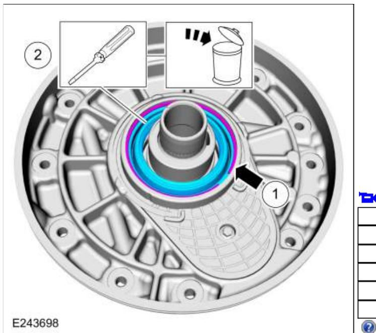
248. Remove the front support cover bolt and the front support cover snap ring.
