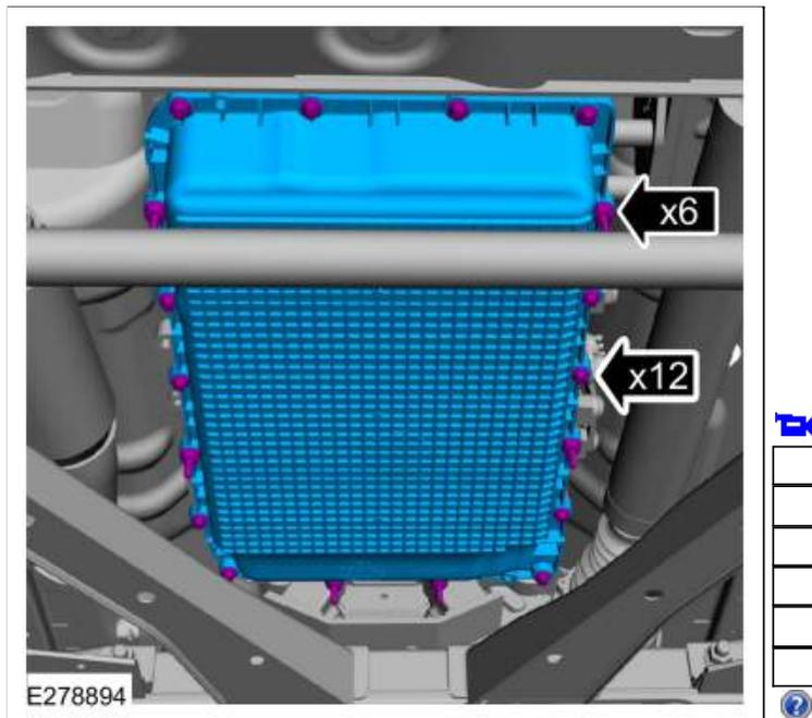
14. **NOTE:** It is not necessary to torque transmission fluid pan bolts at this time.
