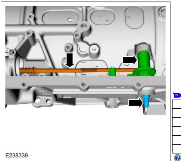
52. Remove and discard the manual control shaft seal.
