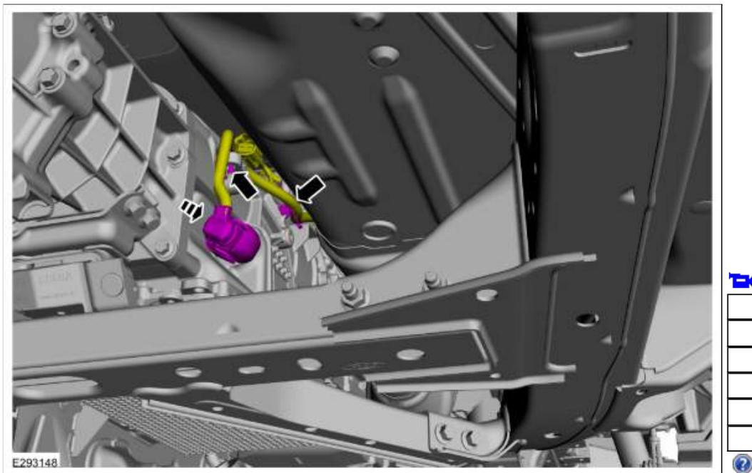
22. If equipped, attach the engine block heater cable.
