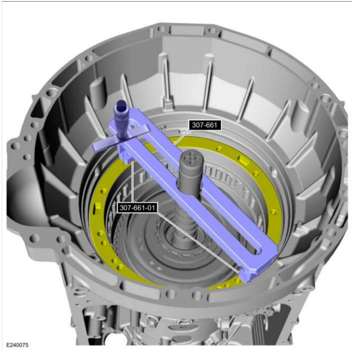
286. Using the special tool and a depth gauge, measure the distance from the top of the special tool to the transmission deck mating surface in 2 different places. Average the measurements. Record this measurement as measurement D. Use Special Service Tool: [307-661 Gauge, End Play](#).
