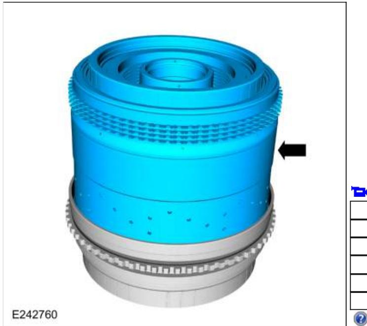
205. Install the No. 3 planetary carrier.
