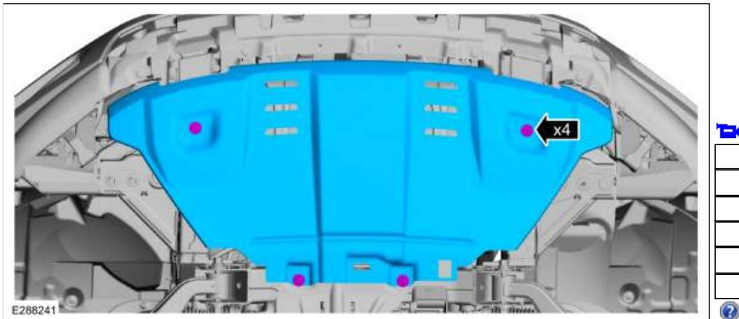
3. Remove the bolts and the rear skid plate.
