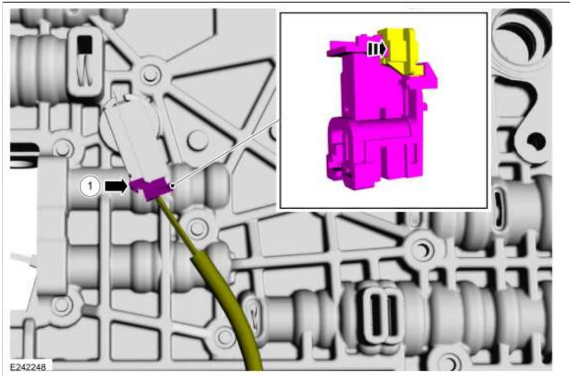
3. Install the main control valve body.
