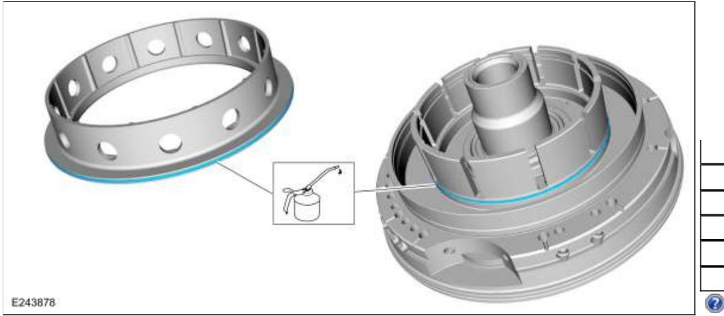
267. Install the A clutch piston by pushing down on the piston until an audible click is heard.
