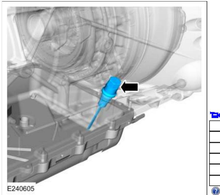
4. **NOTICE:** The vehicle can be driven when the transmission is cold provided the transmission fluid level is between the first hatch mark and 6 on the transmission fluid level indicator. Failure to add transmission fluid to this level can result in damage to the transmission.
