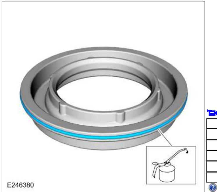
181. Install the E clutch balance dam in the new E clutch piston.
