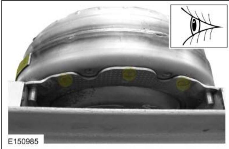
22. After leaks are repaired, clean the remaining transmission fluid dye from serviced areas.
