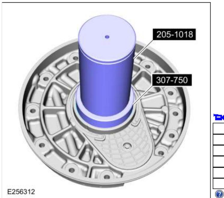
264. Install the torque converter hub seal snap ring.
