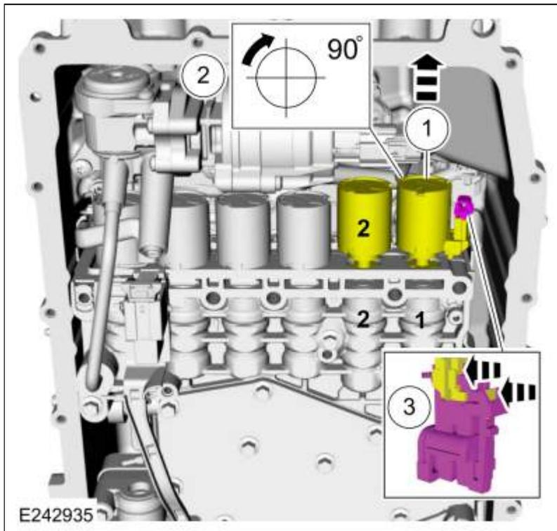
9. Remove the solenoid(s) from the main control valve body.
