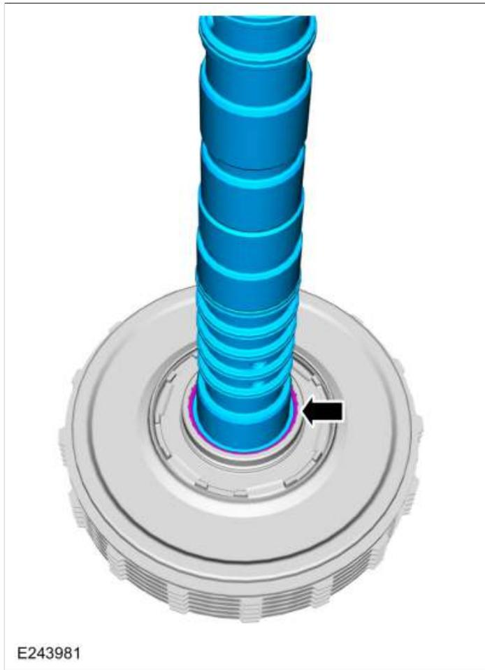
189. Install the (T6) thrust bearing onto the E clutch with the tab locators down. Snap the bearing into place.
