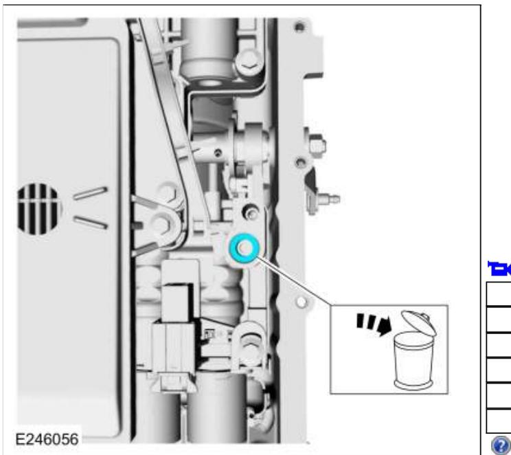
31. Disconnect the transmission fluid auxiliary pump electrical connector.
