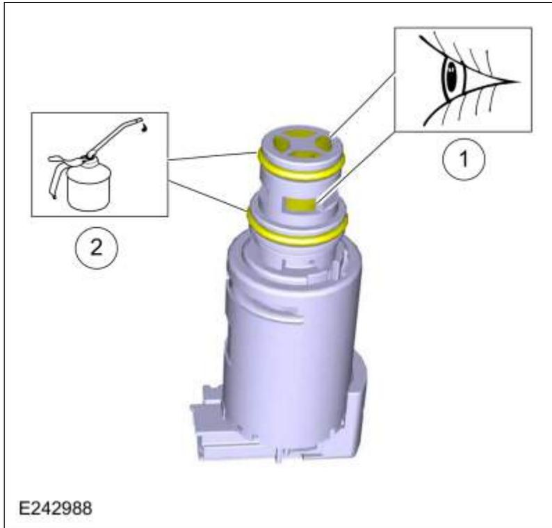
14. Install the solenoid(s) in the main control valve body.
