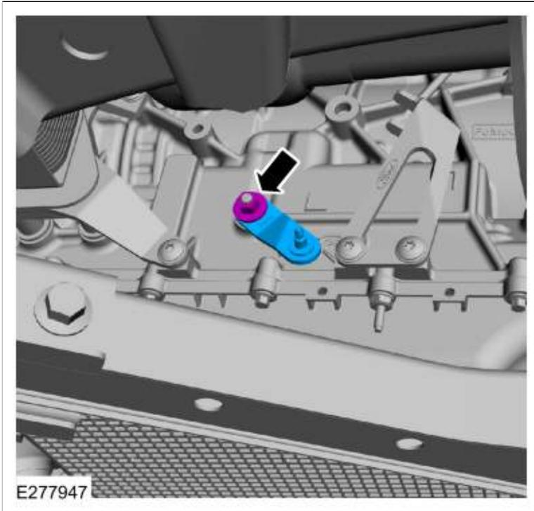
6. Remove and discard the selector shaft seal (7F337).
