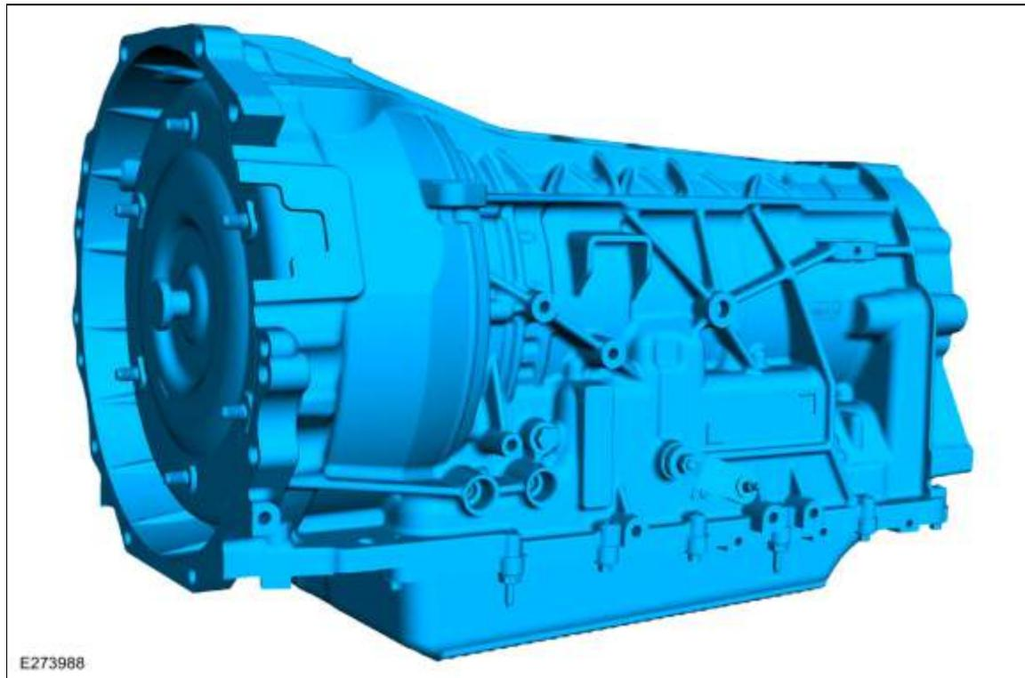
This transmission is a 10-speed electronically controlled transmission which uses planetary gears. Gear selection is achieved by the electronic control of transmission fluid flow to operate various internal clutches.
