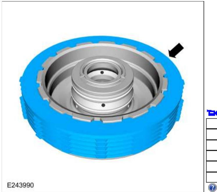
175. Remove and discard the E clutch piston and balance dam inner seals.
