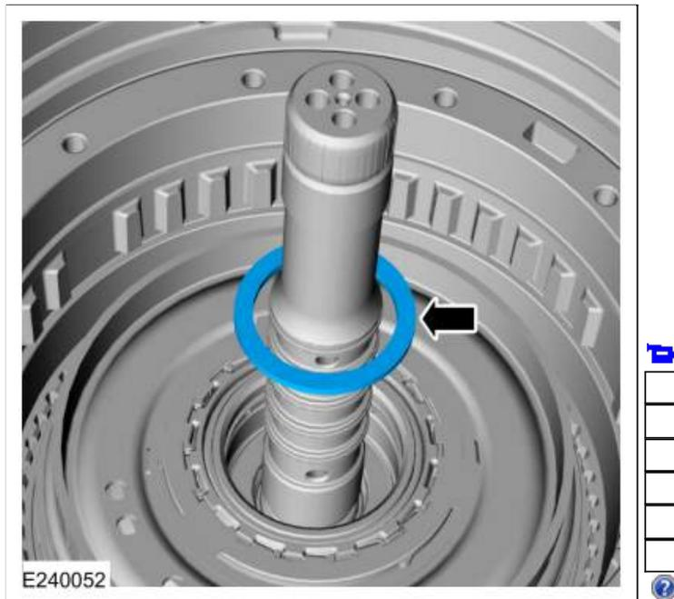
290. **NOTE:** The A clutch separating springs are not installed when measuring the A clutch clearance.
