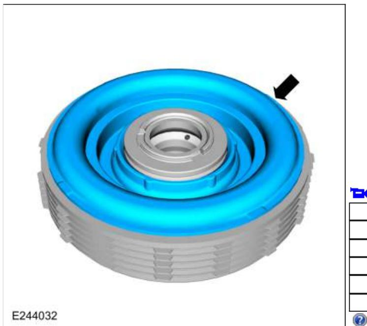
184. **NOTICE: Do not compress the balance dam too far or damage to the E clutch hub can occur. Only compress the E clutch hub far enough to install the retainer.**
