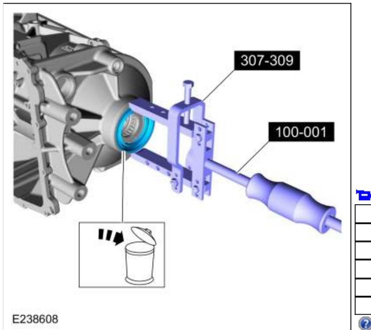
61. If equipped with 2WD, remove the (T11) thrust bearing and the thrust washer.
