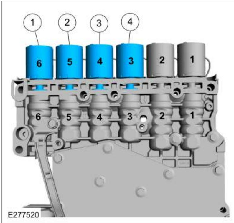
3. Connect the electrical connectors and slide the plastic lock to the locked position.
