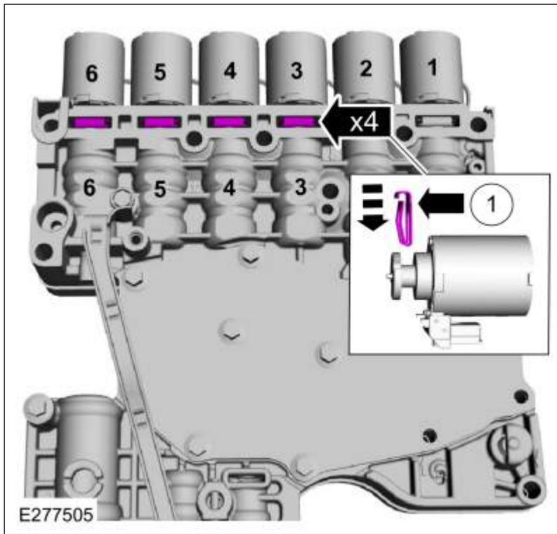
5. Install and the shift solenoid retaining plate and the bolts.
