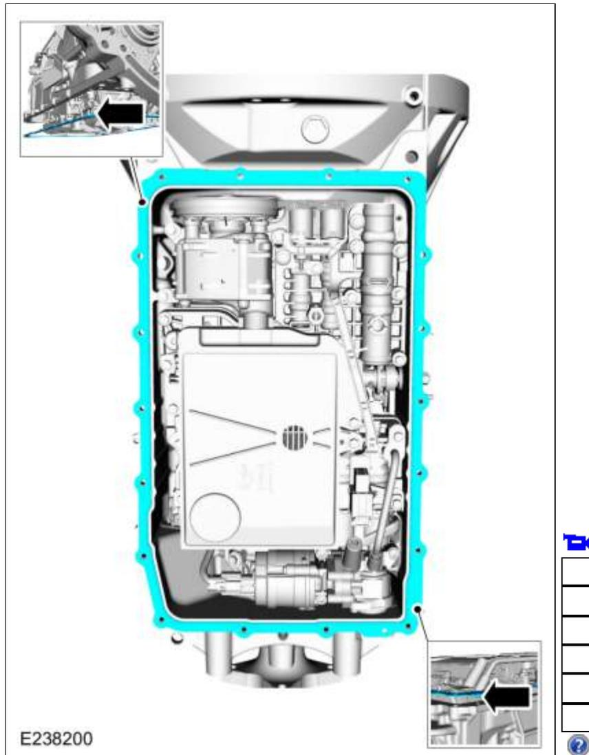
5. **NOTE:** *Install the bolts and studbolts in the correct locations noted during removal.*
