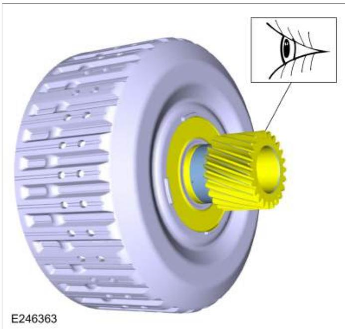
163. Remove the (T7) thrust bearing.
