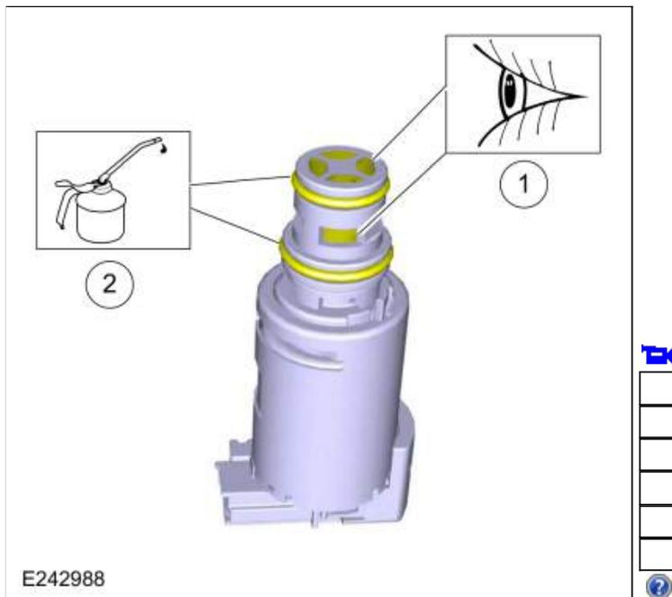
36. Install the TCC solenoid, LPC solenoid, solenoid retaining plate and the new bolts.
