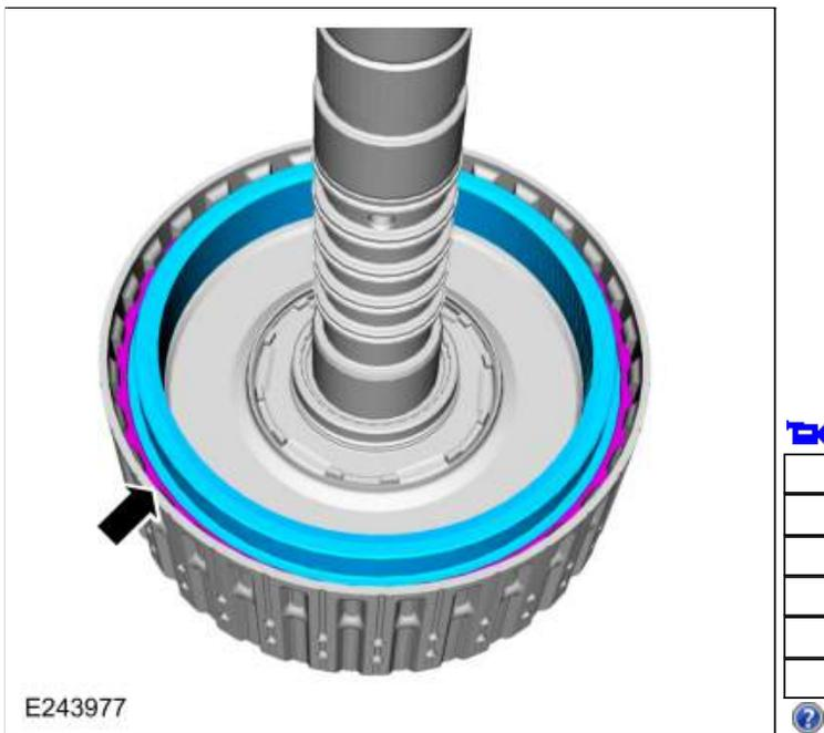
159. Remove the rear No. 3 ring gear snap ring.
