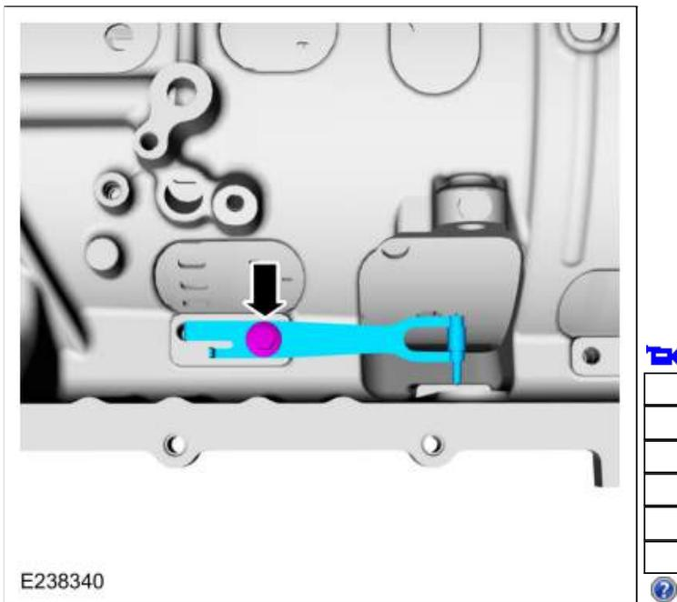
54. Rotate the transmission to a vertical position. Remove and discard the front support assembly bolts.
