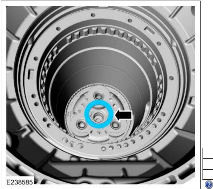
58. Remove the output shaft and planetary carrier No. 4 assembly.
