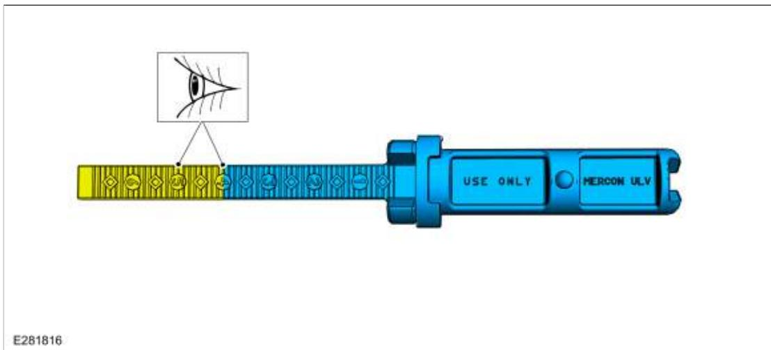
6. If the transmission fluid is not at the correct level, follow the steps for adding or removing transmission fluid.
