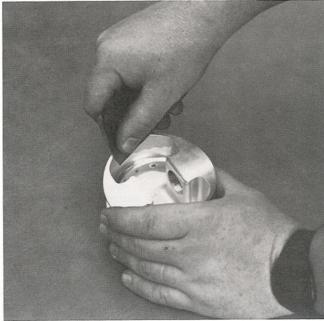
Lightly deburr the piston with 400-grit wet-or-dry sandpaper. Make sure to use a light lubricant like kerosene to help flush the paper while in use.
