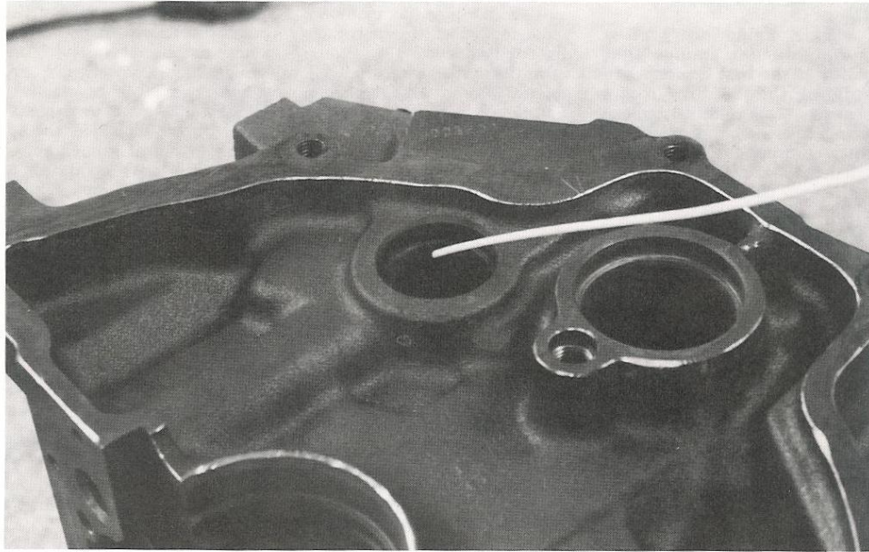
Take great care when removing the rear freeze plug so that the seating lip will not be damaged. Never drive either the freeze plug or the cam core plug into the block to remove.
