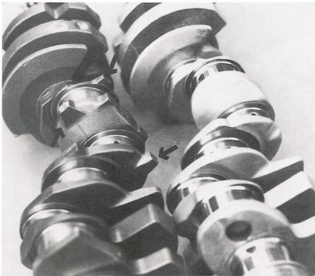
This picture illustrates the rather significant amount of material removal involved in deburring. Notice the absence of the indicated bosses on the finished crank (right).
