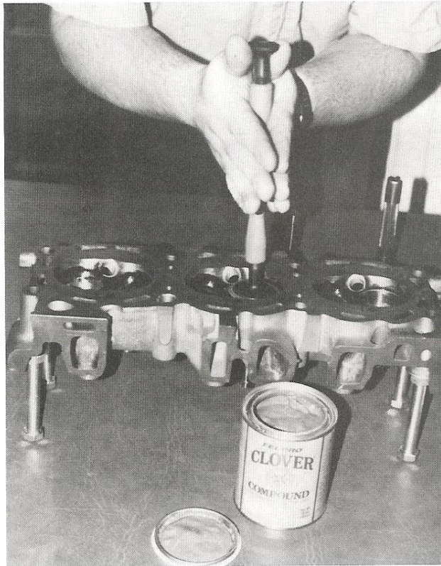
Other than a little arm work, valve lapping requires only two things: a good lapping stick and Clover lapping compound.
