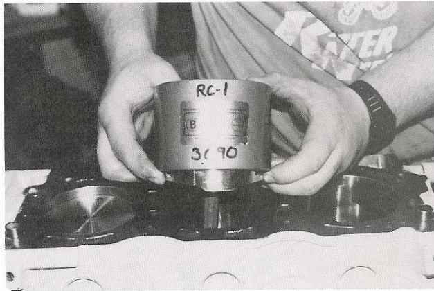
The best way to install the pistons into your engine is to use a tapered ring compressor like the one shown. These
