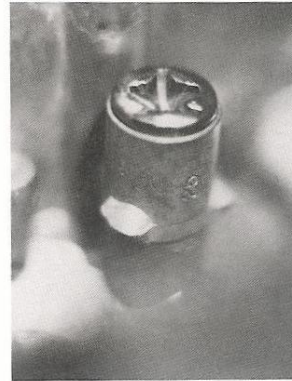
Pump squirters for the 8007 Holley should be a standard configuration type with 0.025in orifices. This squirter can be identified by the #25 stamped on its body.
