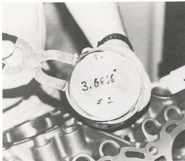
The top and second piston rings should never be installed by hand. Instead, use a piston ring expander
