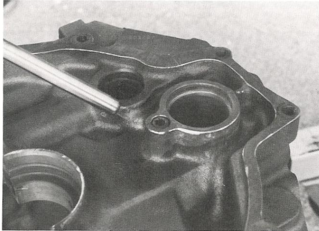
To help remove the rear oil gallery plug, use a propane torch to heat the area around the plug to loosen the factory sealing adhesive.
