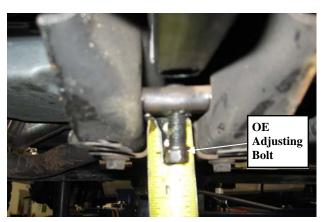
6. Starting on the driver's side, remove the torsion bar adjusting screw. In-
