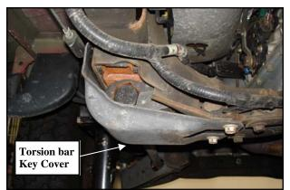
Measure the torsion bar adjusting screw depths and record this dimensions for later use on reassembly. Mark the orientation of the torsion bar in relation to the front A-arm.
