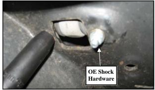
15. With the shocks removed from the vehicle, press the lower mounting studs out.
